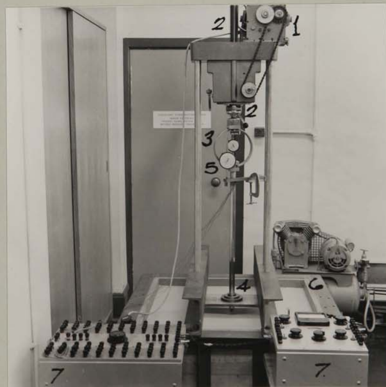
PLATE 2.2. FULL SECTION CONTAINER WITH LOAD CELL IN OPERATION
