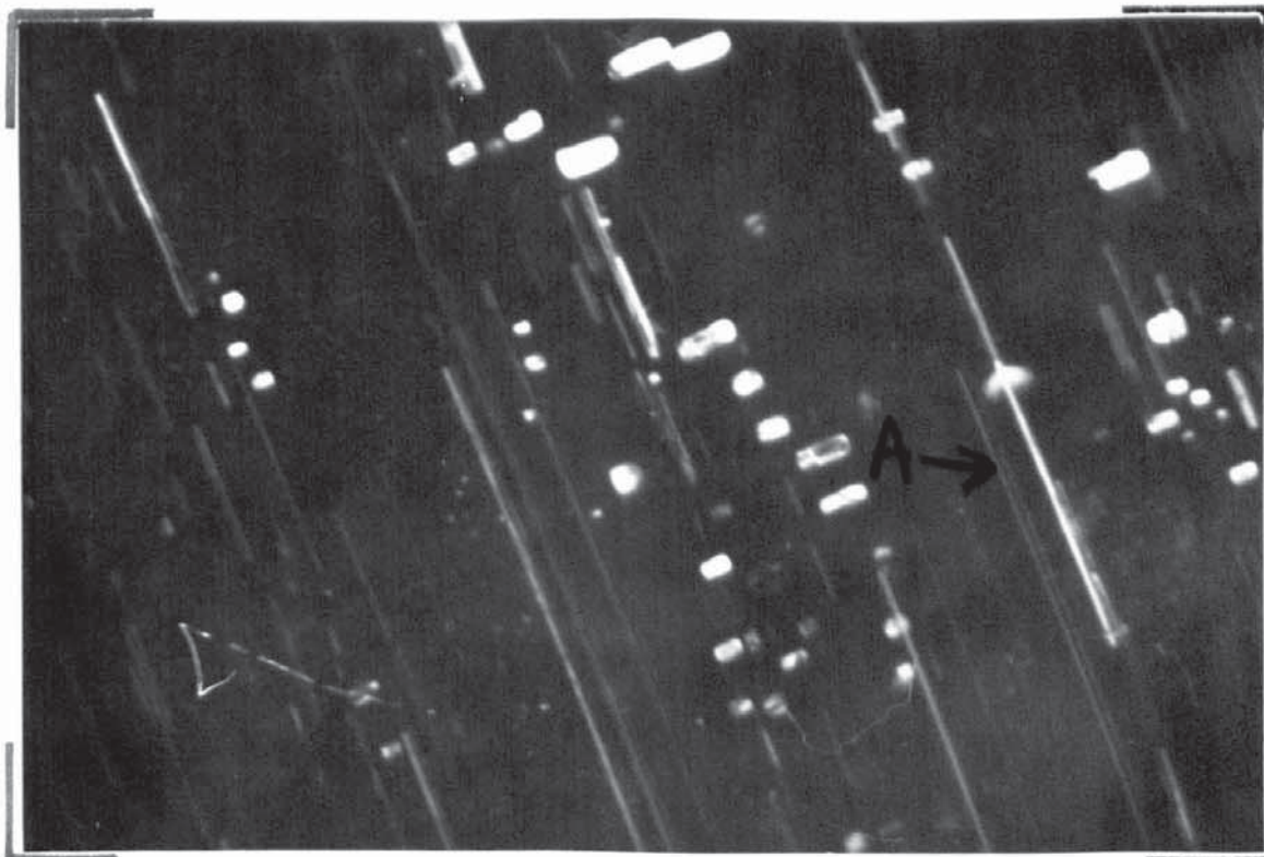
Figure 8.30. Image formed using a precipitate diffracted beam. Diffraction conditions as shown in Fig. 8.28.
