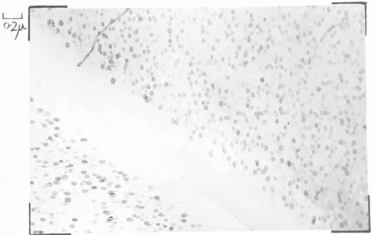
Figure 7.5. Showing a precipitate free zone at a grain boundary.
