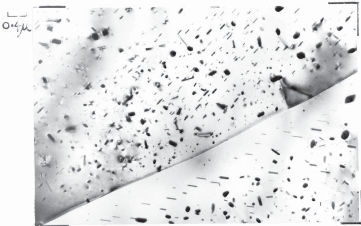
Figure 5.40. As Fig. 5.39 showing an asymmetrical precipitate free zone.
