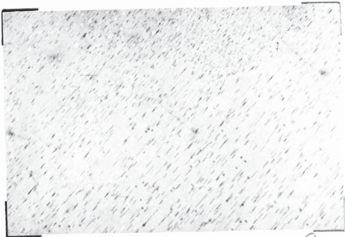
Figure 8.18. Structure after 96 hours at 90°C.. (10\bar{1}0) Mg foil orientation.
