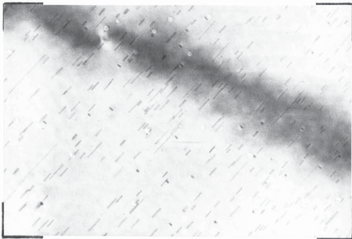
Figure 5.14. Z6 aged for 96 hours at 90°C..
