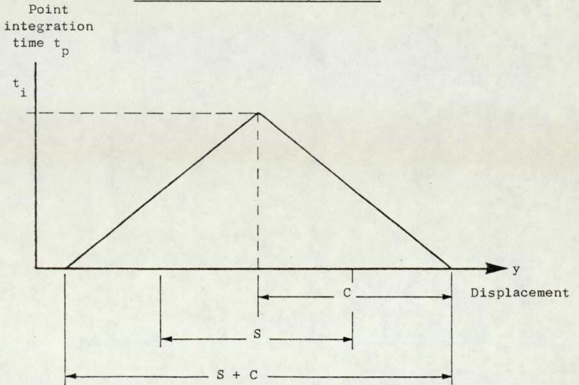
Figure 5.18c. The Sensitivity over a Scanned Strip
