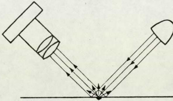
(a) The specular reflection from the bright surface is detected
