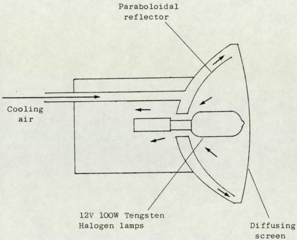
Figure 6.6: Through the Lens Illumination
