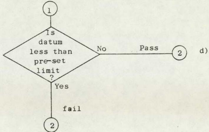
Figure 6.15.e. Flow Chart for Defect Detection Strategy 4
