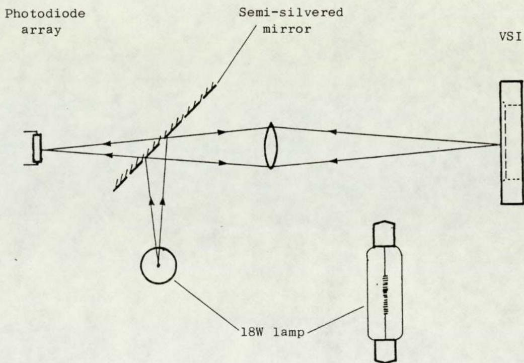
iance with a small 18w lamp which was experimentally useful though inadequate practically in this application. The image of the lamp was focussed onto the component surface. The lamp must have a sufficiently long filament to illuminate the whole of the projected array. If focus is sharp, the image of the filament can be seen in the video signal. The optimum reflectance of the  $45^{\circ}$  semi-silvered mirror is 50 per cent, assuming no losses.
