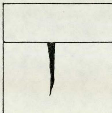
c) Excess penetrant removed
