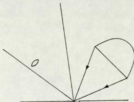
With the small source, the lens does not collect light from surface irregularities which therefore appear dark.
