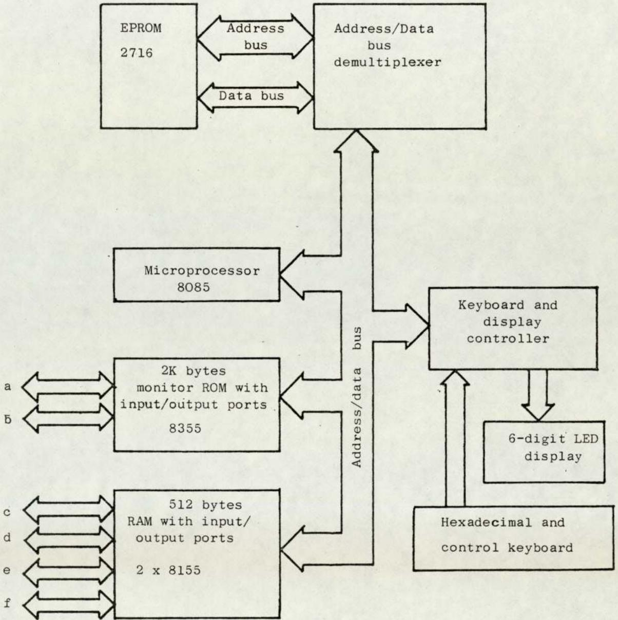
Figure 6.14. Inputs and Outputs to and from the Microcomputer
