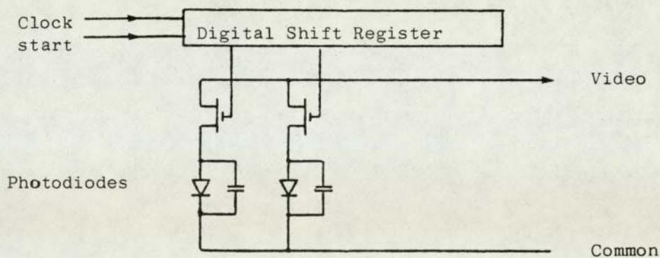
Figure 5.3. Simplified Longitudinal Section of a Linear CCD
