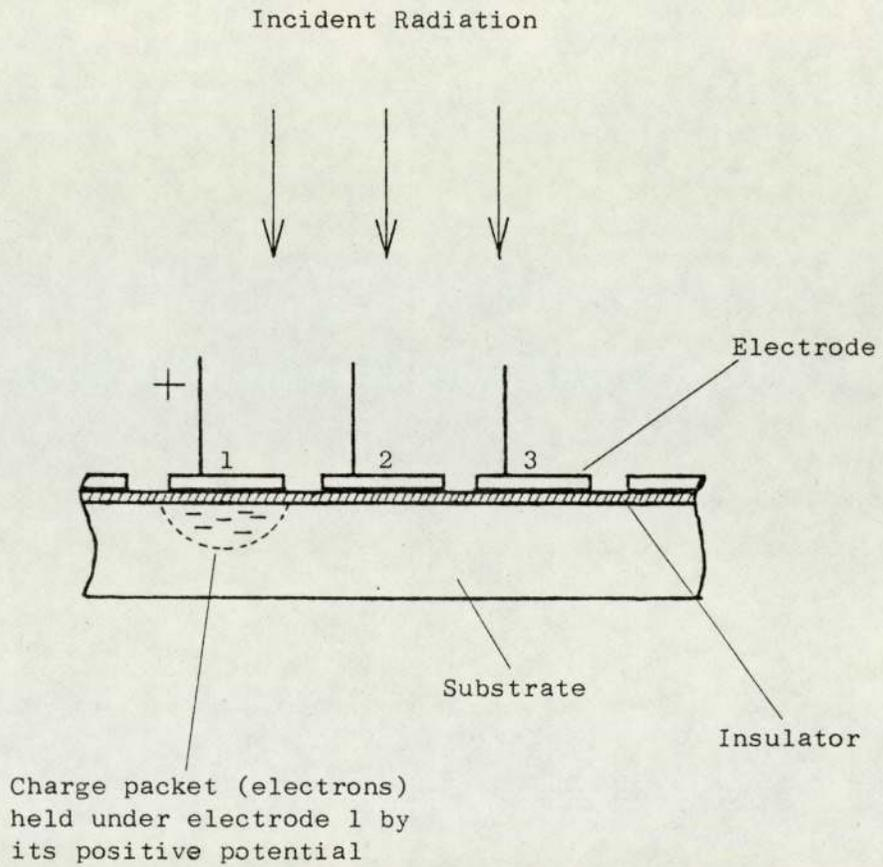
5. c) iii) Mechanism of shifting charge packets
