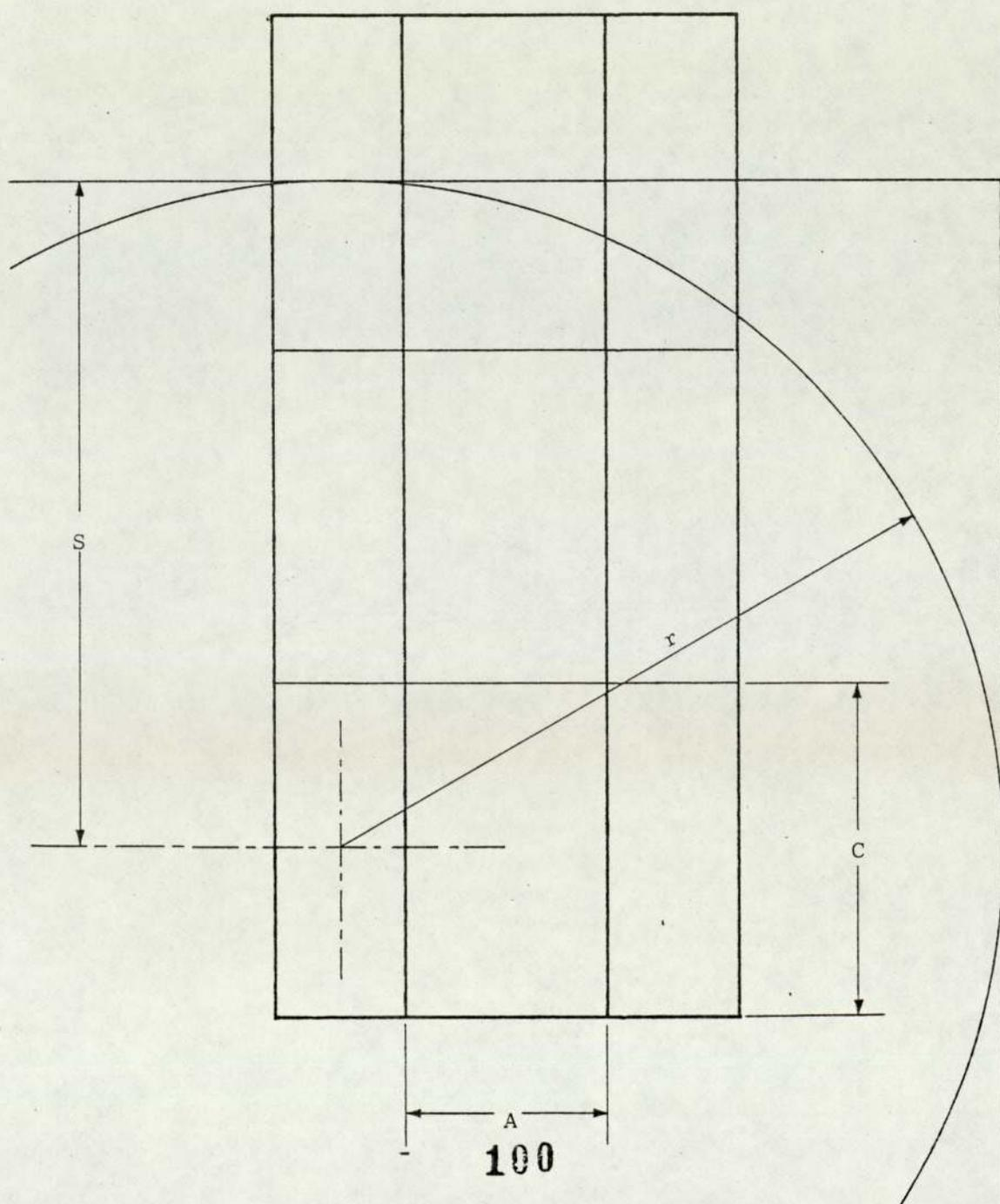
Figure 5.25. The Sensitivity of a Scanned Strip
