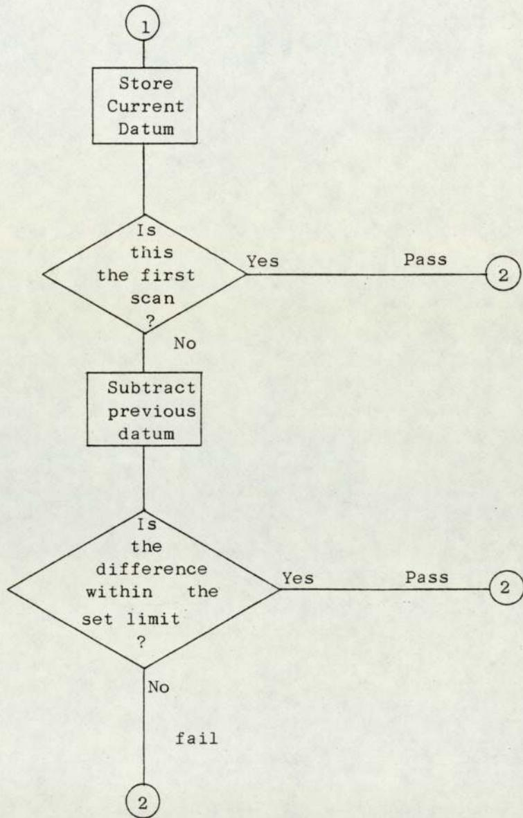
Figure 6.15.f. Flow Chart for Defect Detection Strategy 5
