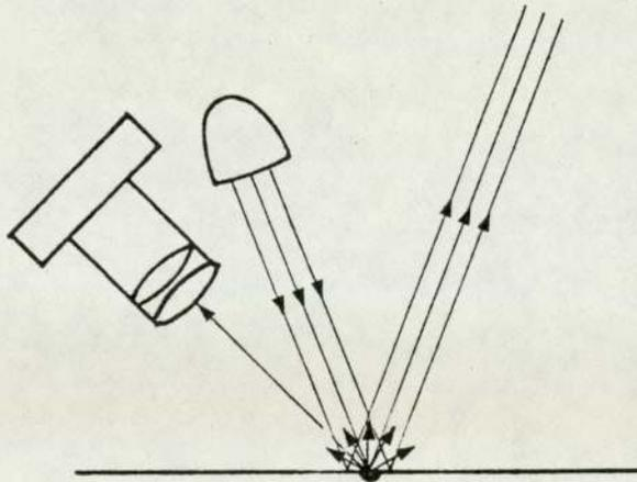
(b) The scattered light from a non-reflective defect is detected.
