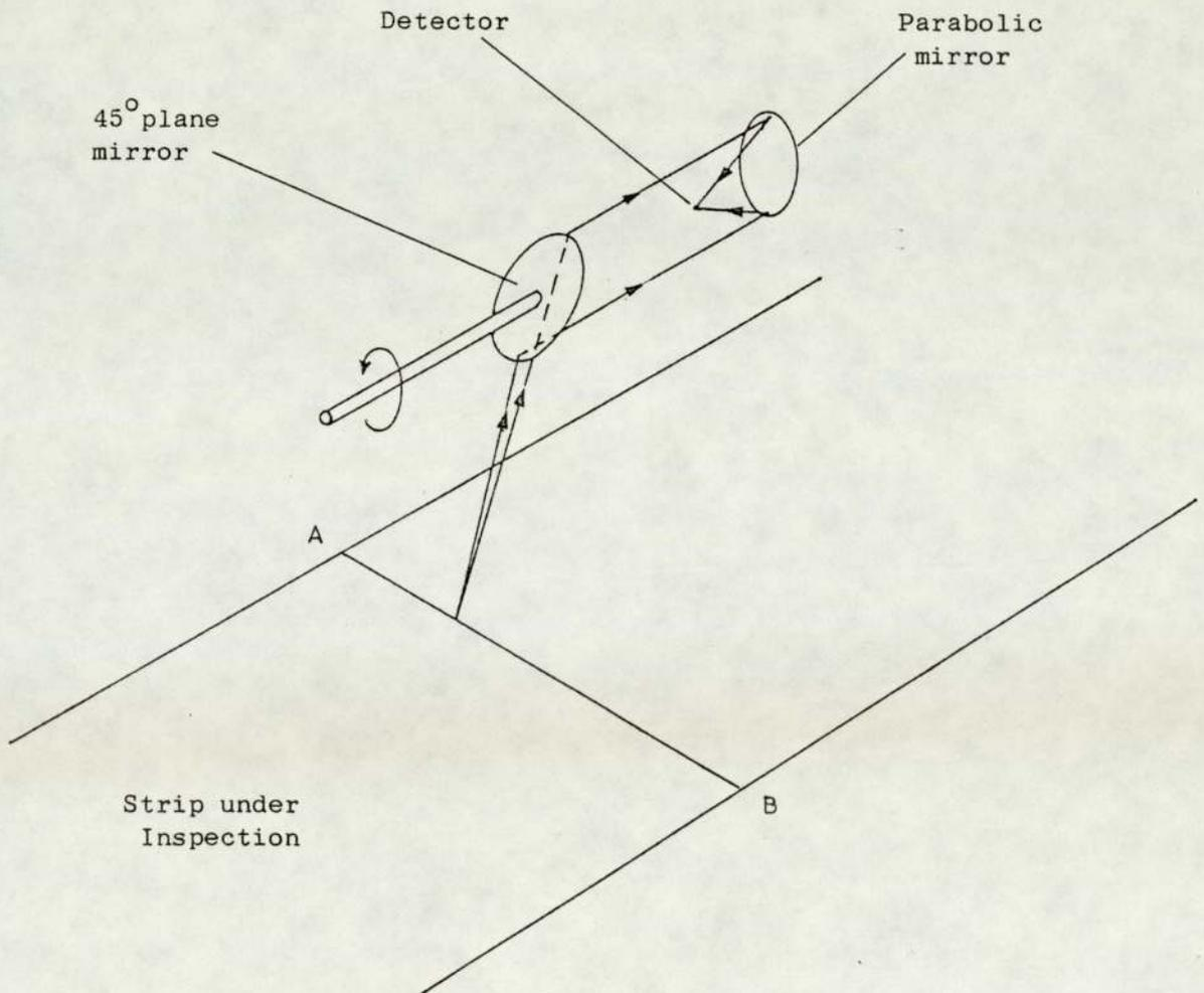
Figure 4.3. Flying Spot Scanner : as developed by the Sira Institute
