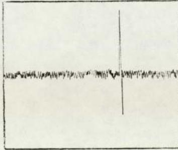
Noise and defect signal (.015") at valve seat centre
