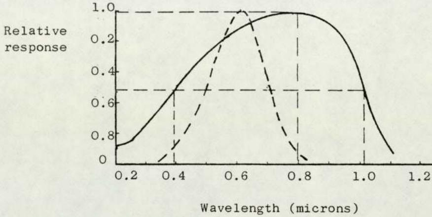
Figure 5.5. Responsivity of One Photodiode in the Array
