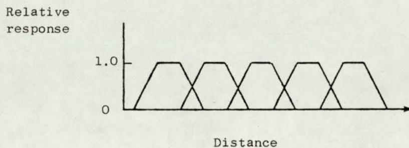
Figure 5.7. A Projection of Array Elements onto a Surface
