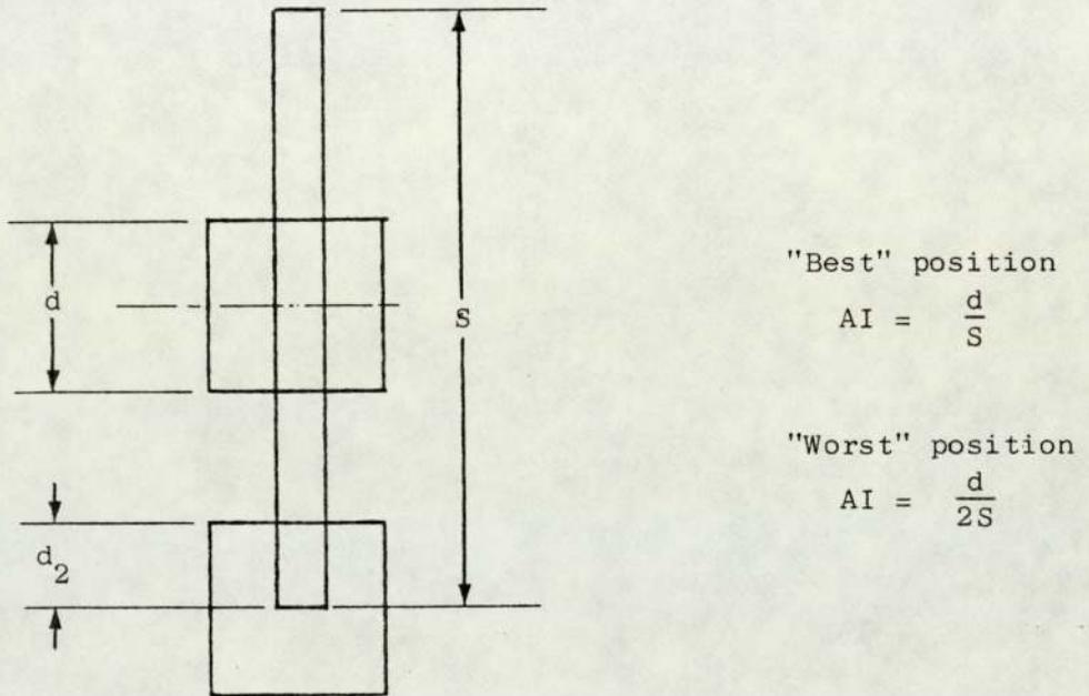
Figure 5.17. AI/Defect Size, for the case shown in Figure 5.16.
