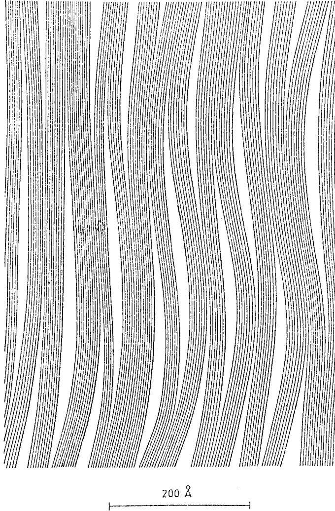
Fig. 3.2 Schematic representation of the ribbon type structure of high modulus carbon fibres.
