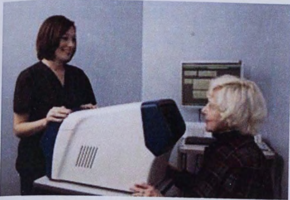
Figure A2.4: Macuscope. The MacuScope uses the psychophysical technique of heterochromatic flicker photometry to measure MPOD.
