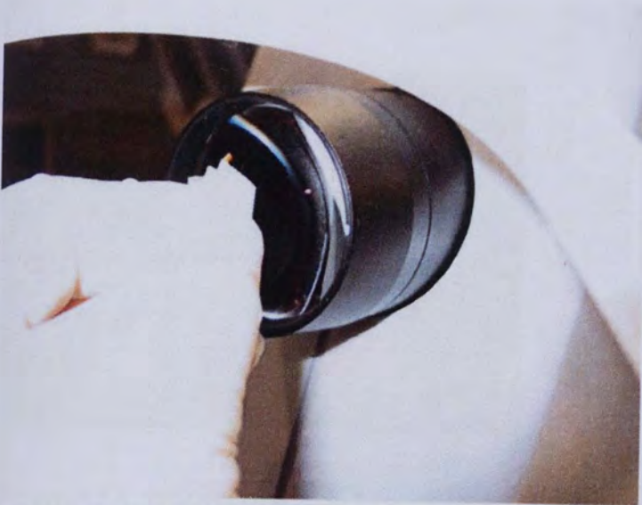
Figure A2.2 Cleaning by circular movements
