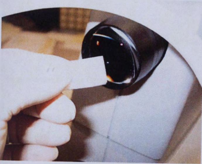
Figure A2.1 Preparing for cleaning with the folded cleaning cloth
