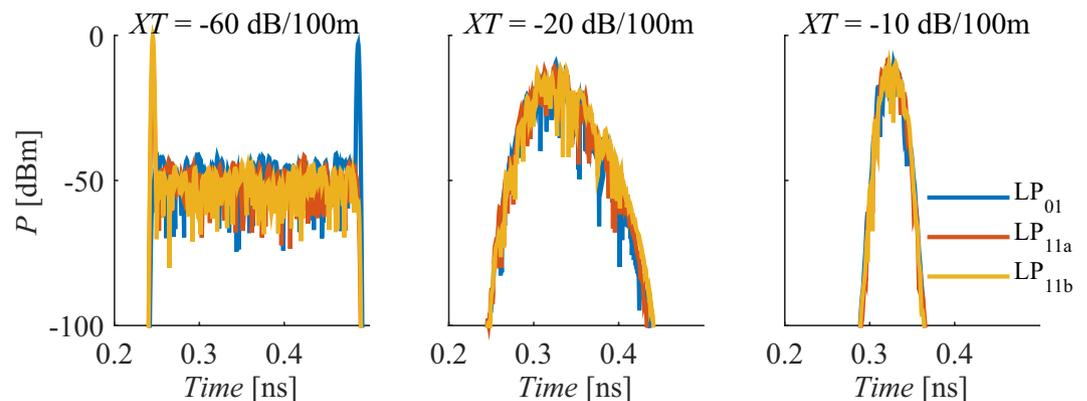
**Figure 2.** Channel impulse response of a 50 km long three-mode fibre with a DMD of 5 ps/km, given the simultaneous launch of three Gaussian pulses (2.5 ps FWHM), one per mode, with XT equal to: (a)  $-60$  dB/100 m, (b)  $-20$  dB/100 m, and (c)  $-10$  dB/100 m.
