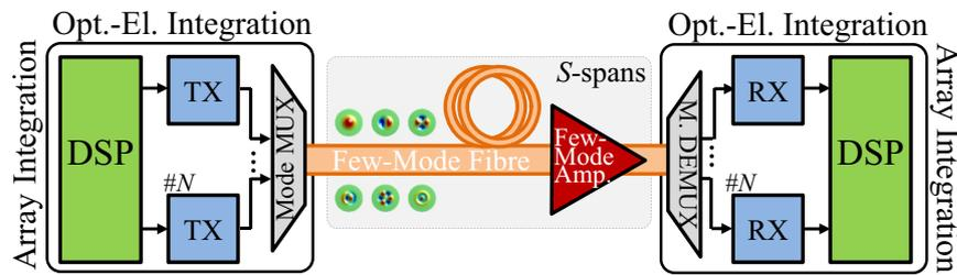
**Figure 1.** Basic system concept for a multi-span MDM system. MDM offers the possibility of high-density integration of the optical-electronic components and of efficient exploitation of shared DSP to simultaneously mitigate FMF specific impairments and array-specific impairments.
