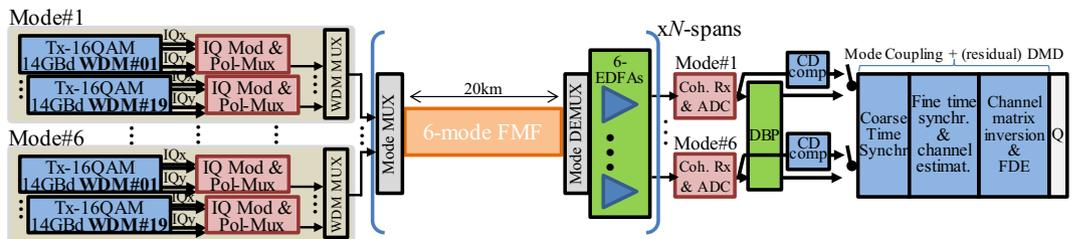
**Figure 5.** Simulation setup for 6 LP modes each with 2 orthogonal polarisations, 19 WDM channels, including: optical transmitter, mode multiplexer (MUX) and demultiplexer (DEMUX), FMF, coherent receiver, and DSP blocks.
