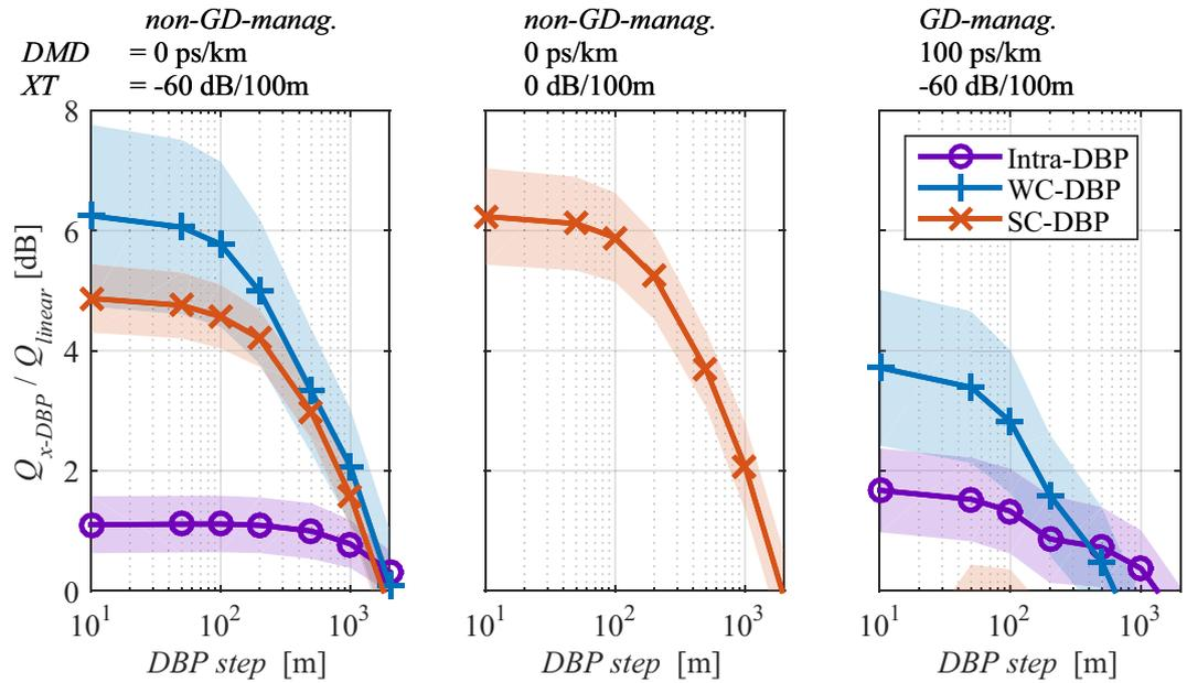
**Figure 6.**  $Q$ -factor gain over linear equaliser for WC- and SC-DBP as a function of the DBP step after 240 km for 0 dBm/ch and for different combinations of  $XT$ ,  $DMD$  and  $GD$  management segments. Lines shadow accounts for 3 times the standard deviation for 40 repetitions.
