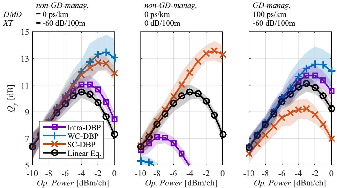
**Figure 7.**  $Q$ -factor as a function of the power per channel after 240 km for different combinations of  $XT$ ,  $DMD$  and  $GD$  management segments. Lines shadow accounts for 3 times the standard deviation for 40 repetitions.
