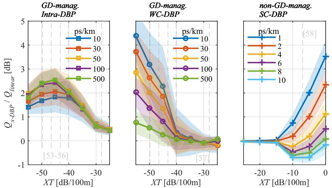
**Figure 8.** *Q*-factor gain over linear equaliser as a function of *XT* after 240 km, 0 dBm/ch and different *DMD* values, with: (a) Intra-DBP, (b) WC-DBP and (c) SC-DBP. Lines shadow accounts for 3 times the standard deviation for 100 repetitions.
