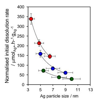
**Figure 5.** Ag<sup>+</sup> dissolution rates normalized to mass of Ag determined by XANES for Ag/SBA-15, Ag/TiO<sub>2</sub>/SBA-15 and Ag/TiO<sub>2</sub>/MM-SBA-15.
