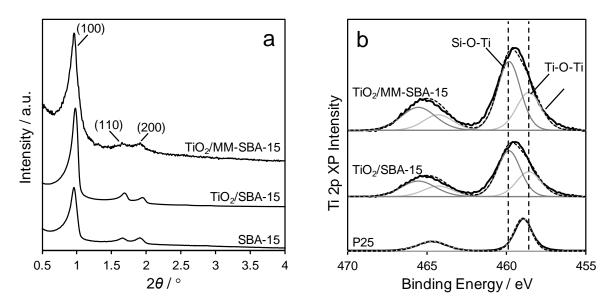
**Figure 3.** (a) Low angle X-ray diffraction (XRD), and (b) fitted Ti 2p XP spectra of TiO<sub>2</sub>/SBA-15 and TiO<sub>2</sub>/MM-SBA-15, alongside pure silica (SBA-15) and titania (P25) references.
