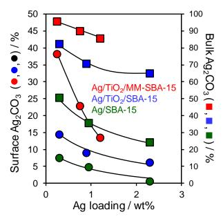
**Figure 4.** Surface (XPS) and bulk (XANES) silver speciation as  $Ag_2CO_3$  of Ag/SBA-15,  $Ag/TiO_2/SBA-15$ , and  $Ag/TiO_2/MM-SBA-15$  as a function of Ag loading.
