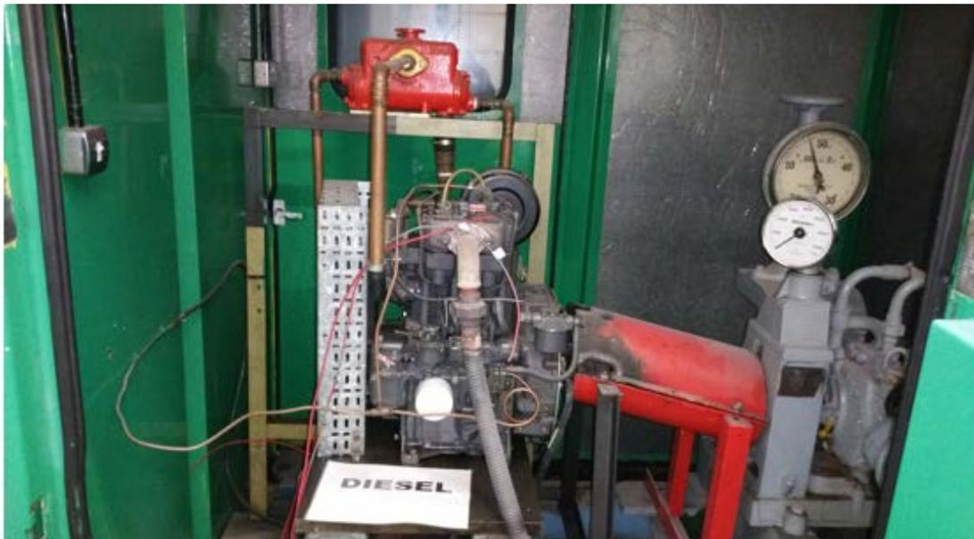
Figure 44: Engine testing platform before modification.
