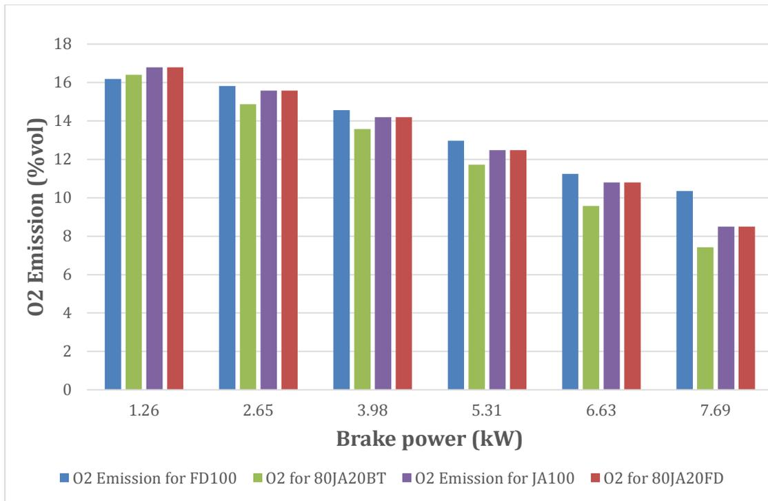
Figure 85: O<sub>2</sub> emission vs. load of FD100, JA100 and its blends.
