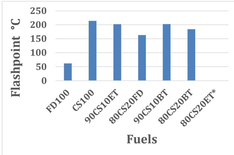
Figure 77: Flashpoint of CS100 and its blends.
