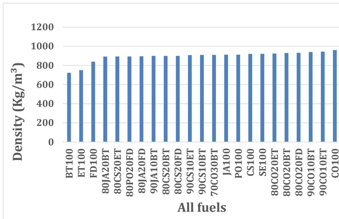
Figure 70: Density of all fuels – ASTM 1298.
