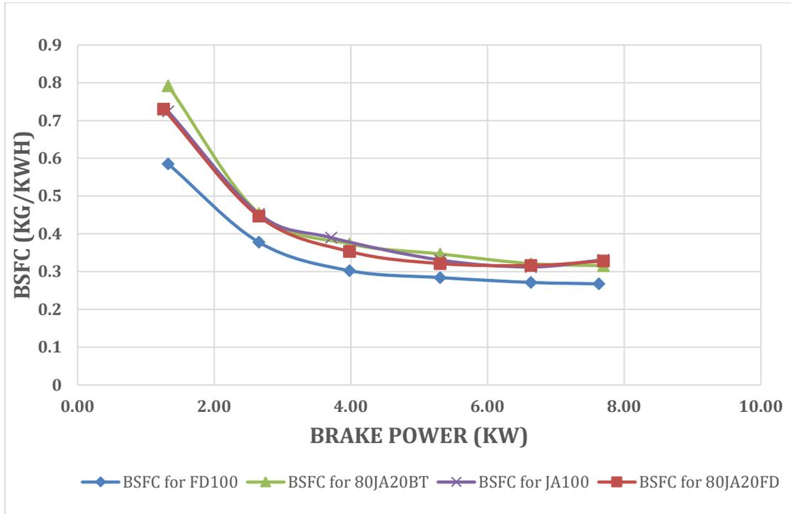
Figure 80: Brake Specific Fuel Consumption vs. load of FD100, JA100, and its blends.
