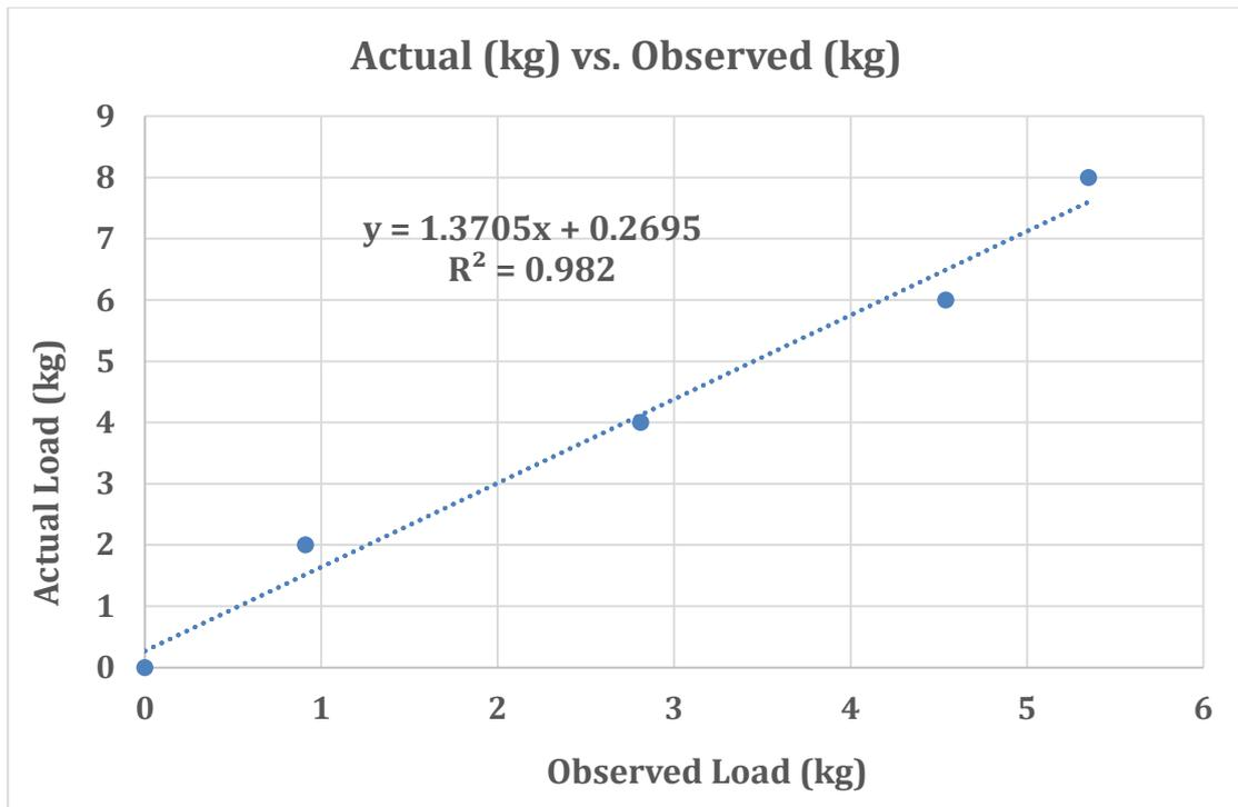
Figure 45: Froude Dynamometer Calibration.
