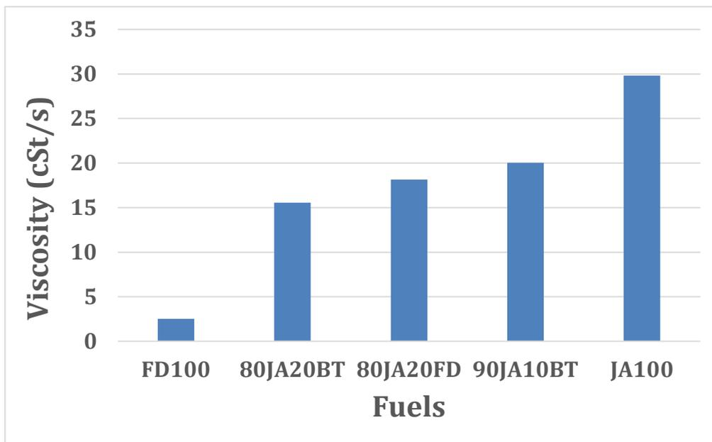
Figure 69: Viscosity of FD100 with JA100 and its blends at 40 °C.
