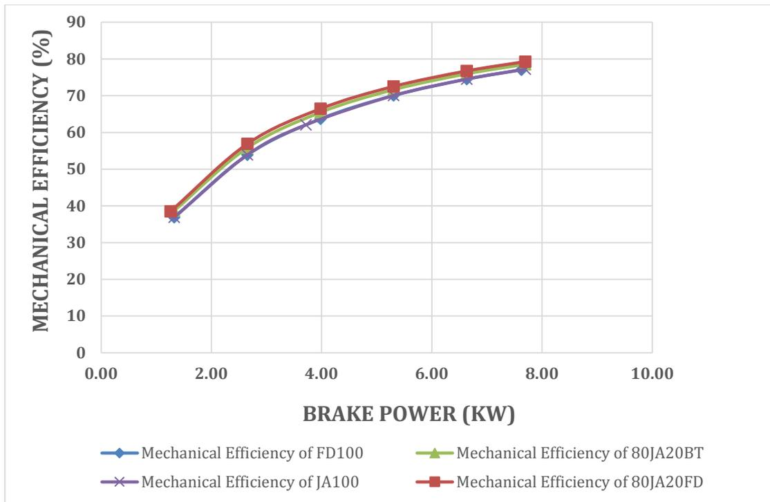
Figure 82: Mechanical Efficiency vs. load of FD100, JA100 and its blends.
