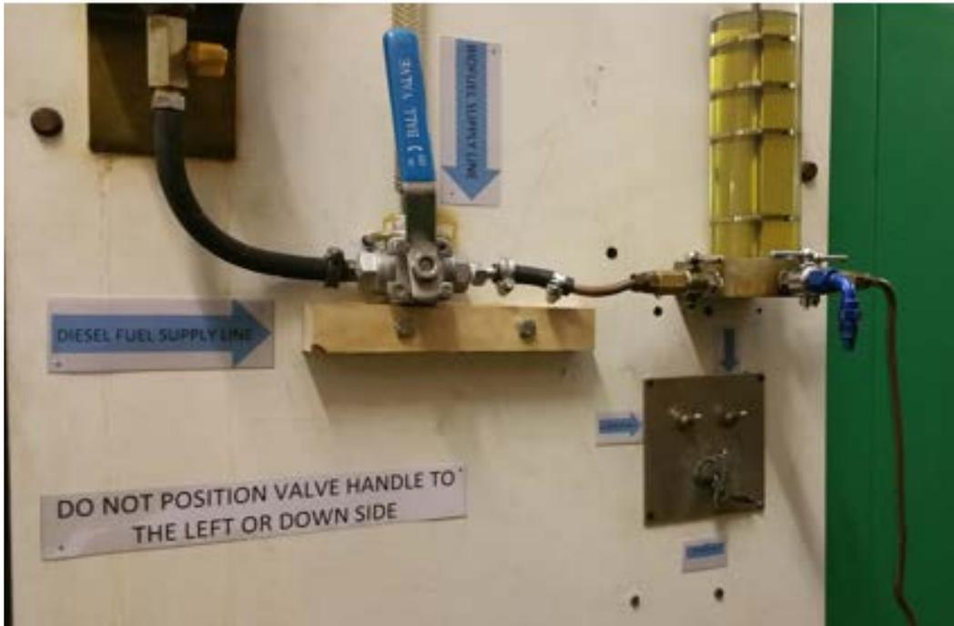
Figure 50: Three-way ball valve for fuels is changing.
