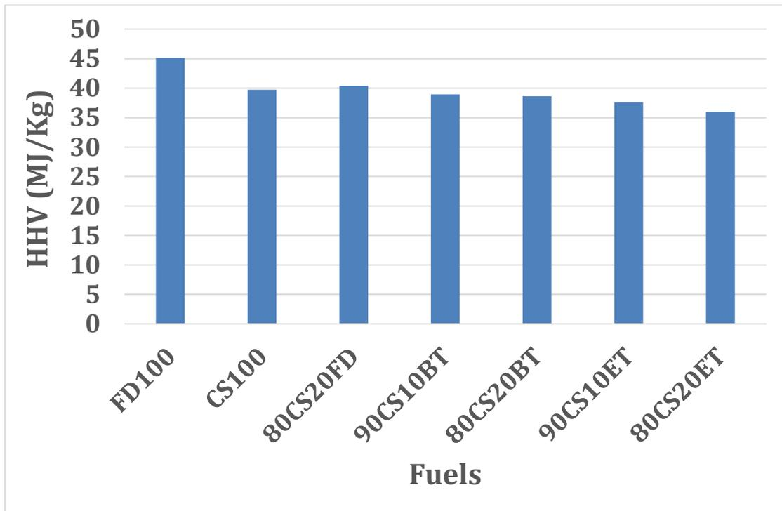
Figure 62: HHV of FD100 with CS100 with its blends.
