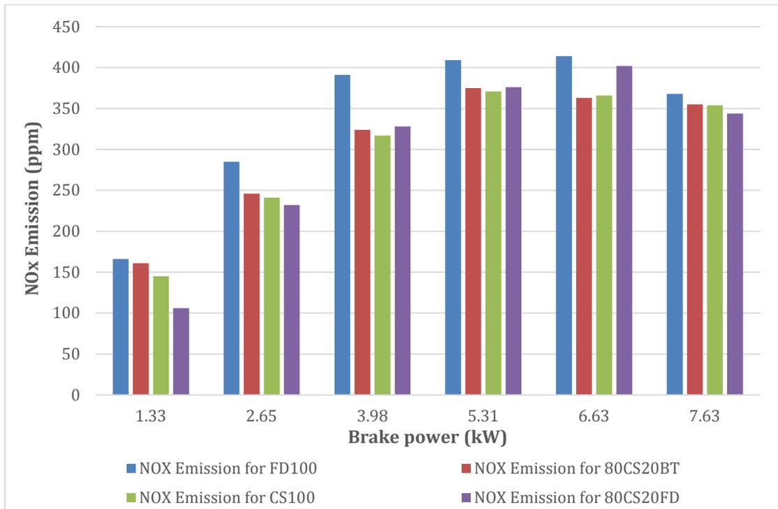
Figure 101: NO<sub>x</sub> emission vs. load of FD100, CS100 and its blends.
