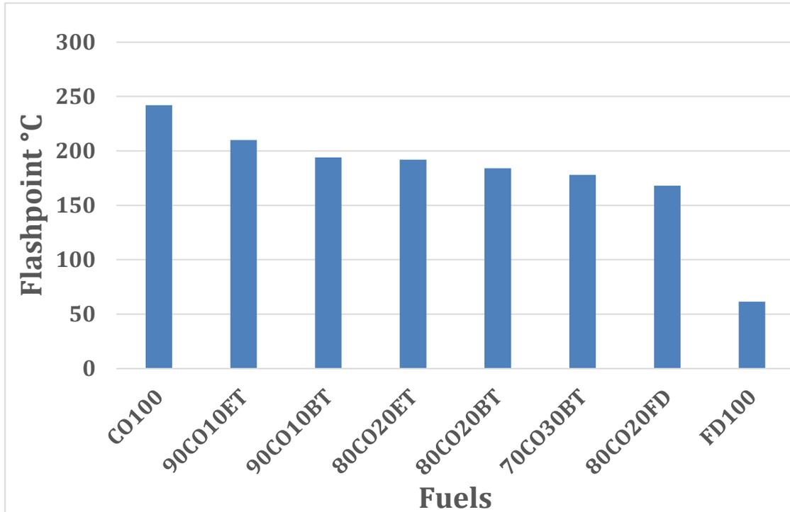
Figure 78: Flashpoint of CO100 and its blends.
