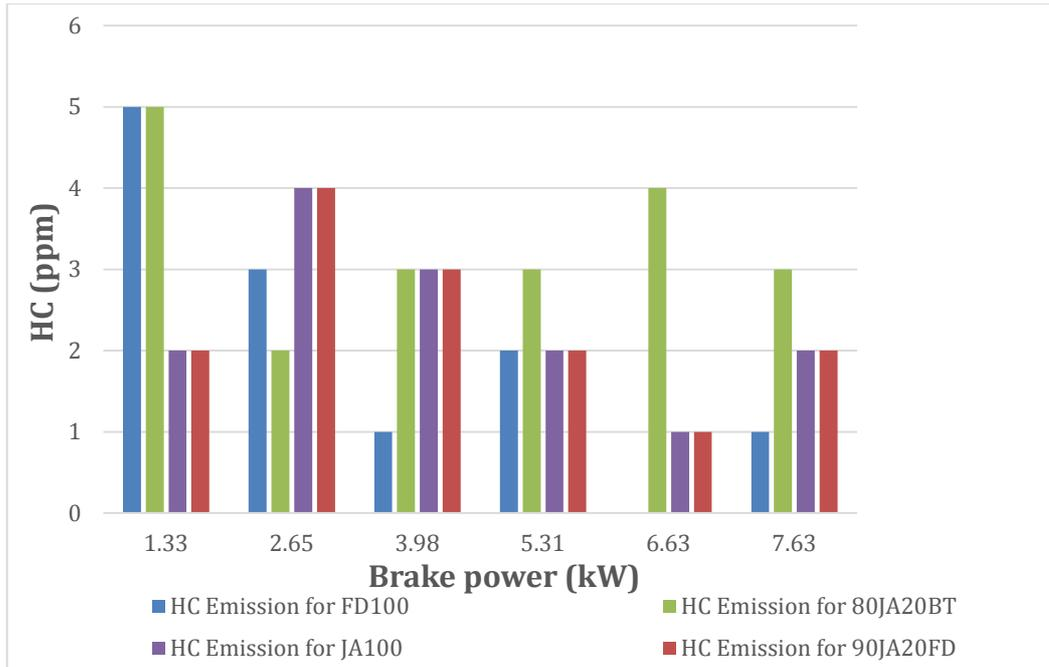
Figure 87: HC emission vs. load of FD100, JA100 and its blends.
