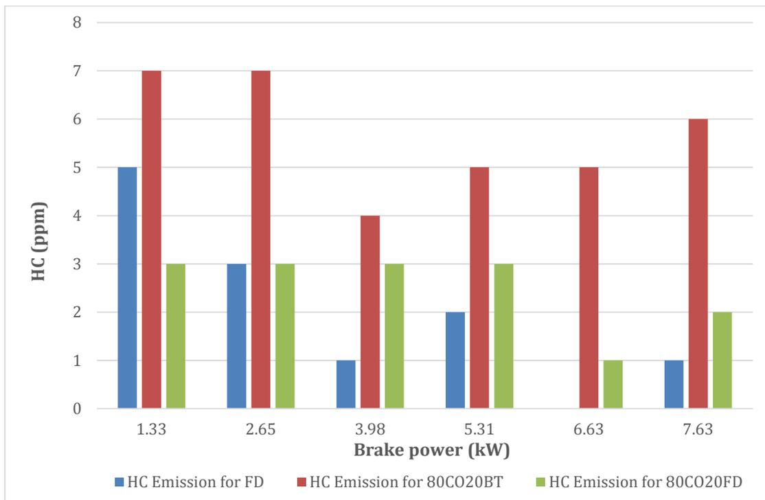
Figure 111: HC emission vs. load of FD100, CO100 and its blends.
