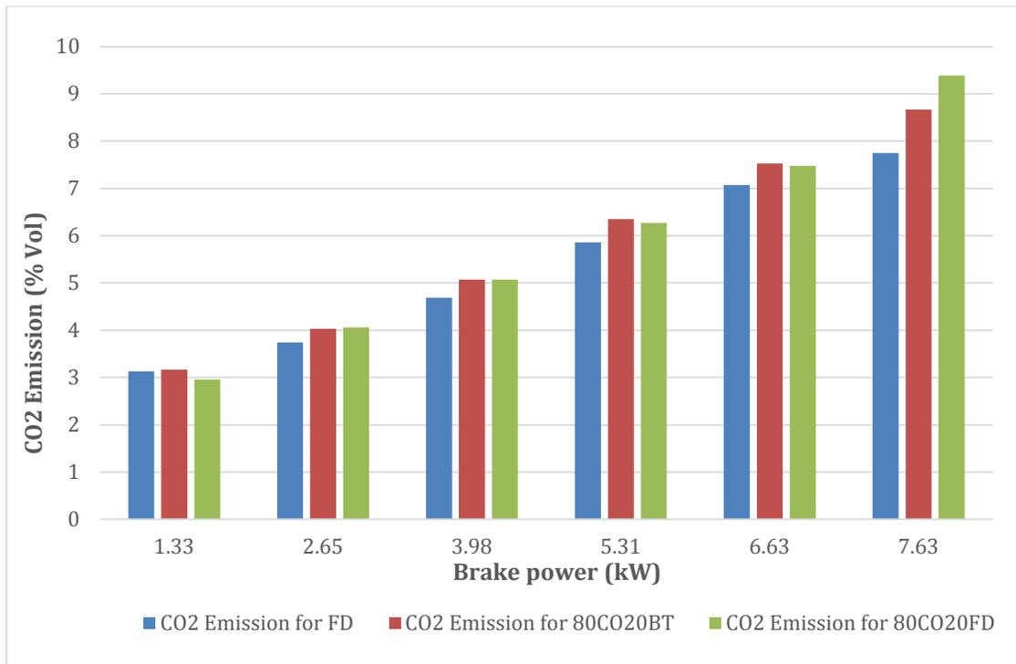
Figure 110: CO2 Emission vs. load of FD100, CO100 and its blends.
