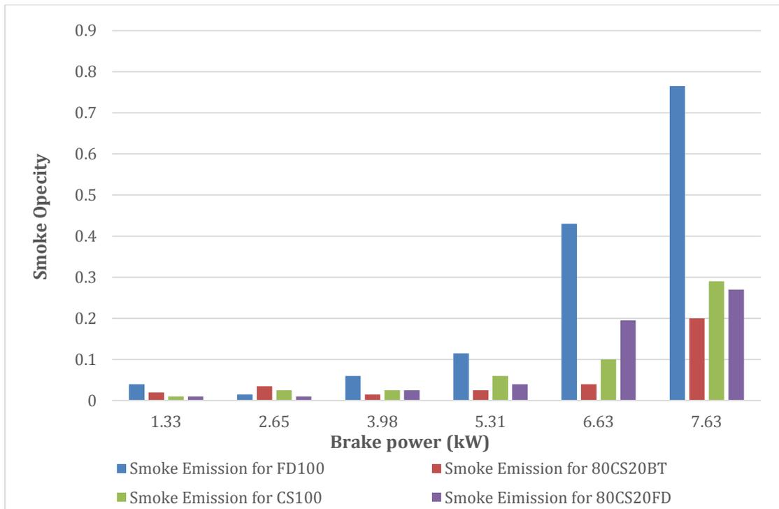
Figure 102: Smoke emission vs. load of FD100, CS100 and its blends.
