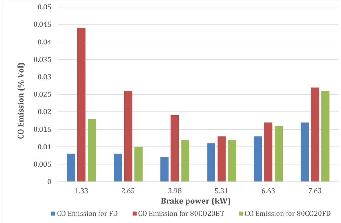
Figure 108: CO emission vs. load of FD100, CO100 and its blends.
