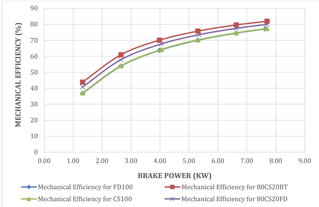
Figure 94: Mechanical Efficiency vs. load of FD100, CS100 and its blends.
