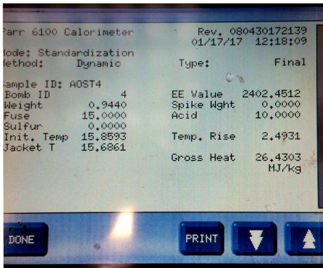
Figure 1: Standardization of Parr 6100 Calorimeter.
