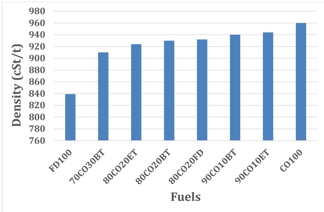
Figure 74: Density of FD100 and CO100 with its blends.
