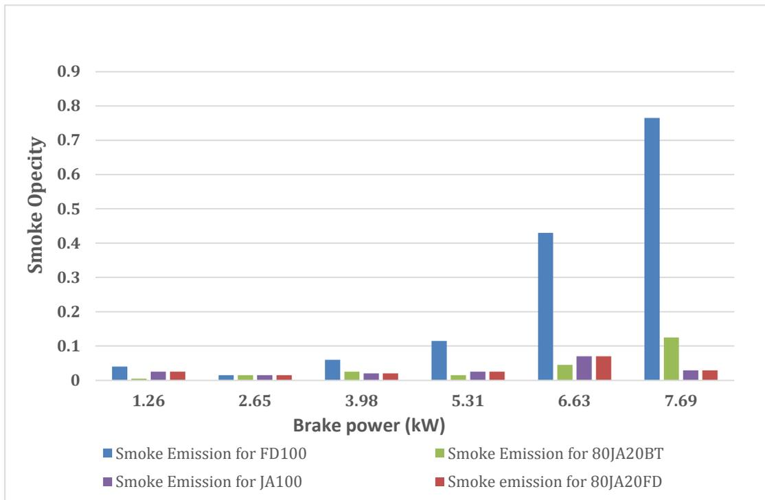
Figure 90: Smoke emission vs. load of FD100, JA100 and its blends.
