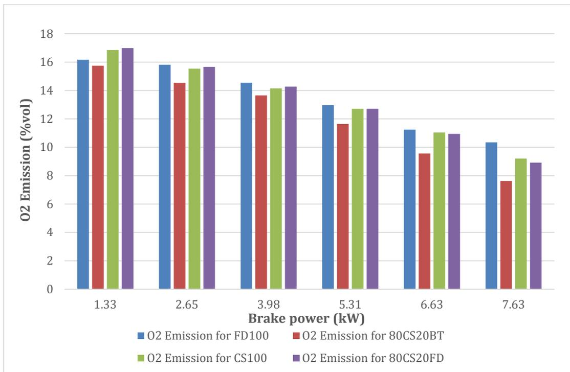
Figure 97: O<sub>2</sub> emission vs. load of FD100, CS100 and its blends.
