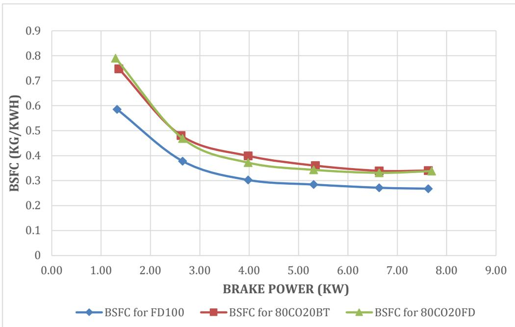
Figure 104: Brake Specific Fuel Consumption vs. load of FD100, CO100, and its blends.
