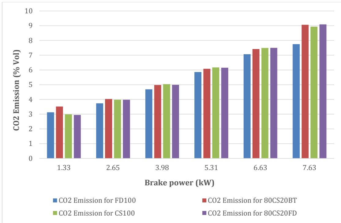
Figure 98: CO<sub>2</sub> Emission vs. load of FD100, CS100 and its blends.
