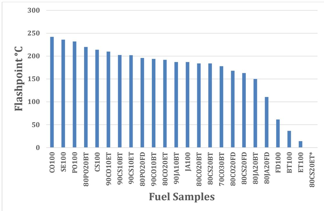
Figure 75: Flashpoint of pure plant oils -ASTM D3278.
