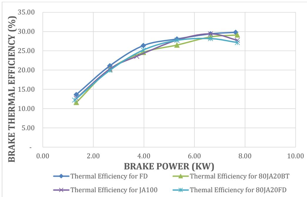
Figure 81: Brake Thermal Efficiency vs. load of JA100 and its blends.
