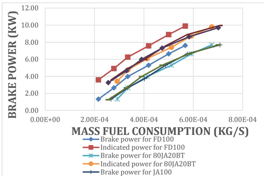
Figure 79: Brake and Indicated powers vs. Mass Fuel consumption of FD100 & JA100 and its blends.
