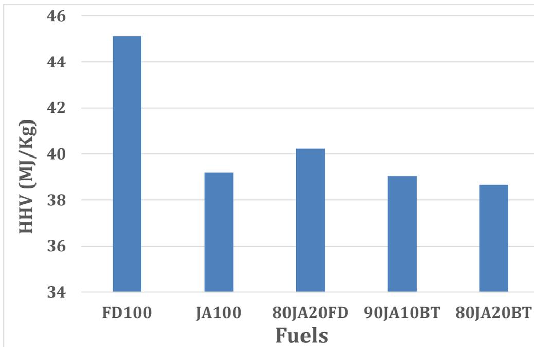
Figure 63: HHV of FD100 with JA100 with its blends.
