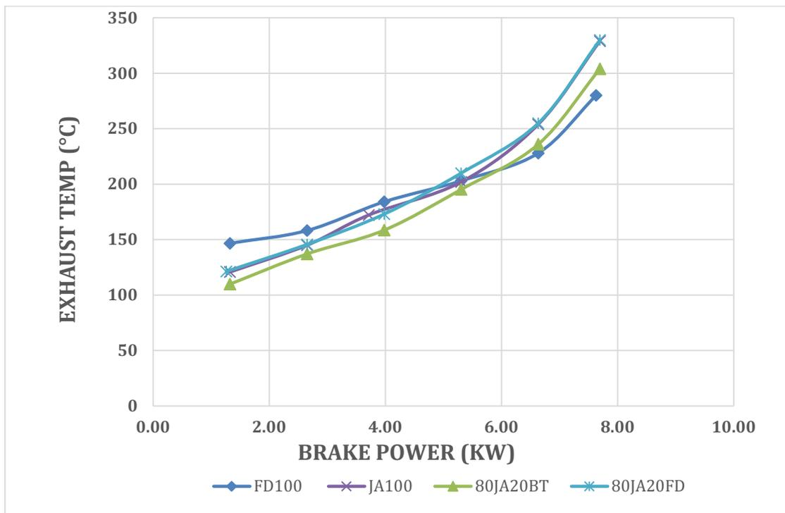
Figure 83: Exhaust temperature vs. load of FD100, JA100 and its blends.
