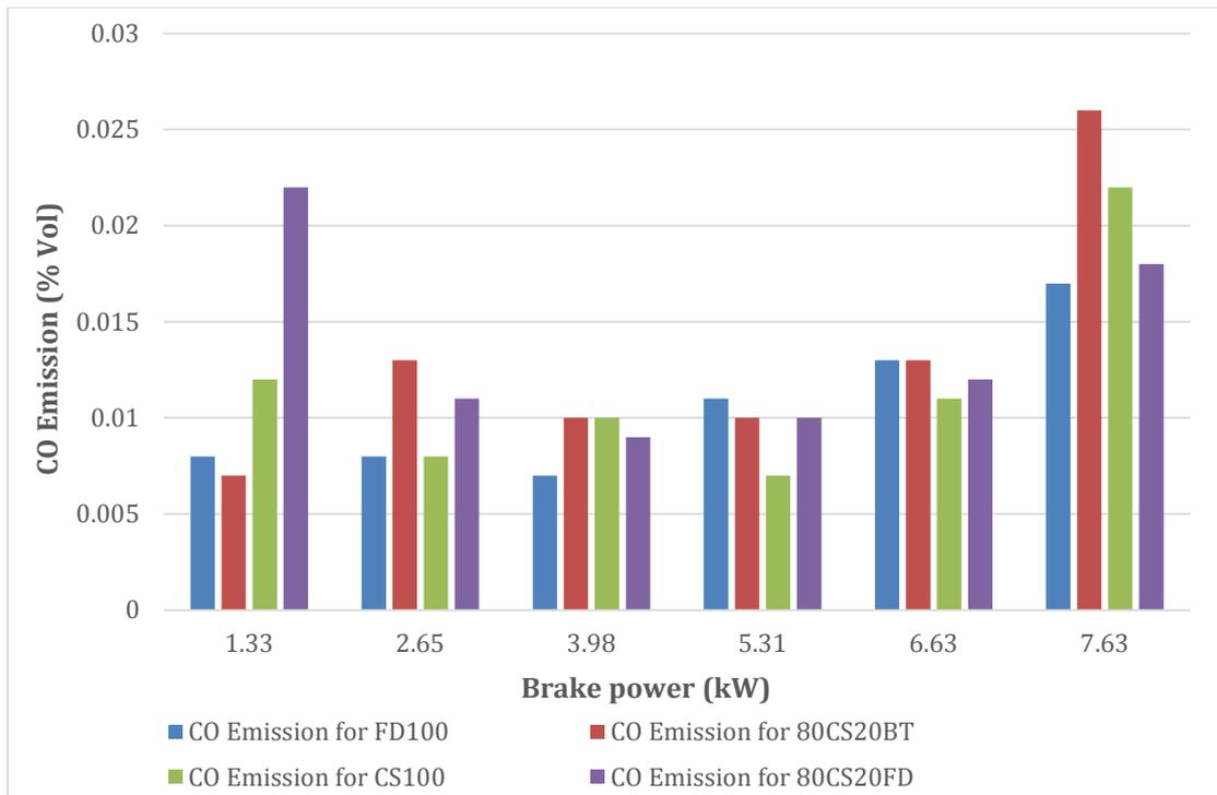
Figure 96: CO emission vs. load of FD100, CS100 and its blends.
