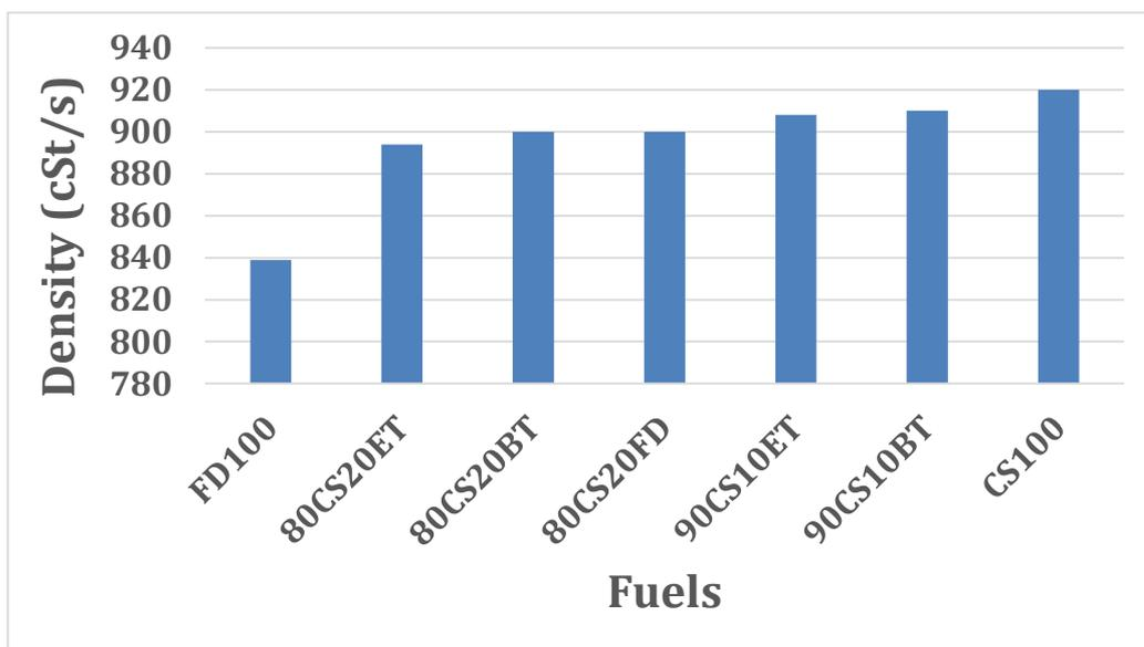
Figure 72: Density of FD100 and CS100 with its blends.
