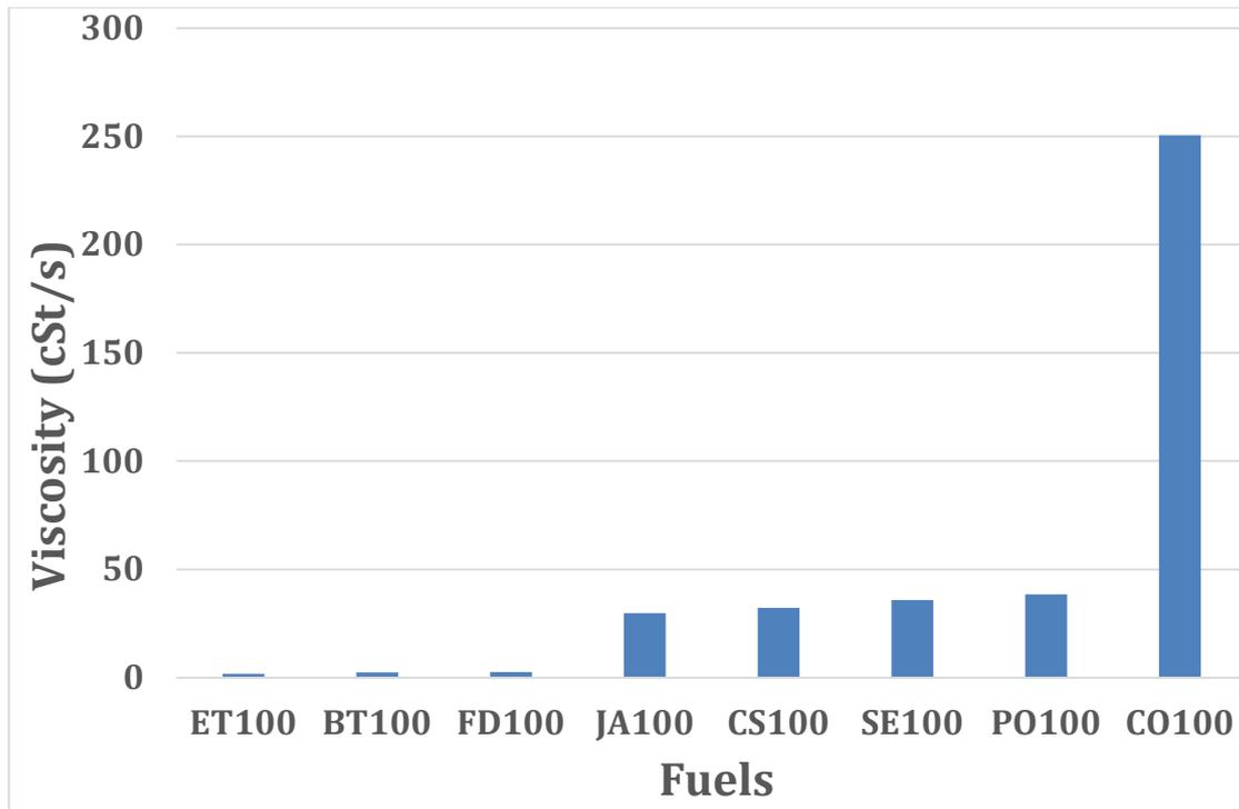
Figure 67: Viscosity of FD100 and other 100% fuels at 40 °C.
