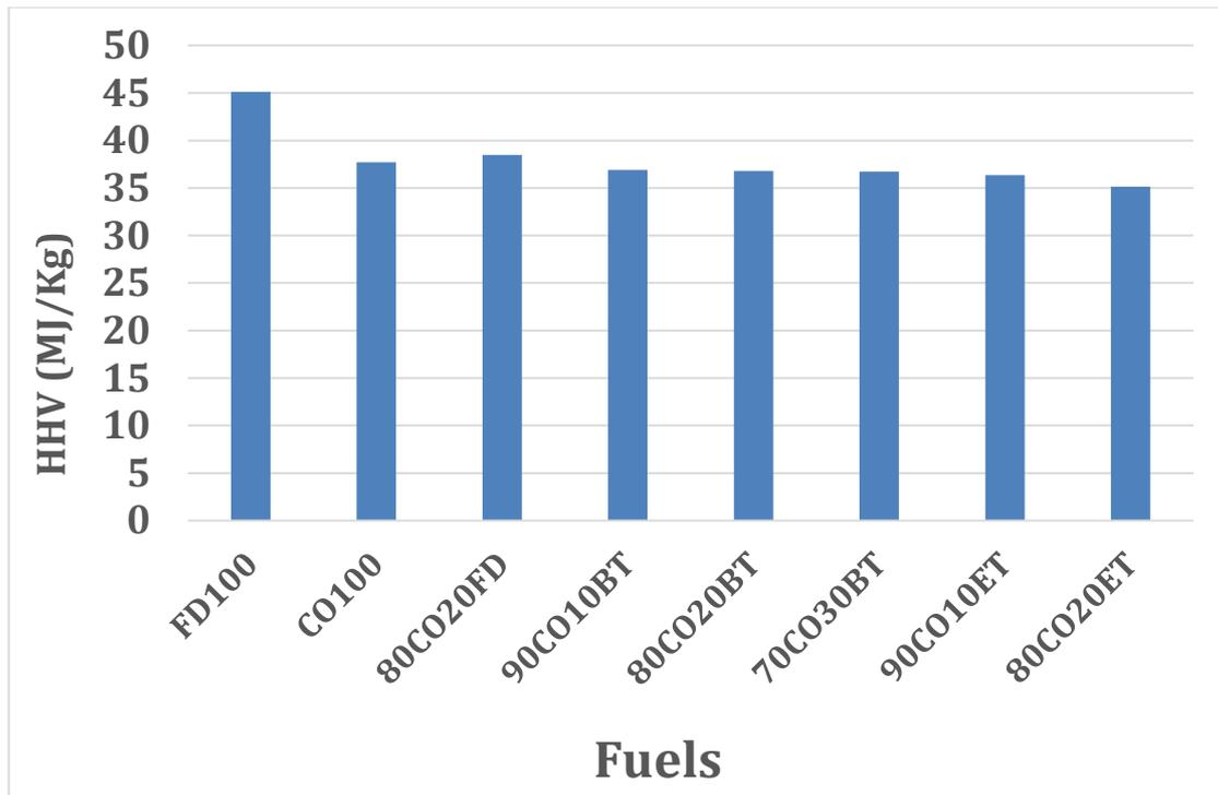
Figure 64: HHV of FD100 with CO100 and its blends.
