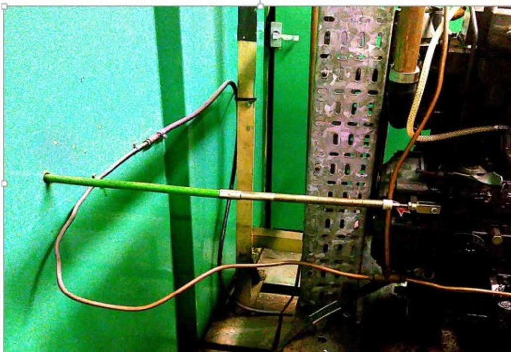
Figure 53: Emergency stop pull off the system.
