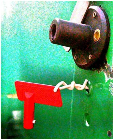
Figure 55: Electrical circuit breaker.
