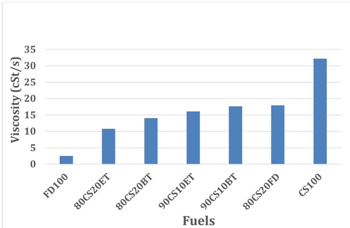
Figure 68: Viscosity of FD100 with CS100 and its blends at 40 °C.
