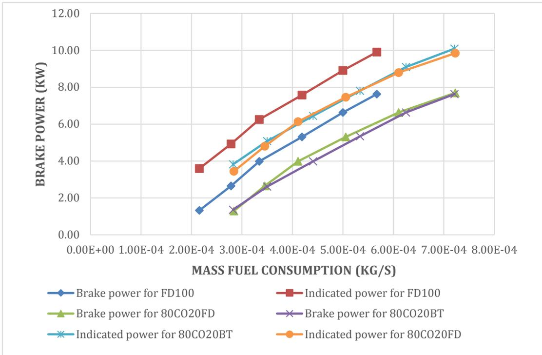
Figure 103: Brake and Indicated powers vs. Mass Fuel consumption of FD100 & CO100 and its blends.
