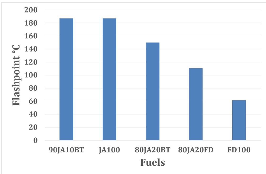
Figure 76: Flashpoint of JA100 and its blends.
