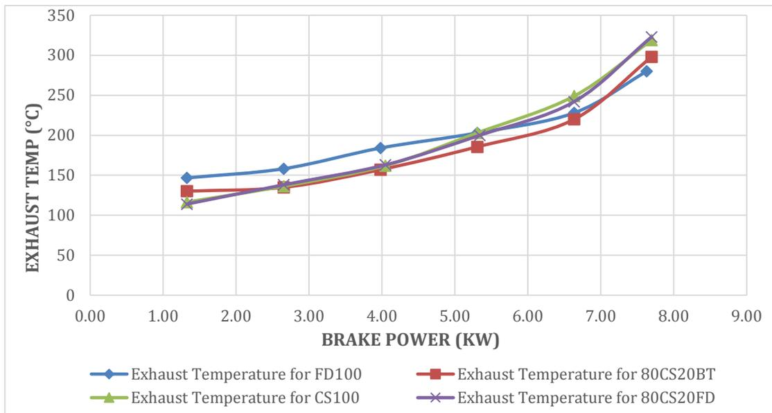
Figure 95: Exhaust temperature vs. load of FD100, CS100 and its blends.
