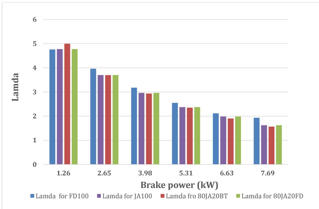
Figure 88: Lambda vs. load of FD100, JA100, and its blends.
