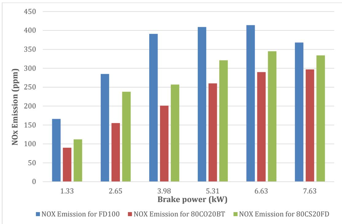
Figure 113: NO<sub>x</sub> emission vs. load of FD100, CO100 and its blends.
