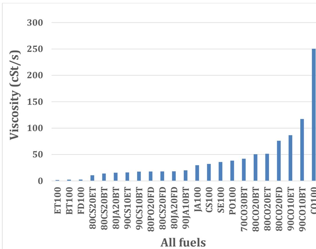
Figure 66: Viscosity of all samples at 40 °C – ASTM D7544.
