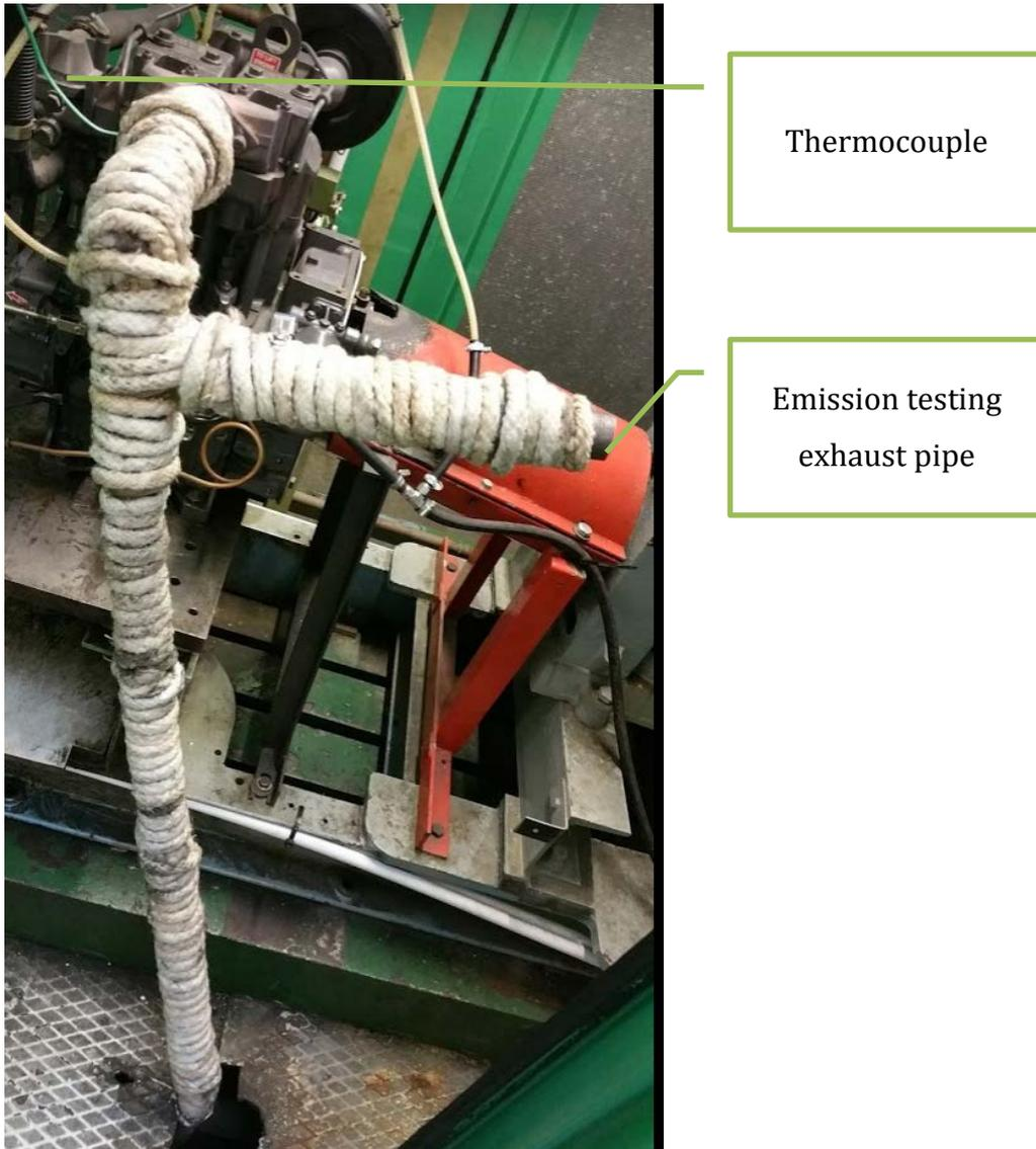
Figure 56: Measurement of exhaust temperature.
