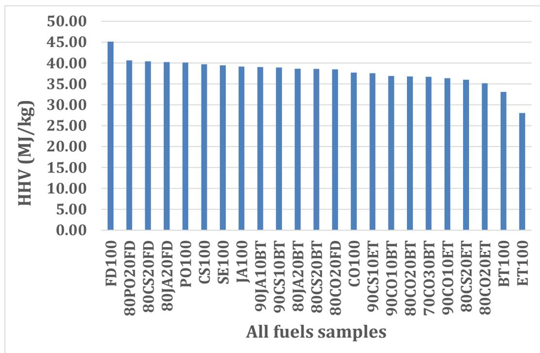
Figure 59: HHV of all samples in order from higher values to lower.
