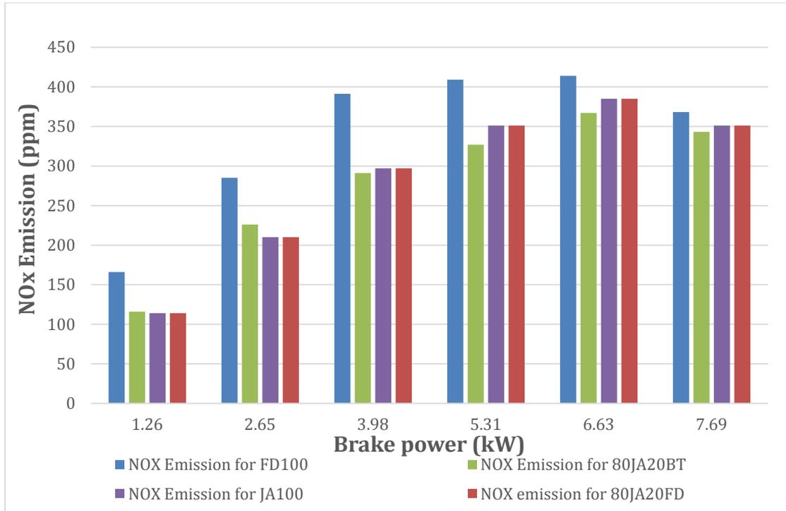
Figure 89: NO<sub>x</sub> emission vs. load of FD100, JA100 and its blends.
