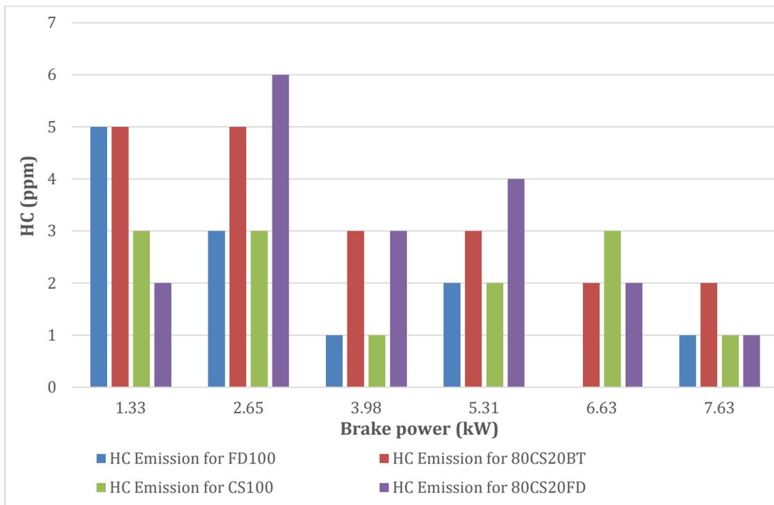
Figure 99: HC emission vs. load of FD100, CS100 and its blends.
