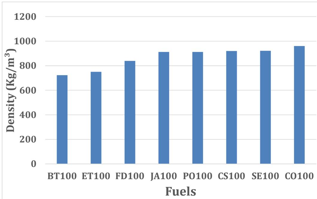
Figure 71: Density of FD100 with all pure samples.
