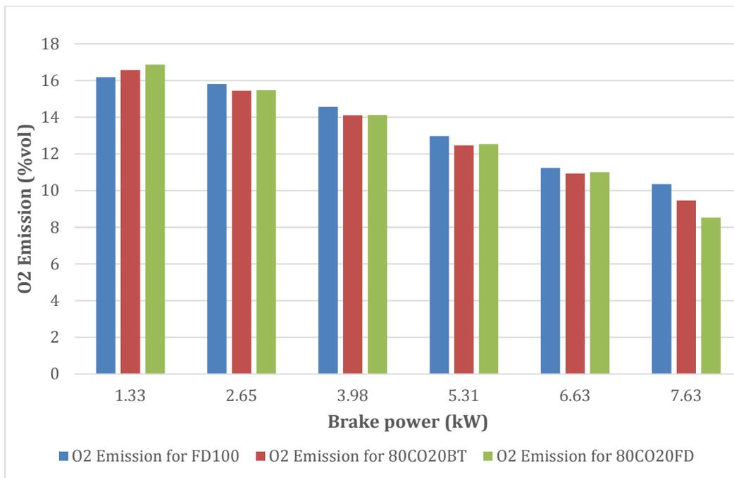
Figure 109: O2 emission vs. load of FD100, CO100 and its blends.
