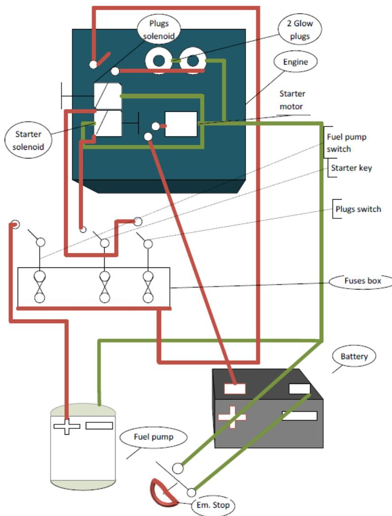
Figure 54: Engine electrical Circuit modification.
