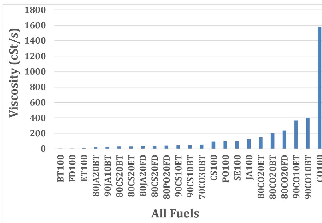
Figure 65: Viscosity of all samples at 14 -25 °C –ASTM D7544.
