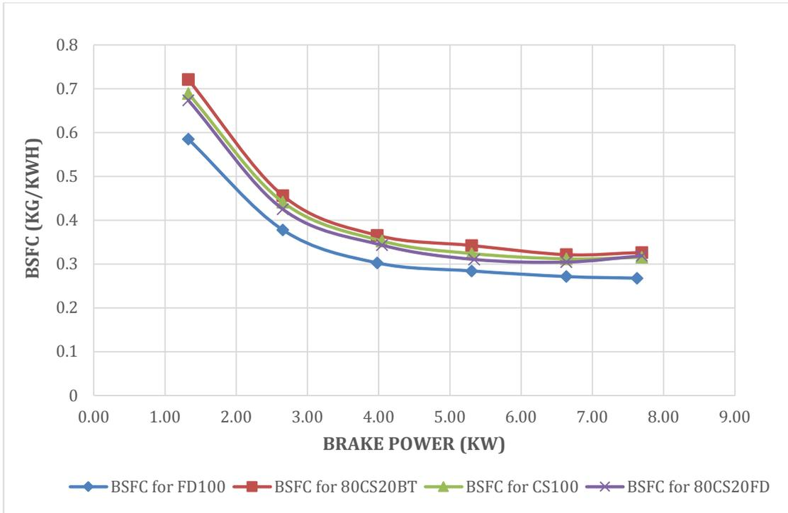
Figure 92: Brake Specific Fuel Consumption vs. load of FD100, CS100, and its blends.
