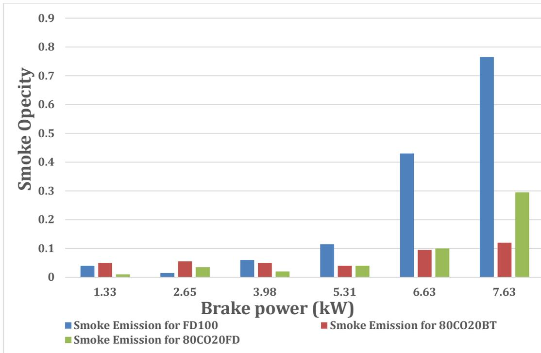
Figure 114: Smoke emission vs. load of FD100, CO100 and its blends.
