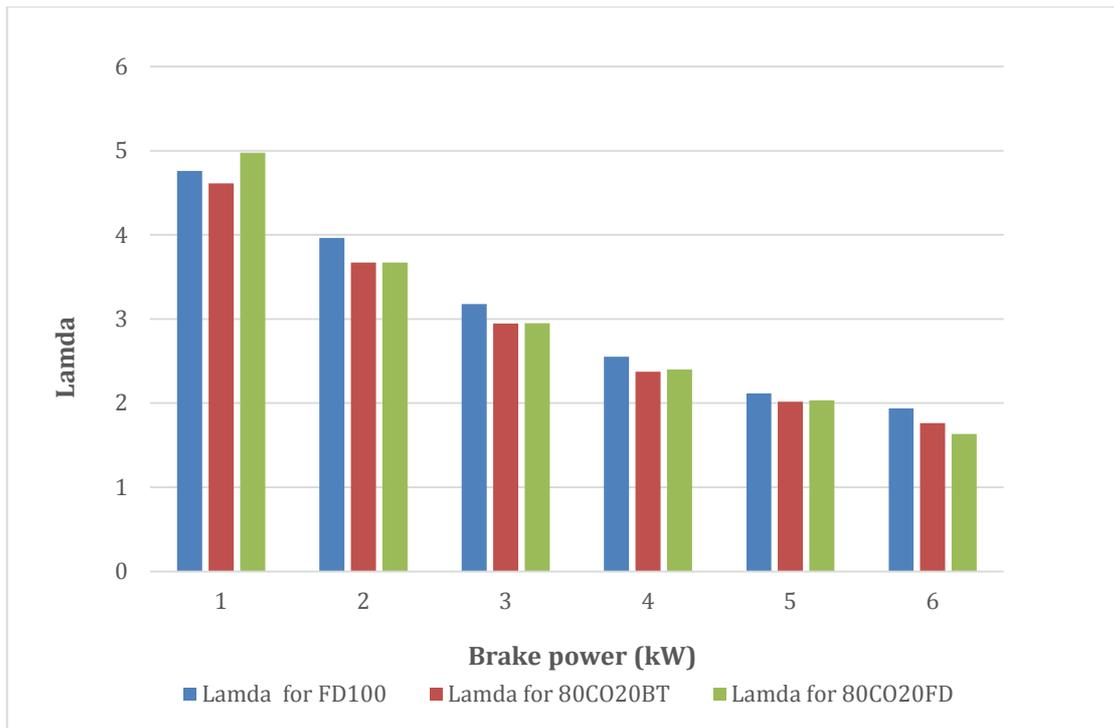
Figure 112: Lambda vs. load of FD100, CO100, and its blends.
