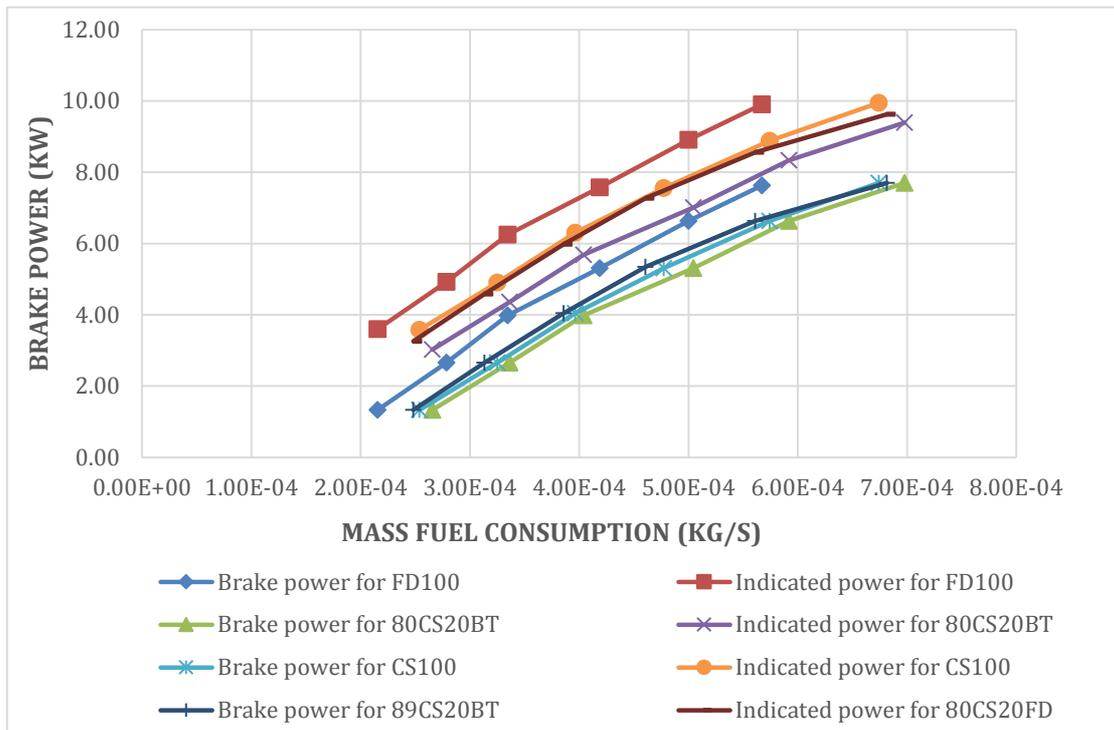
Figure 91: Brake and Indicated powers vs. Mass Fuel consumption of FD100 & CS100 and its blends.
