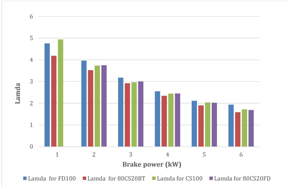
Figure 100: Lambda vs. load of FD100, CS100 and its blends.
