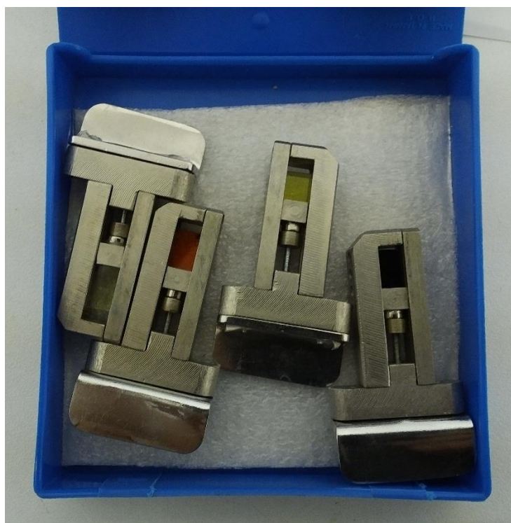
Figure 4.4 The LAKK-M filters. From left to right - filters for excitation wavelengths of UV (365 nm), green (532 nm), blue (450 nm) and red (635 nm).
