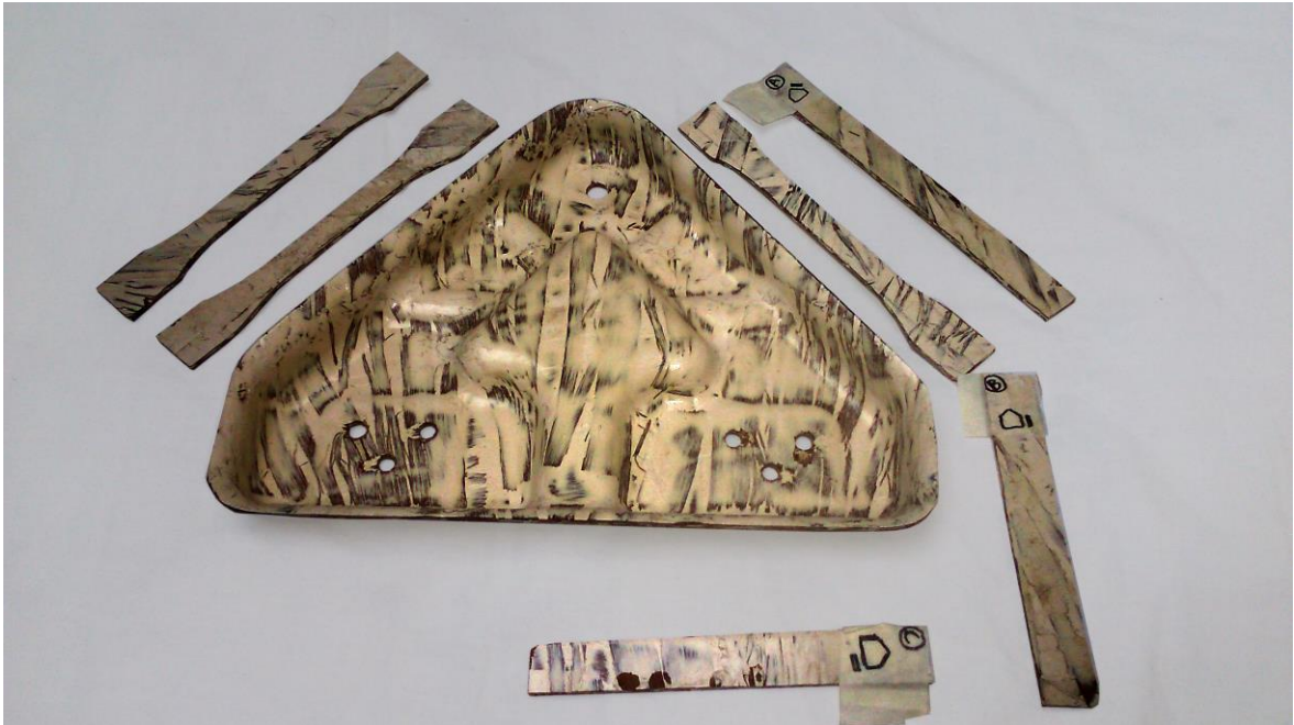
Figure 6.8, Source of tensile samples.
