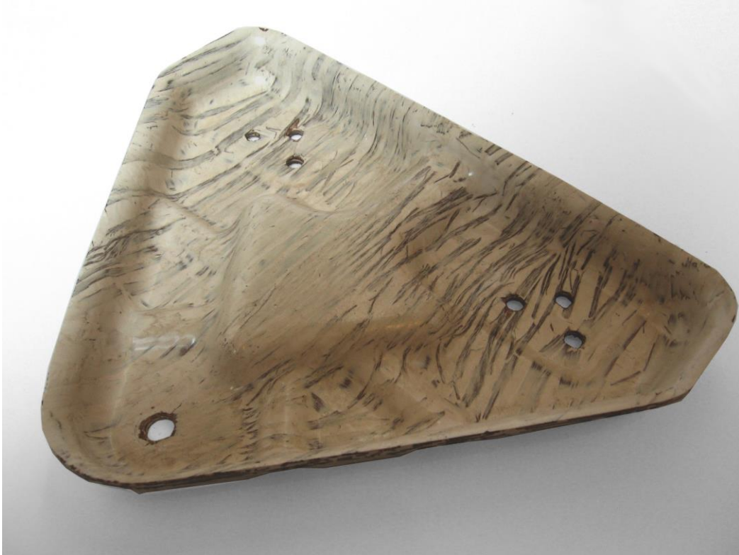
Figure 5.64, Trimmed half wishbone moulding
