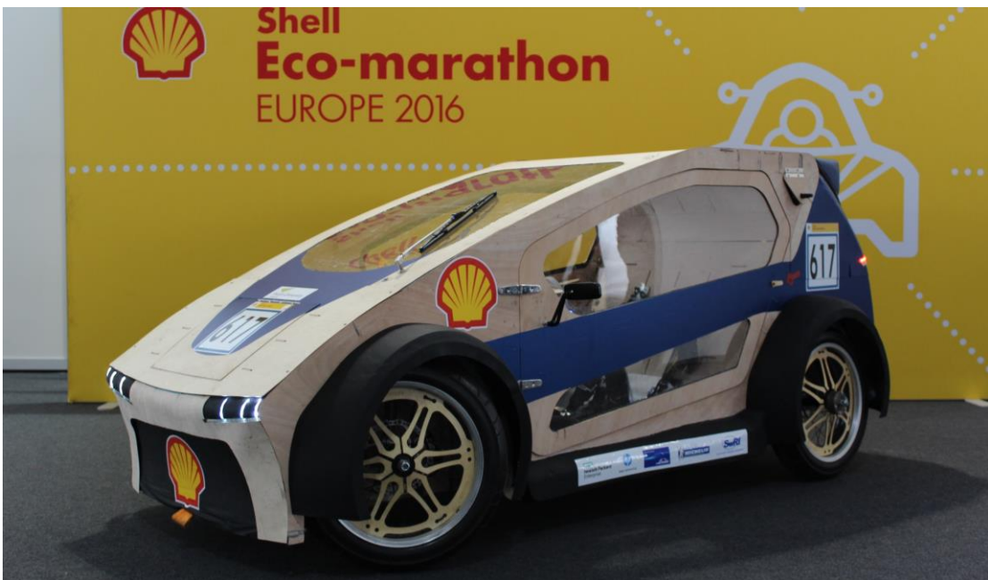
Figure 2.22, 2016 Aston EcoCar - flat pack construction, subject of main study.
