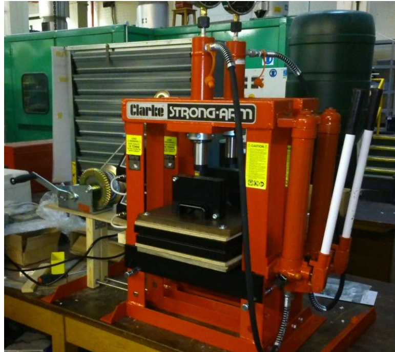
Figure 5.47, Lab press, maximum pressure 20T, maximum temp 230°C.
