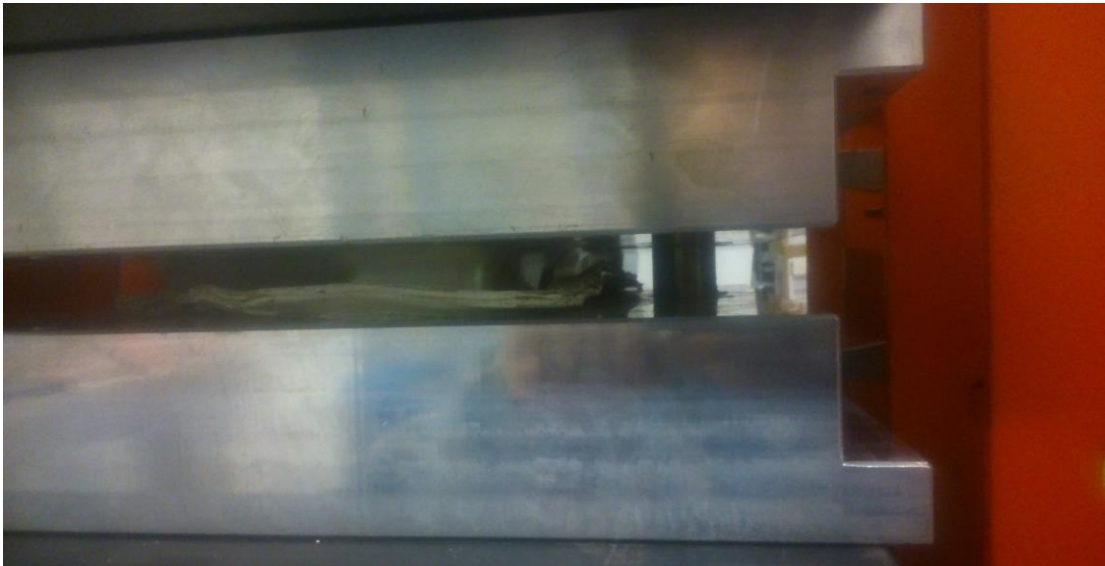
Figure 5.61, Pre-heating the veneer/Blome blank in the mould
