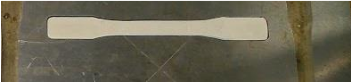
Figure 4.2, Layers of Biome and veneer stacked into a cavity
