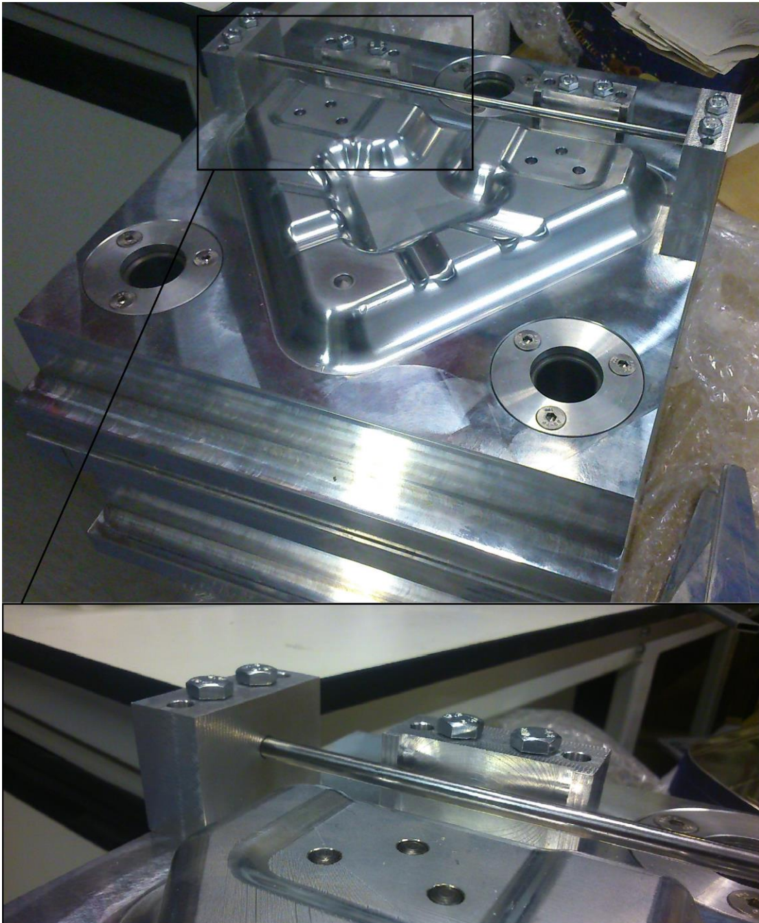
Figure 5.56, Aluminium male mould for the wishbone part, Bottom: Detail of the pivot positioning bar and mould surface.
