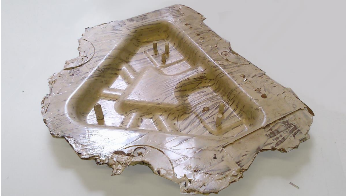
Figure 5.63, Wishbone moulding with flashing and risers.
