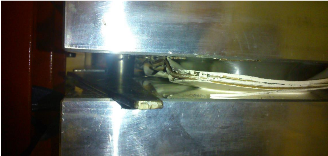
Figure 5.62, 3mm spacer strip between male and female moulds
