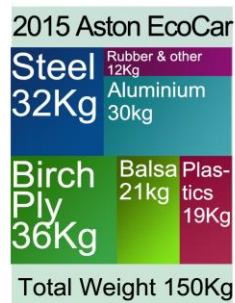
Figure 2.27, Materials comparison Graphic displaying the proportion of materials by weight for the 2015 Aston EcoCar, the VW golf Mk.5 (Volkswagen, (2008): p.22,) and the Average European Car (European Commission, 2008: p.53,).
