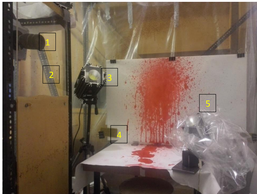
Fig. 2 Set-up for high speed image recording and collection of bloodstain patterns; 1-Photron SA-5 camera, 2-camera protection booth, 3-10 000 lm LED light, 4-paper for collection (horizontal and vertical), 5-8000 lm LED light
