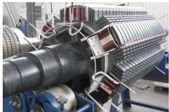
Fig. 2. Arrangement of the rotor winding (concentric).
