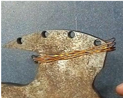
Fig. 8. Installation of the rotor coils.
