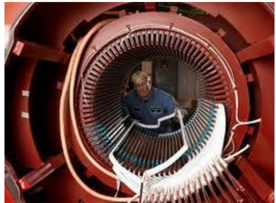
Fig. 1. Arrangement of the stator winding (distributed).
