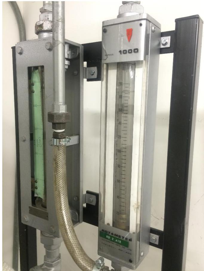
Figure 5.5: Picture of the primary and secondary rotameters used for the experiment.
