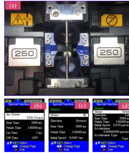
Fig. 2. (a) Photograph of the arc discharge technology employing a commercial fusion splicer (FSM-100P); (b) first step (discharge); (c) second step (move fiber); (d) third step (jump).
