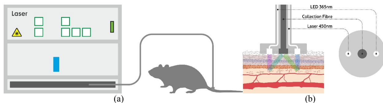
Figure 1. Schematic representation of the setup used to study the transport of fluorescent coloured liposomal nanoparticles in mice using the “LAKK-M” laser system: a) overall view of the experimental setup; b) fibre optic probe.
