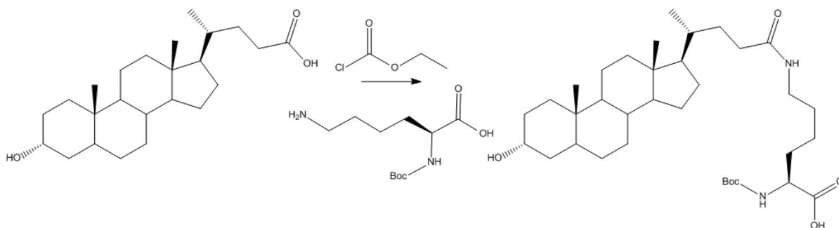
Scheme 23: Mixed anhydride method of attaching an amino acid group to a bile acid.
