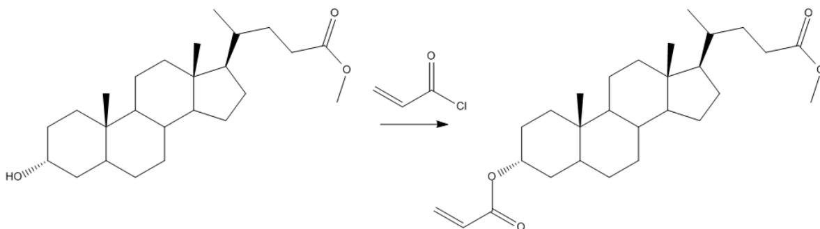
Scheme 15; Formation of an ester linkage at the 3-OH position on methyl lithocholate, using acryloyl chloride.
