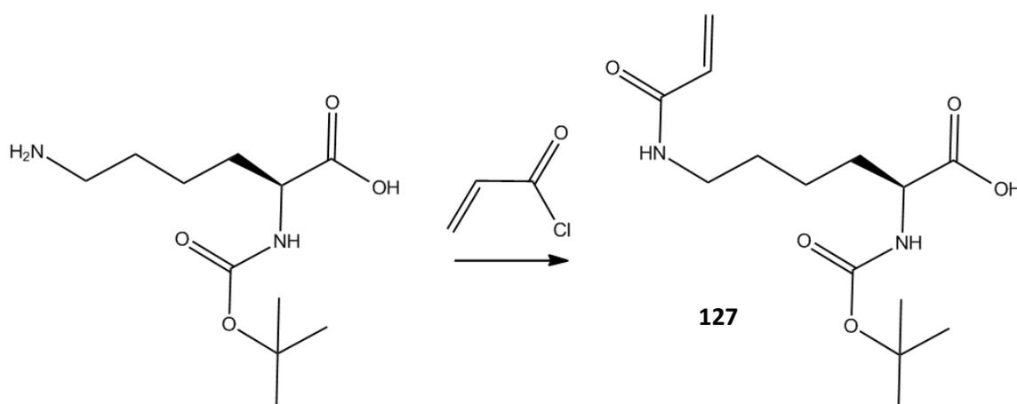
Scheme 22: Compound **127**; a monomeric polymerizable amino acid analogue.
