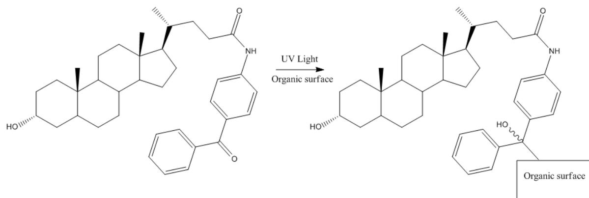
Scheme 25: Binding of benzophenone based bile amides to organic surface containing C-H bonds.
