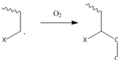
Scheme 8; Peroxy radical formation by allowing free radical polymerisation to occur in an oxygen environment.
