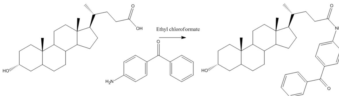
Scheme 24: Synthesis method for a coupling between lithocholic acid and 4-amino-benzophenone.
