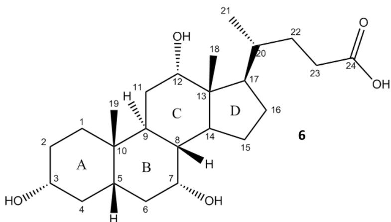
Fig 6: Naming and numbering system of the steroidal rings (compound 6).
