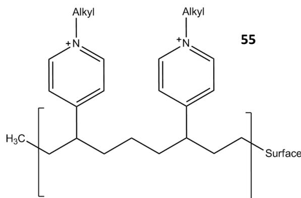
Fig 21: An antimicrobial polymer, with quaternary nitrogen ions, used in the prevention of *S. aureus*. Modified from (Tiller et al., 2001) (compound **55**).
