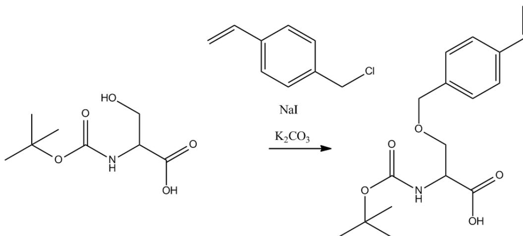
Scheme 19: Attempted coupling of Boc-Ser-OH with vinyl benzyl chloride.
