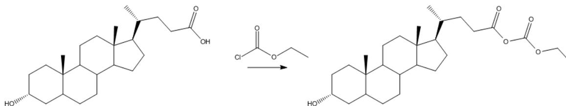
Scheme 6: Production of mixed anhydride using ethyl chloroformate.
