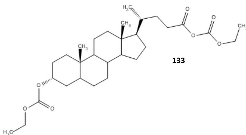
Fig 28: Mixed anhydride of lithocholic acid with an unwanted carbonate formation on the 3-OH position, due to excess ethyl chloroformate (compound **133**).
