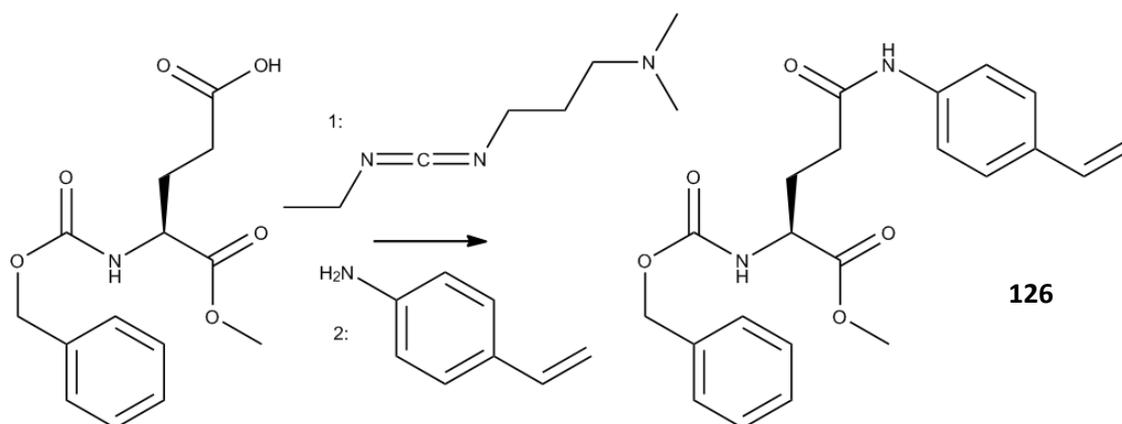
Scheme 21: Synthesis of manipulated amino acid (**126**) using a carbodiimide coupling agent.
