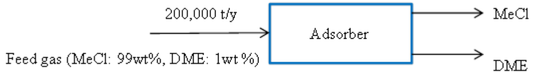
Fig. 4.7: Process flow diagram for throughput entering adsorber.
