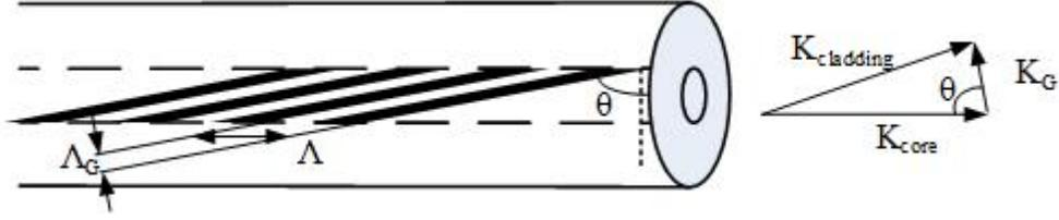
Fig. 2. The schematic and vector phase matching diagram of an Ex-TFG.
