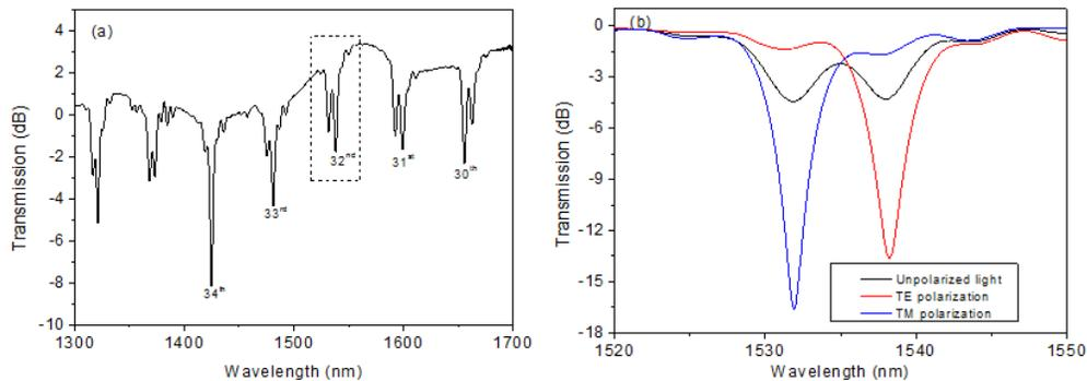
Fig. 6. The transmission spectra of  $81^\circ$ -TFG: (a) a series of dual-peak resonances from 1300 to 1700 nm and (b) zoomed dual peaks at around 1530nm when launched with unpolarized light (black line) and orthogonally polarized lights (blue line – TM and red line - TE).
