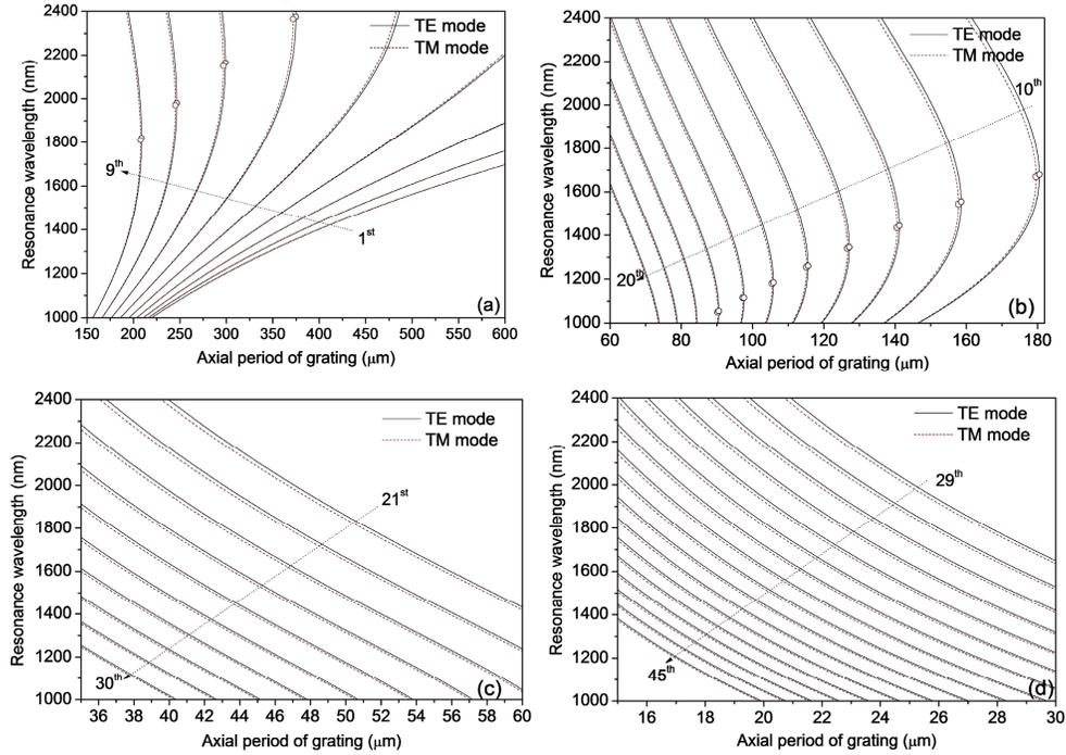
Fig. 3. Simulated resonance wavelength versus the axial period of Ex-TFG with TE (solid line) and TM (dash line) modes for different orders: (a)  $m = 1$  to 9; (b)  $m = 10$  to 20; (c)  $m = 21$  to 30; (d)  $m = 29$  to 45.
