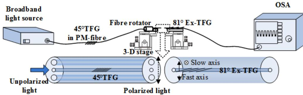
Fig. 7. The experimental setup investigating the polarization dependent loss of the 81°-TFG.
