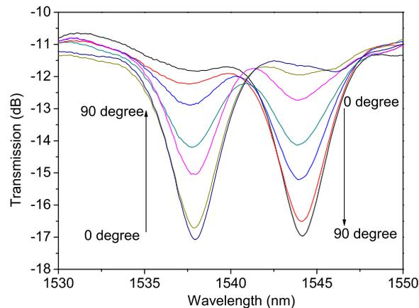
Fig. 8. the transmission spectra of 81°-TFG measured by launching a linear polarization light with different azimuth angles with respect to the fast axis of grating.
