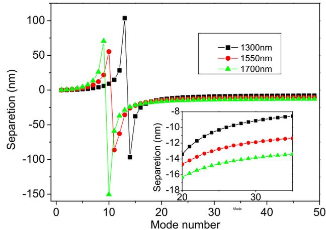
Fig. 4. The separation of TM and TE resonance cladding modes as a function of mode order for 1300nm, 1550nm and 1700nm. Inset in Fig. 4 shows the enlarged separation data from mode 20 to 35.
