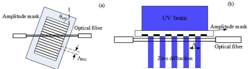
Fig. 5. Schematic of (a) the front view and (b) the top view of amplitude mask and fiber with 0 order diffraction inside the fiber core.
