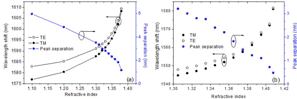
Fig. 9. The simulated (a) and experimental (b) results of peak separation of 32nd dual peak cladding mode versus surrounding medium refractive index.
