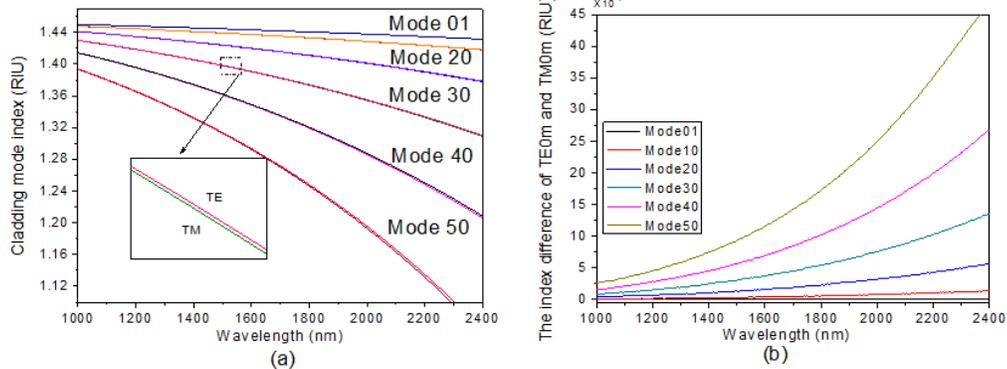
Fig. 1. (a) The mode indexes of TE and TM cladding modes (inset shows the enlarged scale for 30th modes) and (b) the mode index difference between TE and TM cladding modes as a function of the wavelength.
