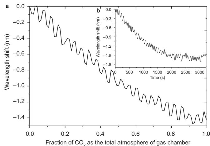
**Figure 6** Typical spectral behavior of the fiber sensor with an LSP wavelength resonance at 1390 nm, (a) as a function of the fraction of CO<sub>2</sub> in the surrounding atmosphere (b) showing the spectral response of the sensor with respect to the time taken for the experiment to be completed.
