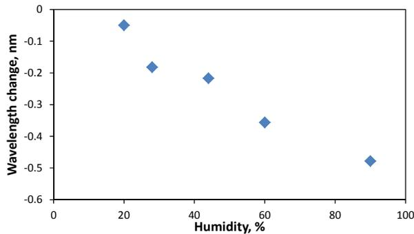
Fig. 6 The wavelength changes vs. the environmental humidity
