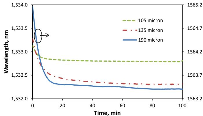
Fig. 7 Time responses of POFBGs with different diameters
