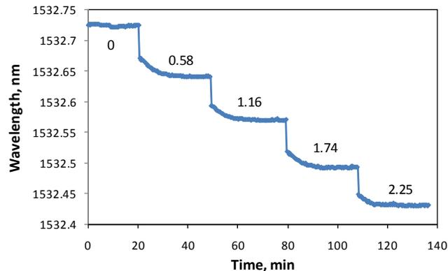
Fig. 8 The wavelength response of POFBG with a diameter of 135  $\mu\text{m}$  with input power from a 1480 nm laser diode varying from 0, 0.58 mW, 1.16 mW, 1.4 mW to 2.25 mW.
