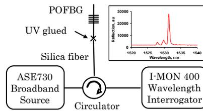
Fig. 2 Experimental arrangement
