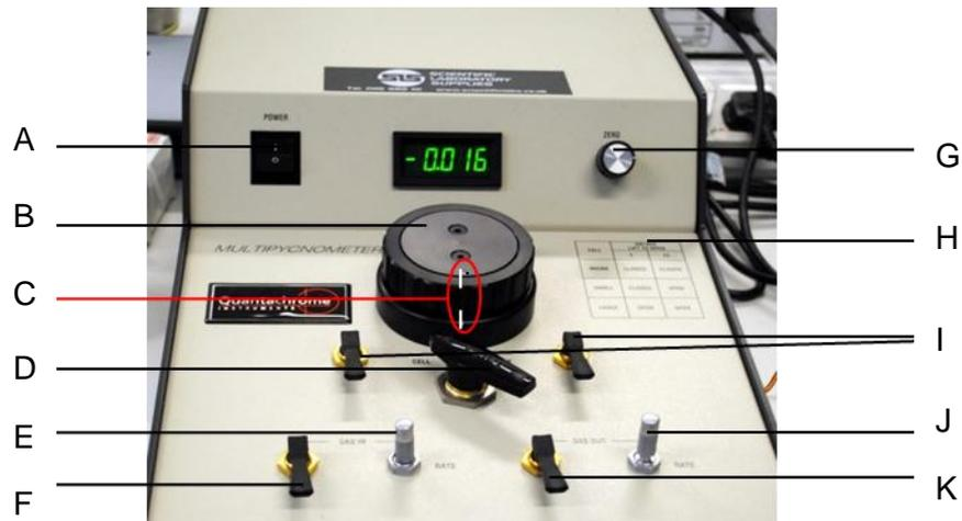
Figure A 3: Photograph of the front panel of multipycnometer (Quantachrome instruments, Model number MUP- 6DCE). Labels A-K corresponds to operation procedure outlined below and is in brackets next to applicable procedure.
