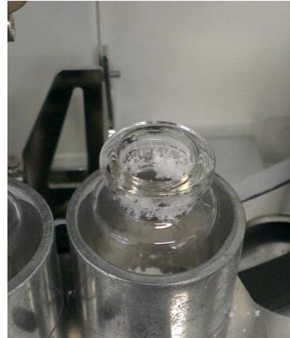
**Figure 5.11: Gravimetric or mass filled lyophilised powder losses due to sticking to inner walls of dosing head (A) and brim of glass vial (B).**
