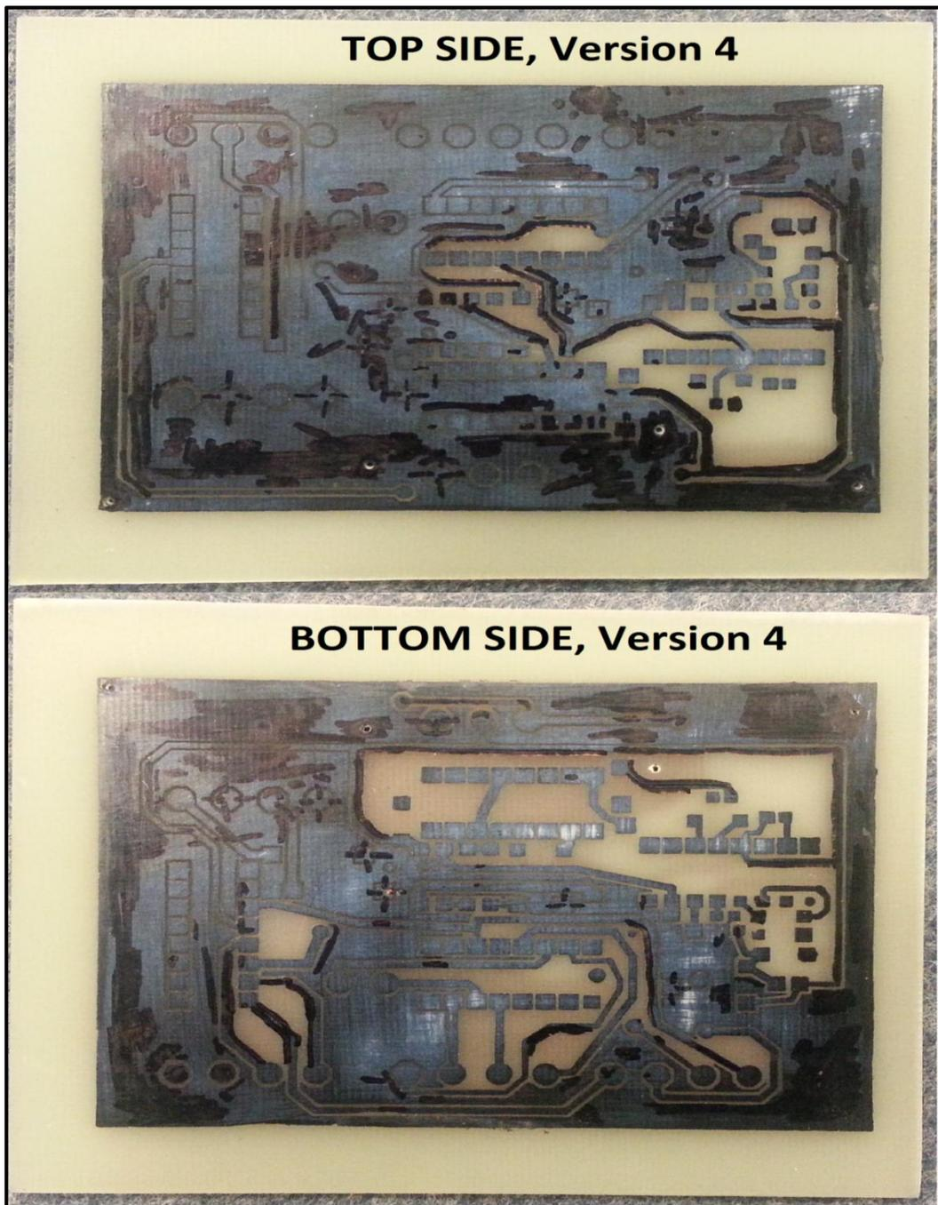
**Figure 7-10: Shows top side and bottom side of PCB board designed (circuit in Figure 7-4) for version 4 of the device. This was manufactured using the 'toner-transfer' method.**
