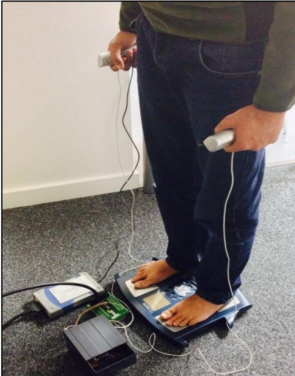
**Figure 11-1: Shows a volunteer undergoing bio-impedance examination on device version 4. As stated in section 9.1 the internal circuitry of the Tanita device pictured is replaced with device V4.**
