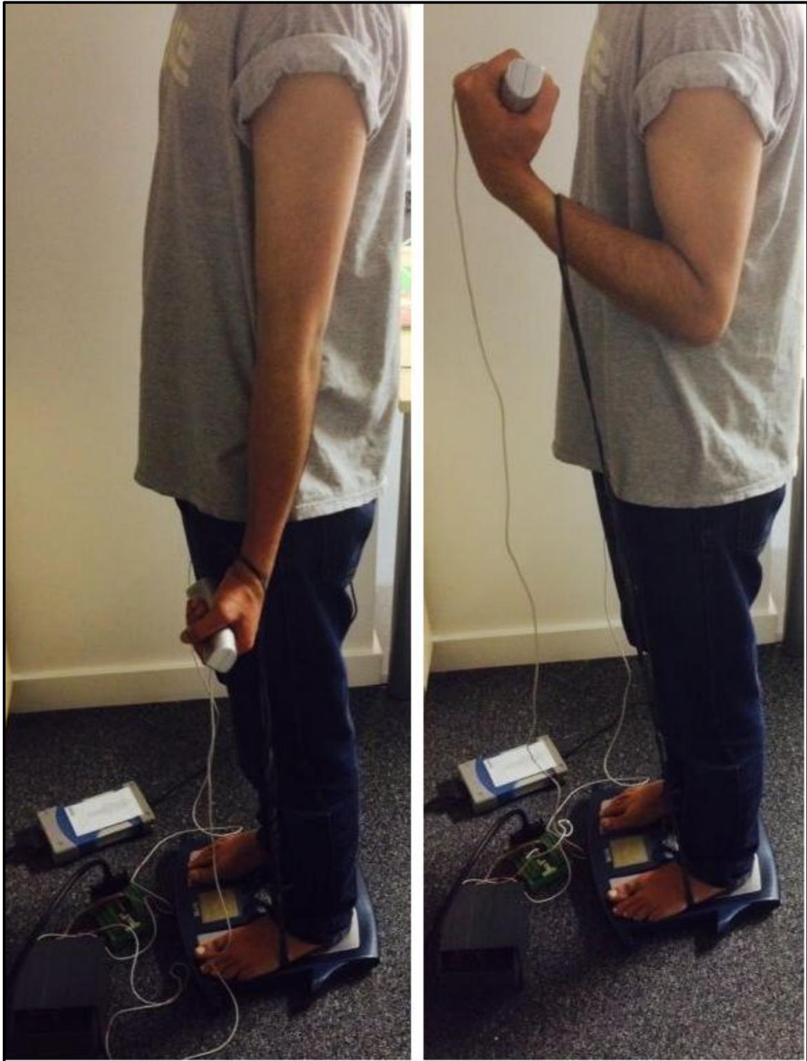
**Figure 11-10: Shows the volunteer undergoing impedance measurement while his arm is flexed. Note the elastic band around the wrist and the change in area of cross section of the arm before and after flexing the arm. The procedure utilized V4 of the bio-impedance device and the signals are recorded using Agilent U2531A.**
