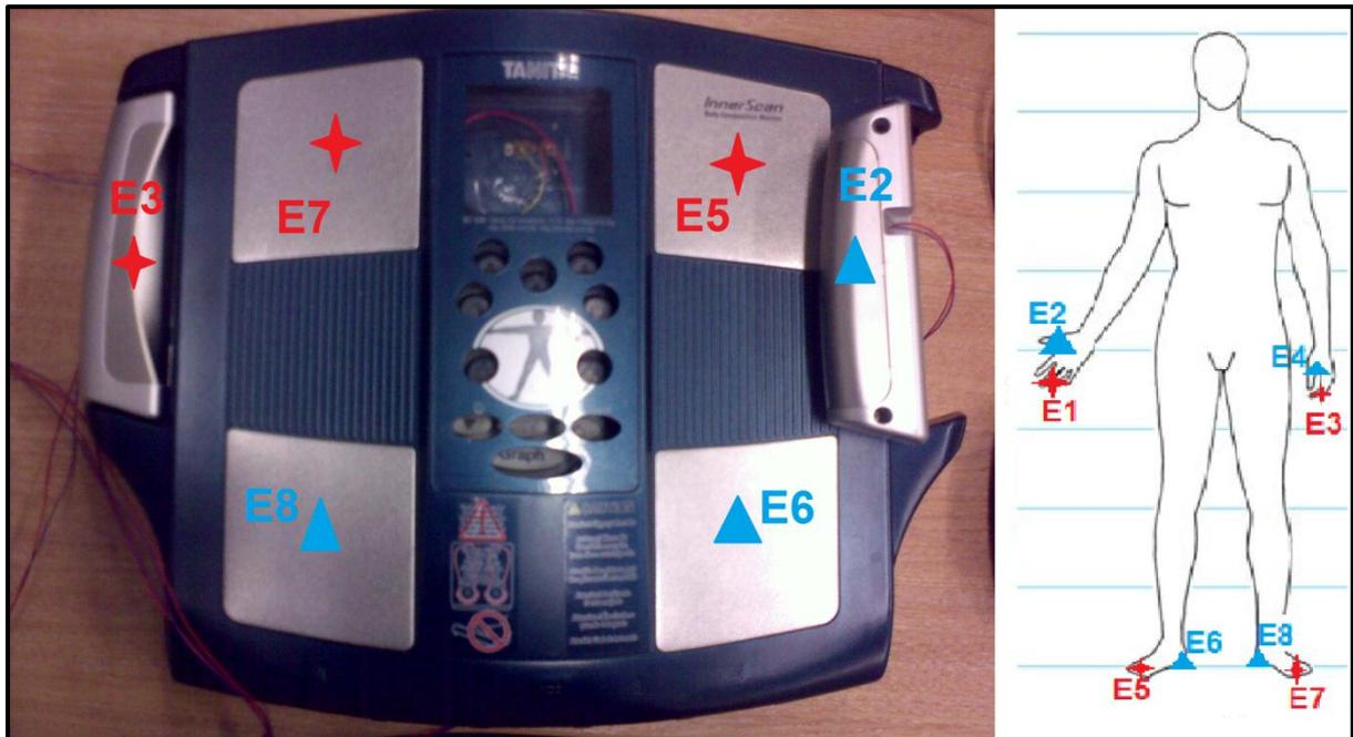
**Figure 5-9:** Shows the electrodes used in the present system and their labels on a subject’s palms and underside of their foot. In essence the subject would stand on the foot electrodes and grab the hand electrode attachment. Note: electrodes E4 and E1 are hidden from view.
