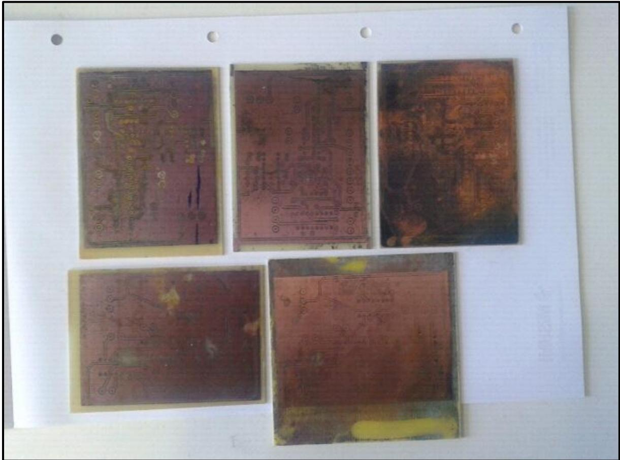
**Figure 6-3: Shows failed attempts to manufacture the SBIA PCB layout in Figure 6-2.**
