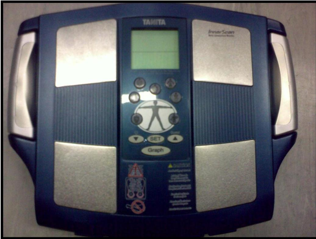
**Figure 3-1: Shows the Tanita BC-545 and 8 foot and hand electrodes (two hand electrodes hidden from sight).**
