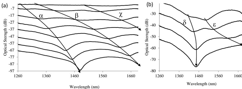
**Figure 3** Transmission spectra of Ge/SiO<sub>2</sub>/PtAu as a function of refractive index of surrounding medium, (a) index variation from 1 to 1.36 and (b) index variation from 1.365 to 1.395.
