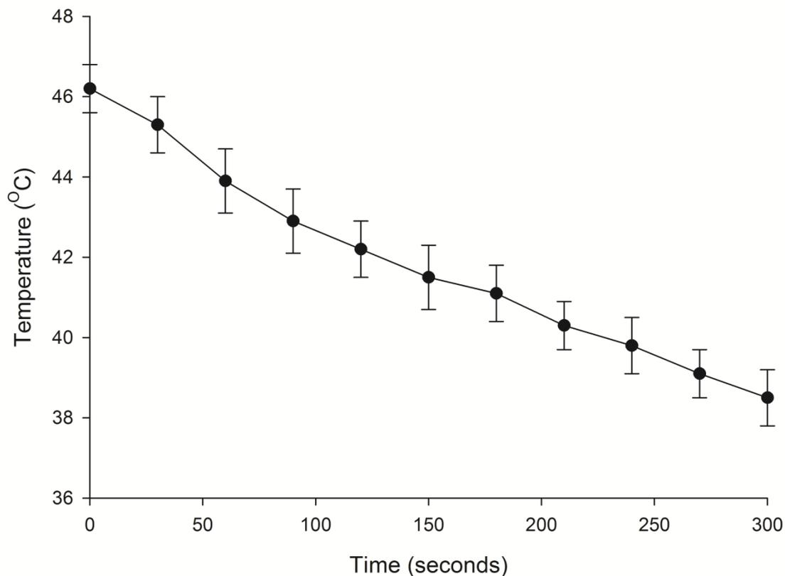
**Figure 5.3.1:** Mean temperature (°C) of the MGDRx EyeBag at 30 second intervals immediately after heating for 5 minutes. Error bars represent  $\pm 1$  SD.
