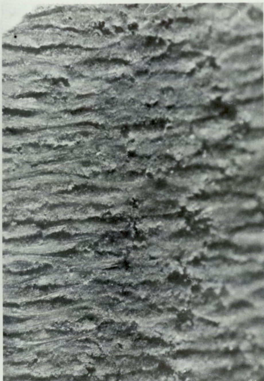
BORE SURFACE AS DRILLED 320 rev/min 0.40 mm/rev
