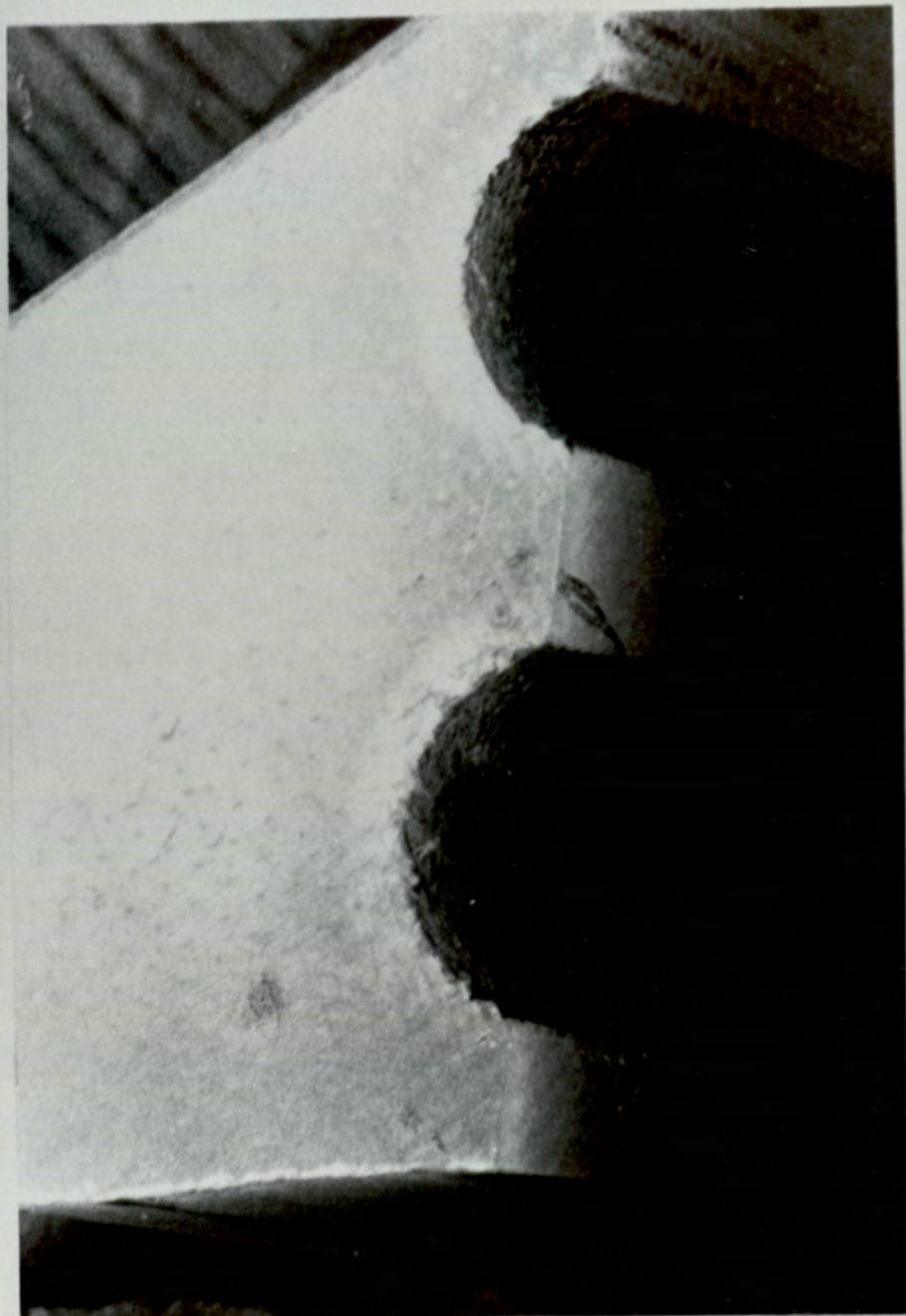
BURR WITH DELAMINATION EXIT OF DRILL 1190 rev/min 0.068 mm/rev
