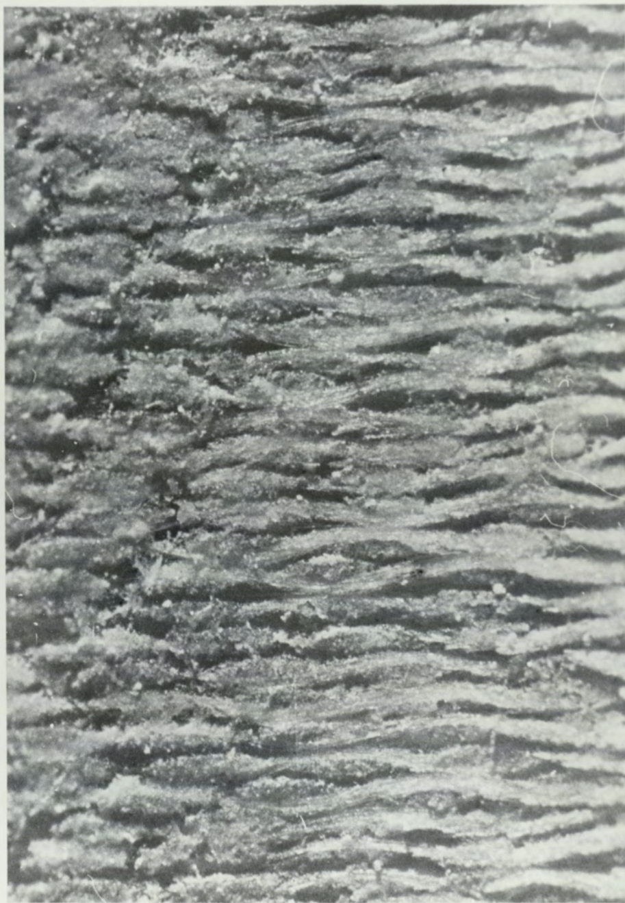
BORE SURFACE AS DRILLED 530 rev/min 0.25mm/rev
