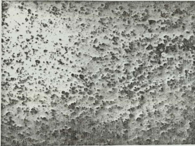
Fig 8.7 Uneven inclusion density corresponding to troughs in the surface of the electrodeposit. Chromium diboride in copper, parallel to surface. x 50 enlarged x 3.
