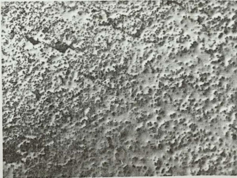
Fig 8.3 Increase in inclusion density at the edge of a specimen. silicon carbide in copper, parallel to surface. x 50 enlarged x 3.
