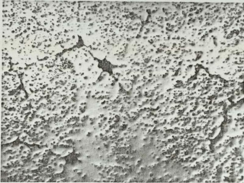
Fig 8.4 High inclusion density in the edge build up:
