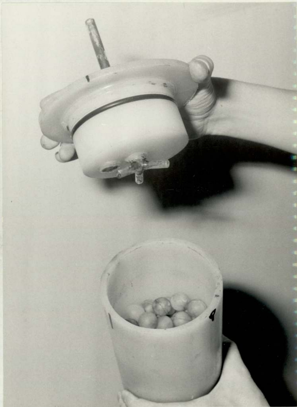
Plate 6. Experimental filter with lid removed showing glass distributor and medium of plastic spheres.
