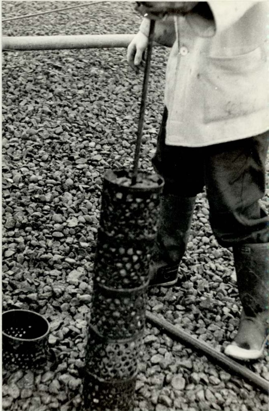
Plate 5. Shaft removed for examination showing vertical arrangement of containers.
