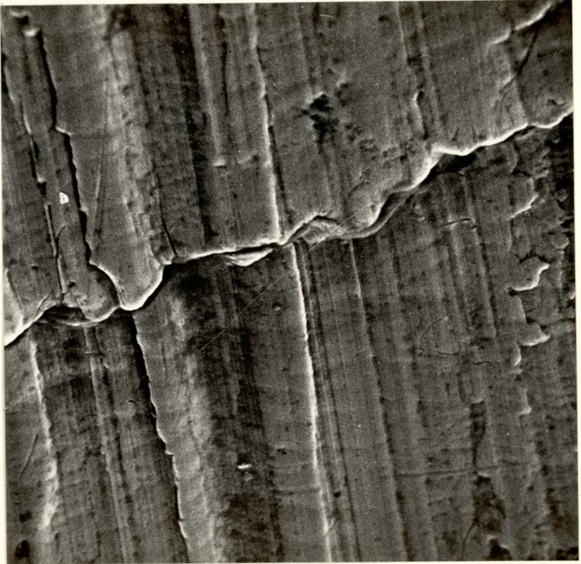
Fig. 1.16. Effect of Abusive Grinding on Distributor Cam Track.
