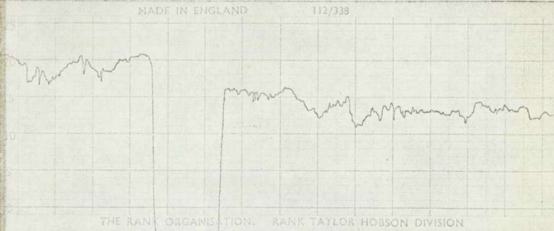
FIG. 6-12 TALYSURF PROFILES . SPECIMEN. 4.
