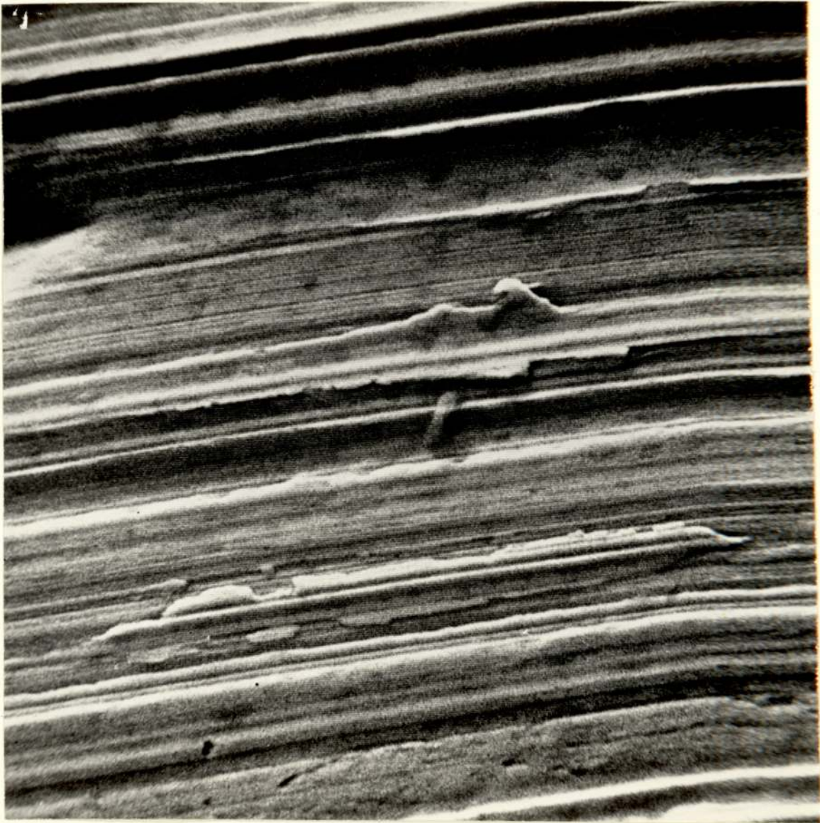
Fig. 1.8. Surface Ground Specimen showing "Wave Formation"
