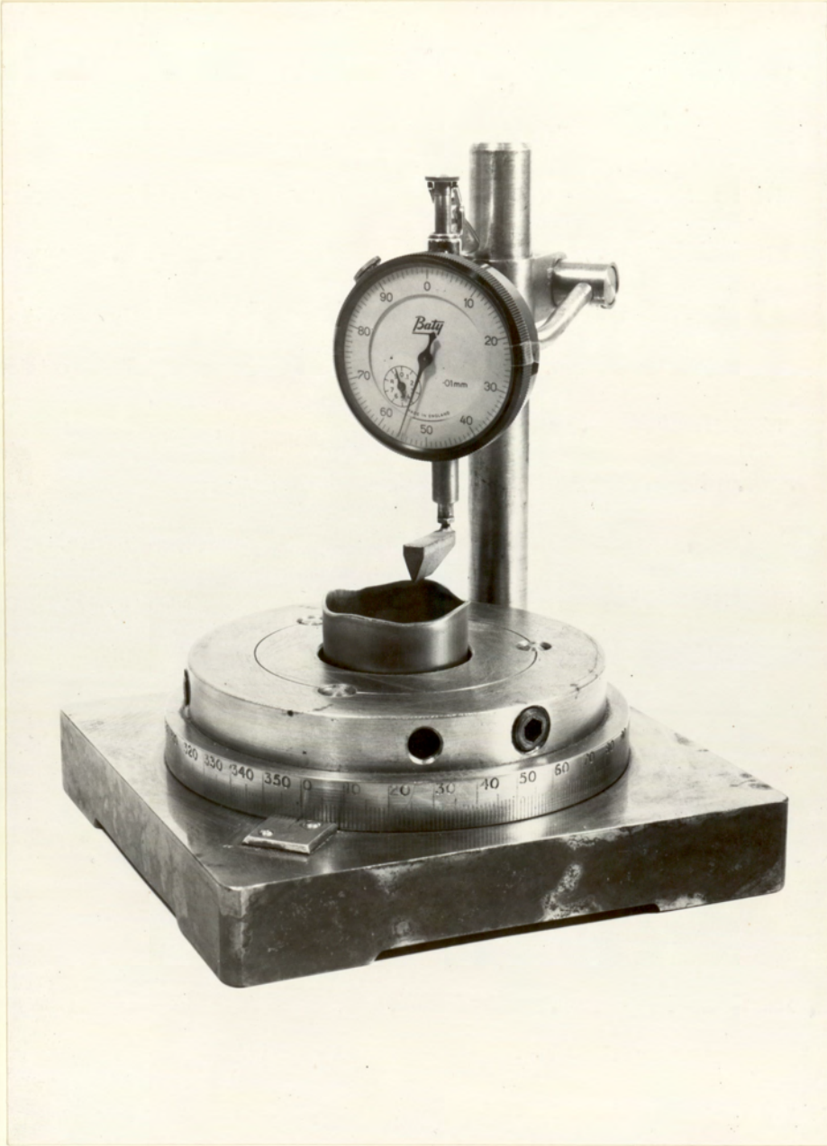
Fig. 19. Jig for measurement of earing
