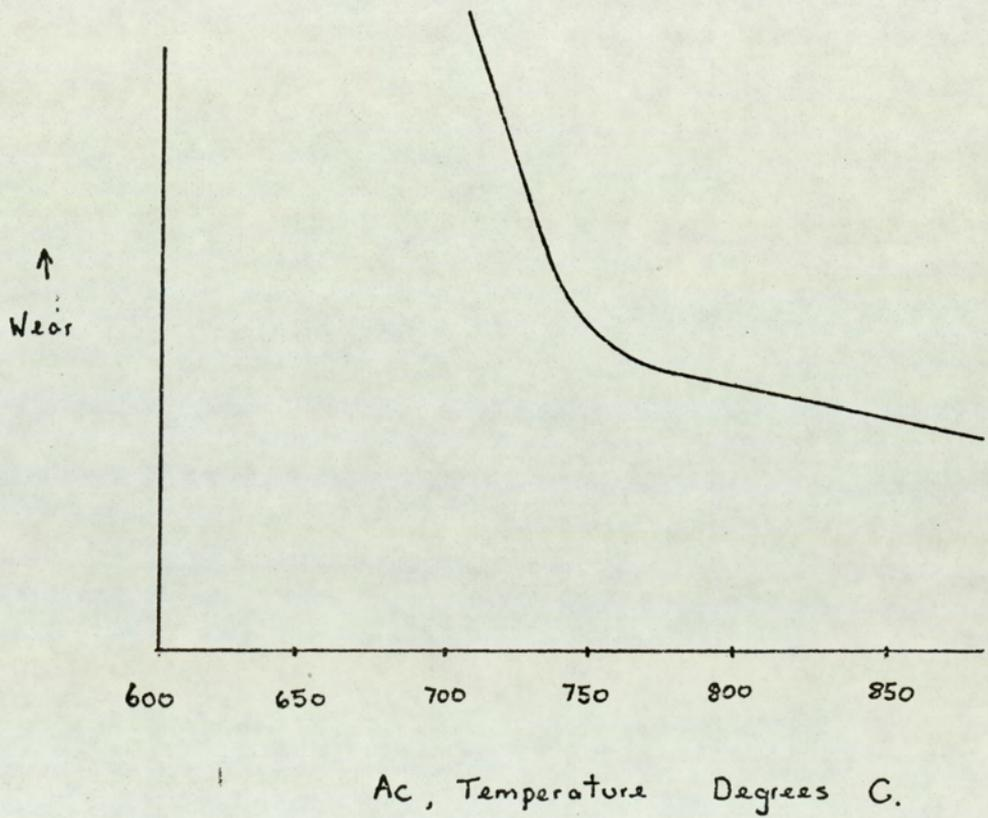
The Dependence of wear on AC<sub>1</sub> Temperatures
