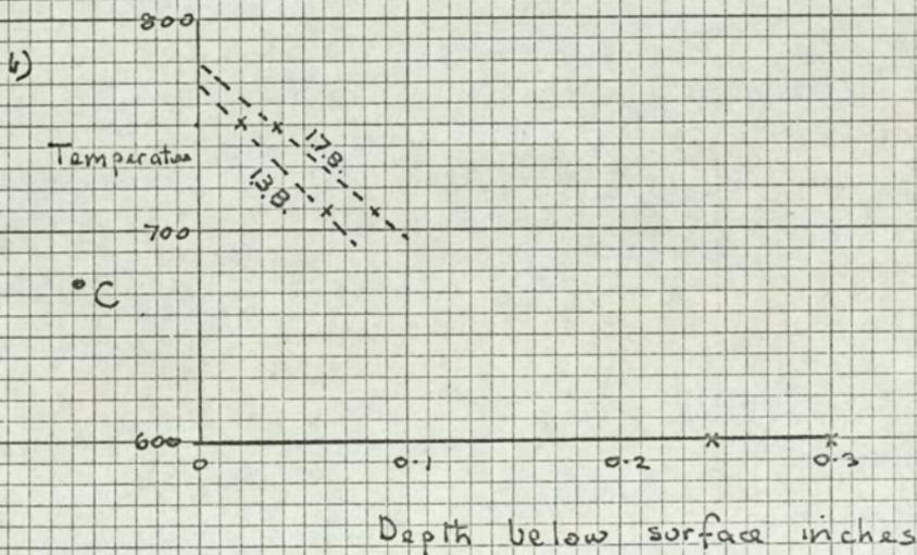
C is the limit of the softened material; the maximum temperature attained at C is insufficiently high to cause appreciable tempering and is designated the original tempering temperature.
