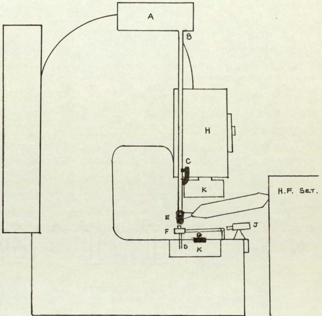
A Schematic Diagram of The Experimental Press.
