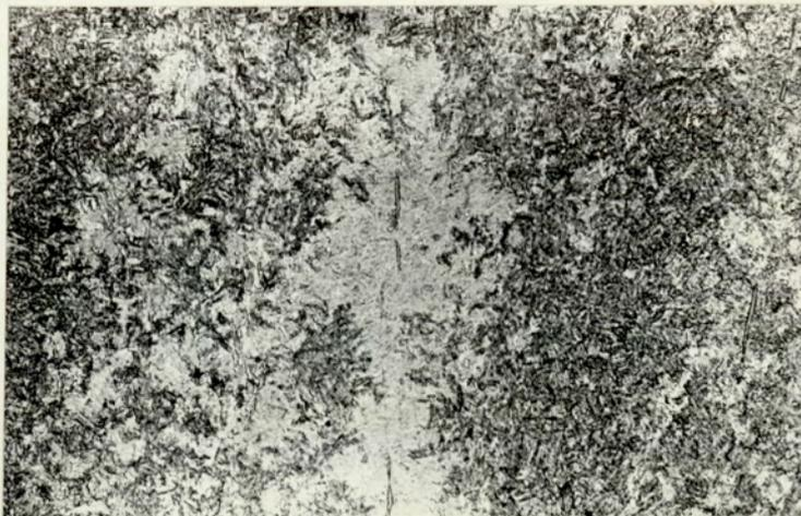
The Inhomogeneity of the Heat Treated Material.
