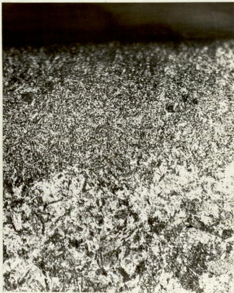
Vertical Section, Showing Transformed Edge.
