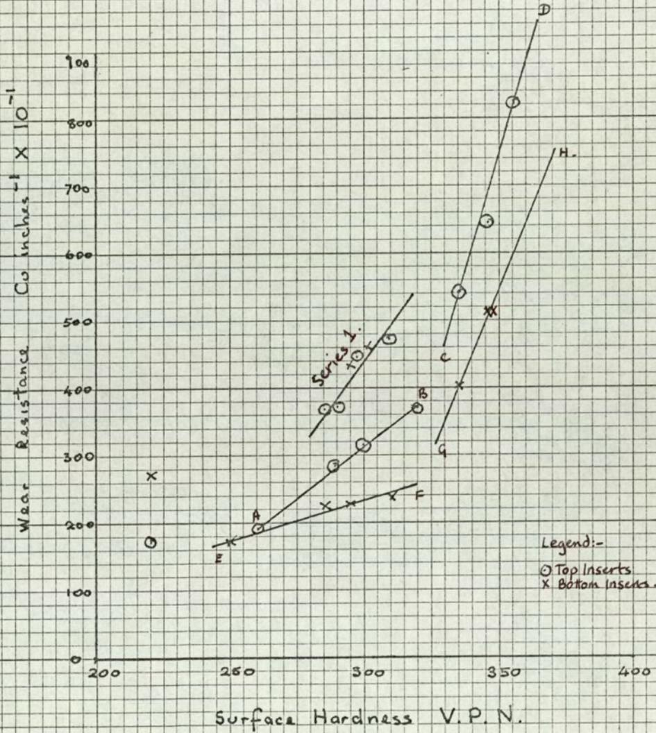
greater than that of the softer inserts, and that the wear resistance of the pearlitic insert 2.8 was relatively greater than would be expected from the trend of the quenched and tempered inserts.
