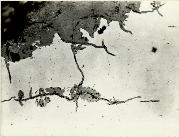
Thermal Fatigue Cracks in Scale Penetrations.
