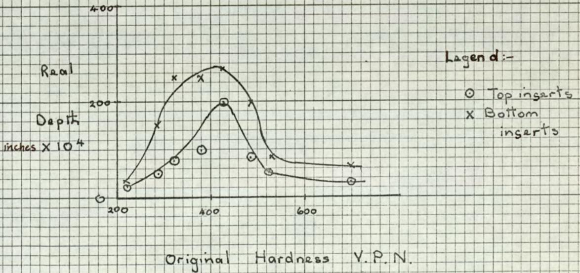
The depth of thermal fatigue cracks at different hardnesses.
