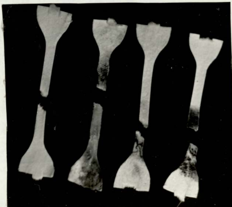
d. Paper strips tested for tensile strength showing location and nature of break areas. From left, a control strip, and strips showing colonisation by fungal species with respectively, rapid, slow, and moderate growth rates.
