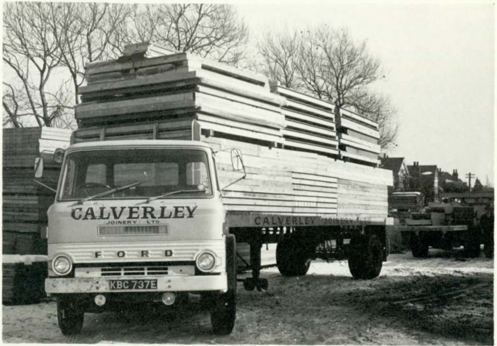
Fig. 6.9 Prime mover and trailer loaded with house panels
