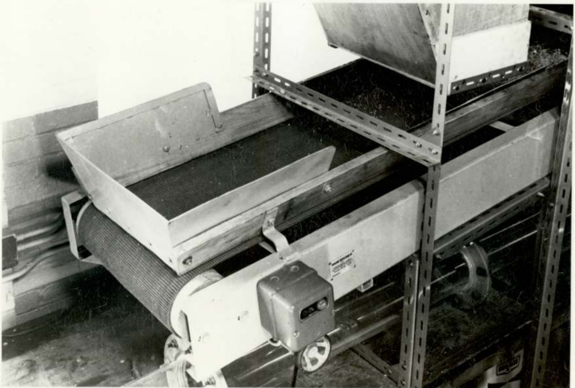
FIG 33 CONVEYOR TAIL END SHOWING VARIABLE BELT SPEED CONTROL
