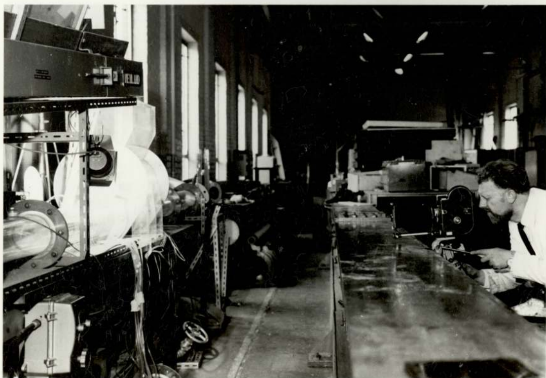
FIG 31 TEST RECORDING USING HIGH SPEED CAMERA
