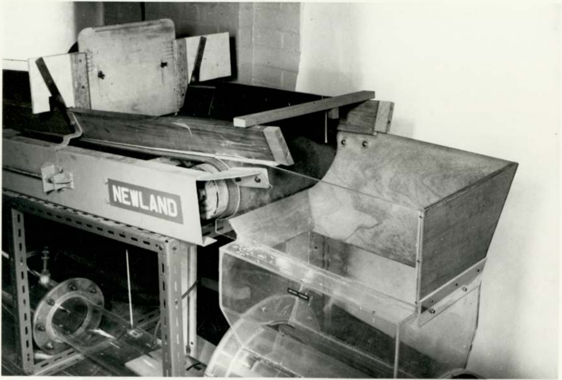
FIG 32 BELT FEED CONVEYOR TO STOWER
