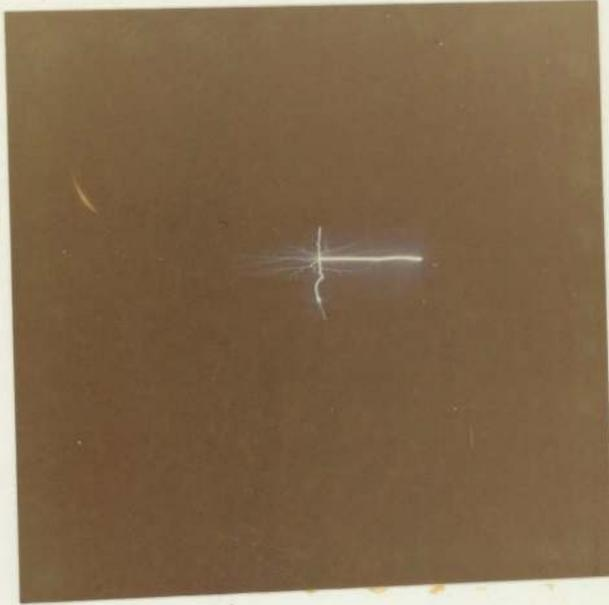
Fig. 2.49 A single-frame, time integrated photograph of secondary positive streamer in air at N. T. P.
