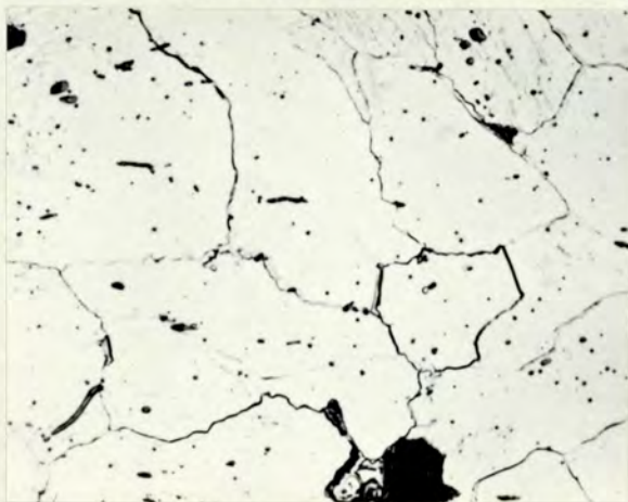
Fig. 3.34. Structures from outside (I), mid-radius (II) and axis (III) of specimens made from steel 1 and deformed at 600°C with 75 rev/min x 300. a - after 4 rev.; b - after 13 rev.
