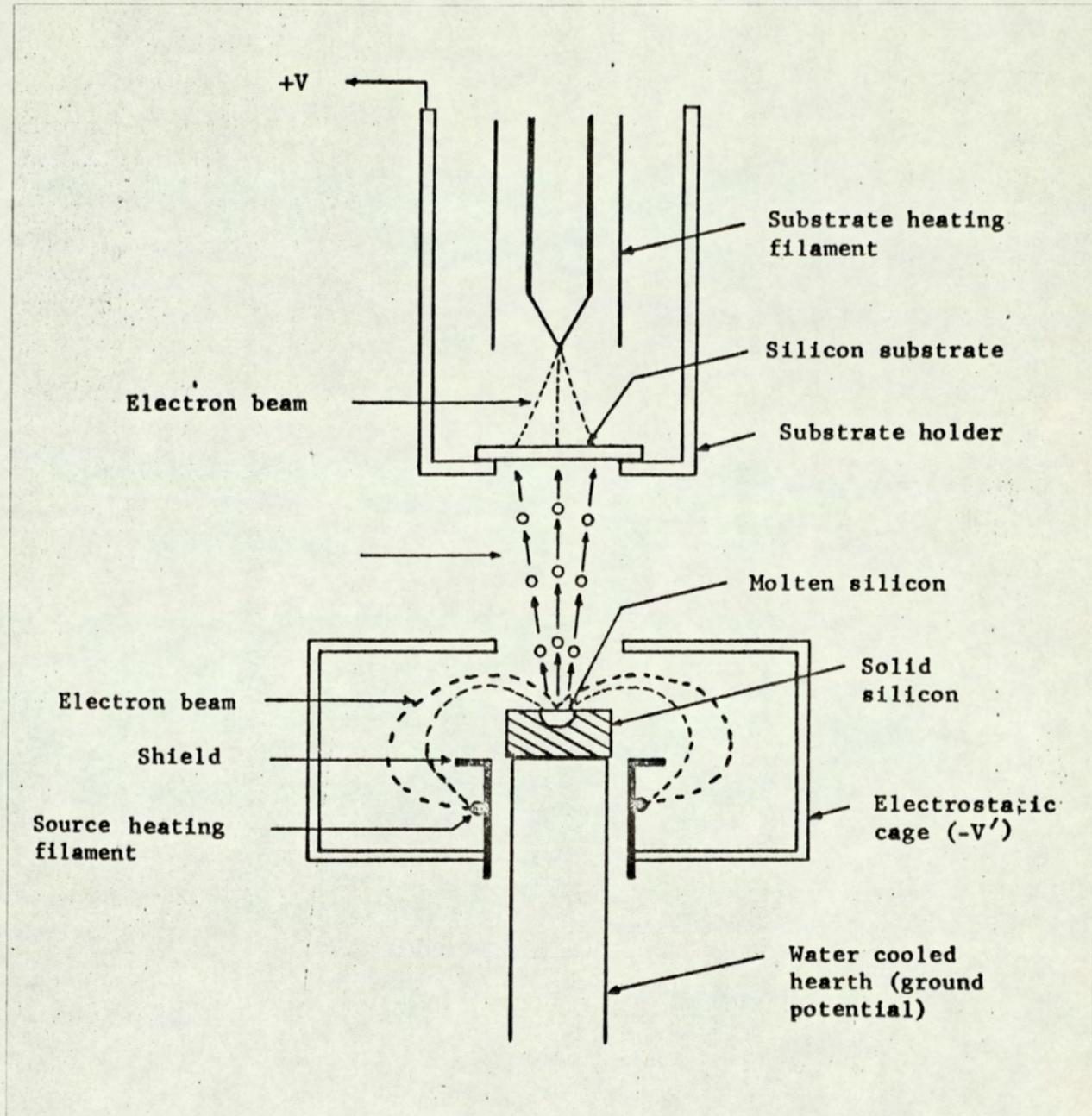
Fig. 2.6 Evaporation and substrate heating by electron bombardment. Ref. 22
