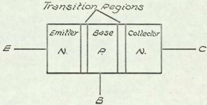
FIG. 1.4 AN IDEALISED STRUCTURE OF A TRANSISTOR.
