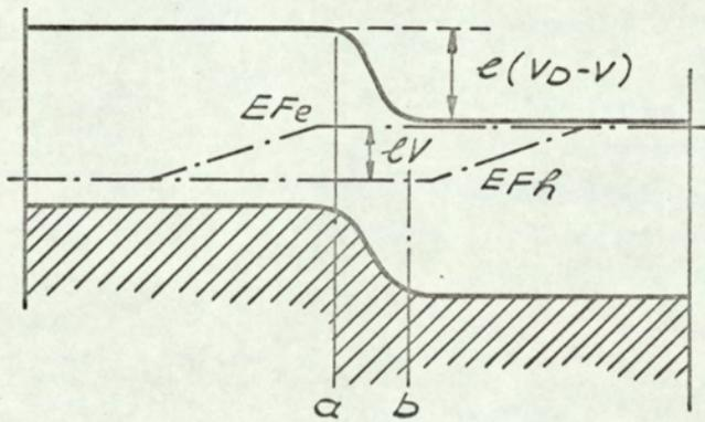
FIG. 4.14. FORWARD FLOW OF CURRENT IN A PN JUNCTION AT LOW INJECTION LEVEL.
