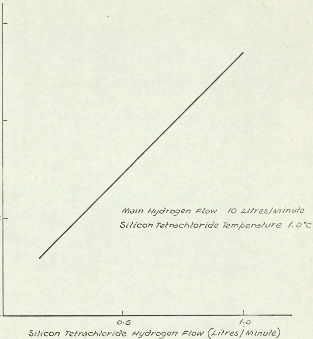
FIG. 5.11 INFLUENCE OF SILICON TETRACHLORIDE - HYDROGEN FLOW ON THE GROWTH RATE IN THE MULTIDEPOSITION APPARATUS.
