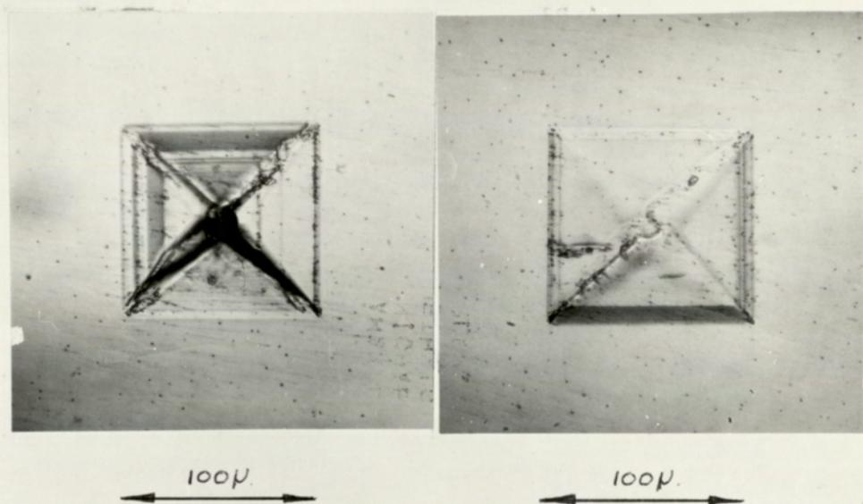
Fig. 6.2 Surface protruding imperfections on (100) orientated substrates
