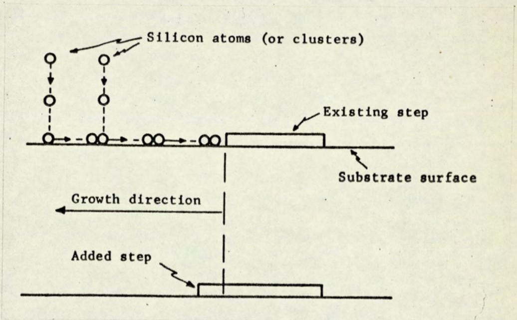
Fig. 2.1 Progress of a step during epitaxial growth
