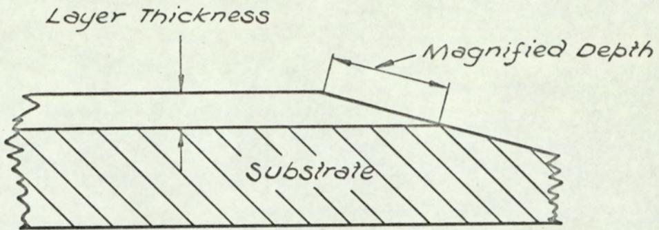
FIG.4.2. SECTION OF BEVELLED SILICON SUBSTRATE.
