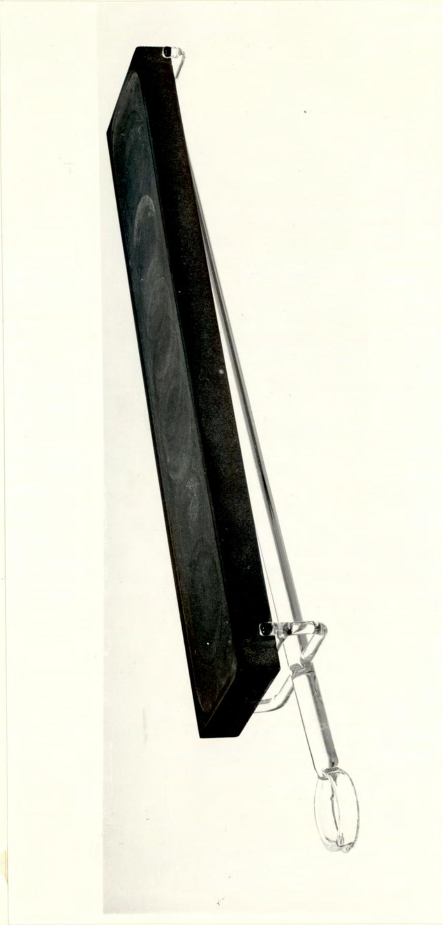
Fig. 3.15 Graphite coated silicon carbide susceptor for the multideposition apparatus
