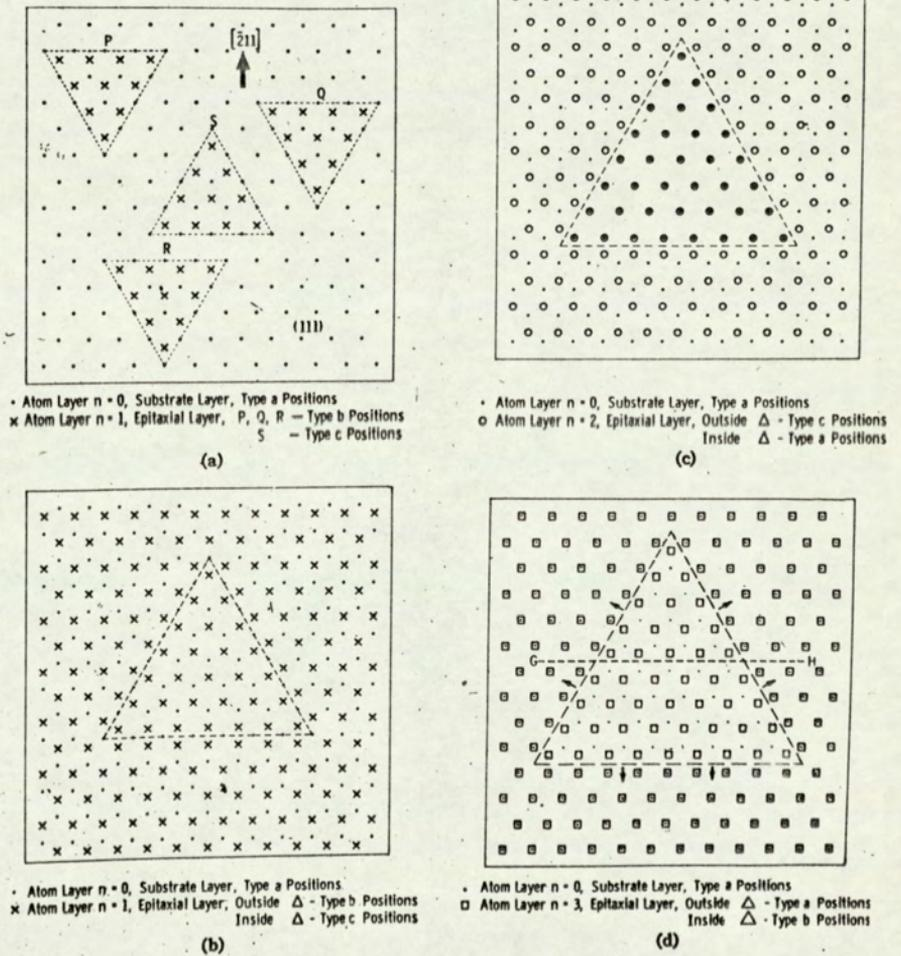
Fig. 7.3 Schematic diagrams showing successive stages in the formation of a triangle defect
