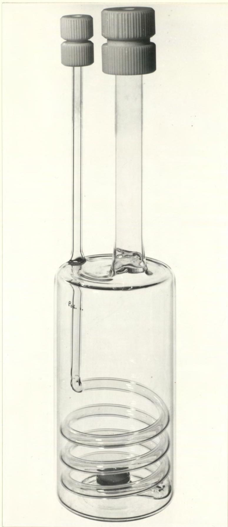
Fig. 3.12 Quartz evaporator and P.T.F.E. couplings used in the multideposition apparatus
