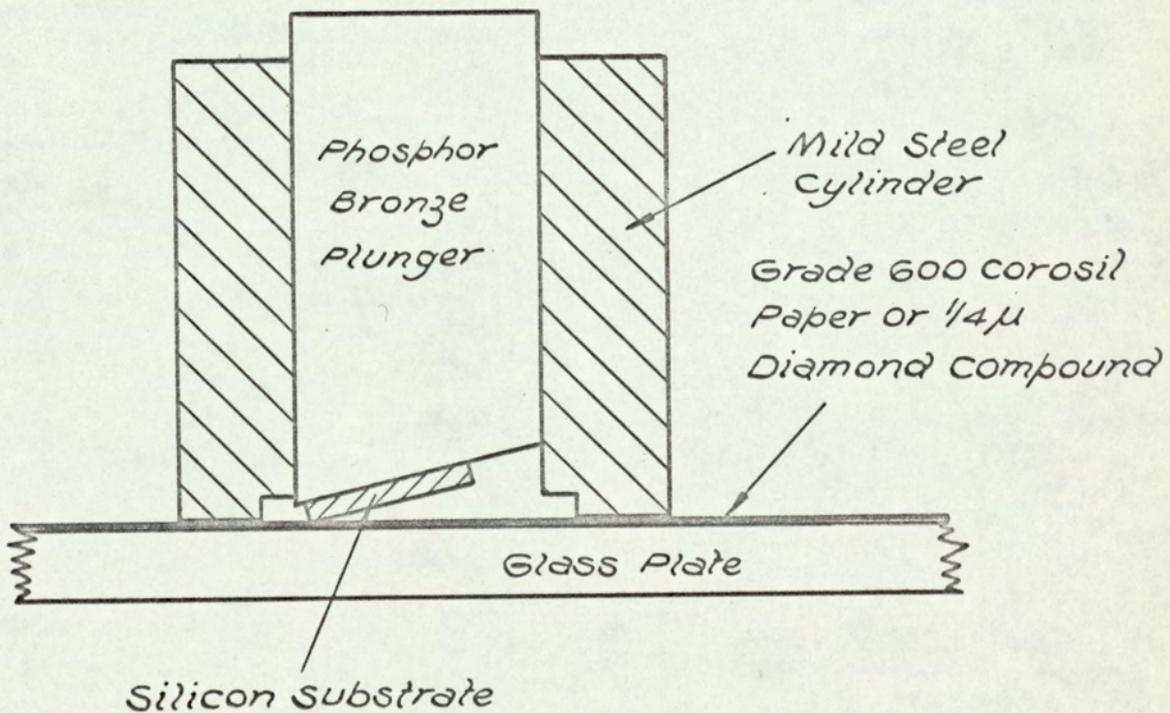
FIG.4.3 GRINDING JIG ASSEMBLY.
