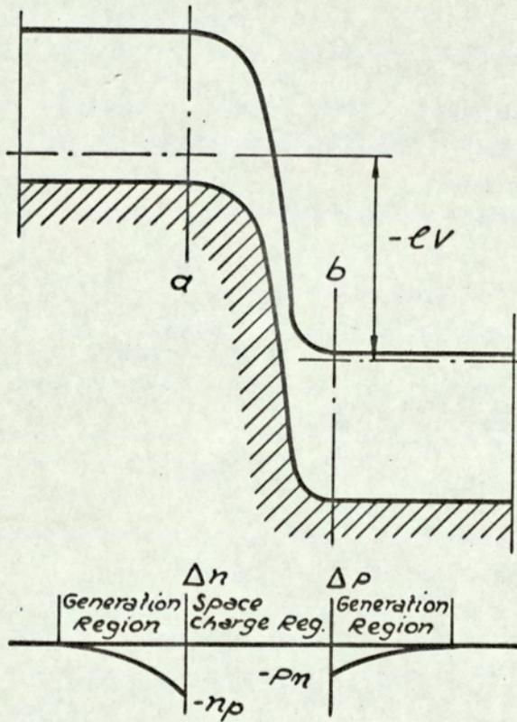
FIG. 4.15. PN JUNCTION WITH A REVERSE APPLIED BIAS.
