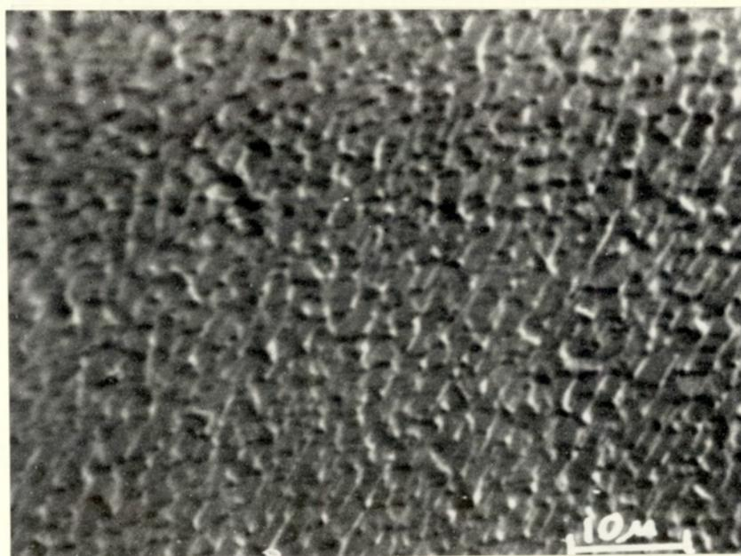
Fig. 2.2 Steps on a layer prepared by sublimation (x500)
