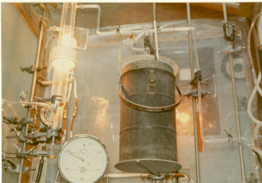
Fig. 3.2 Initial deposition apparatus
