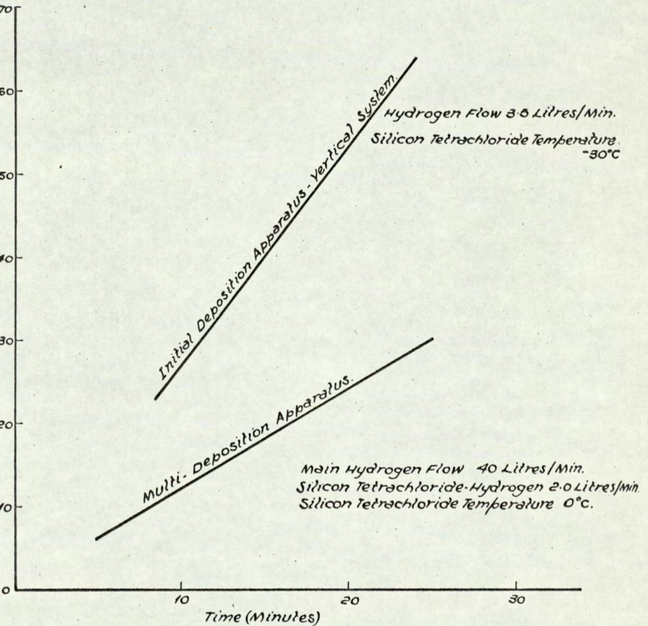
G. 5.13. LAYER THICKNESS AS A FUNCTION OF DEPOSITION TIME.
