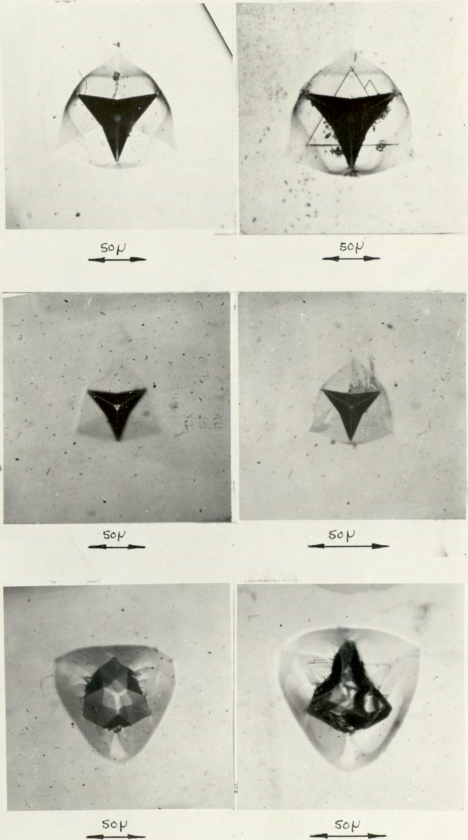
Fig. 6.1 Surface protruding imperfections on (111) orientated substrates
