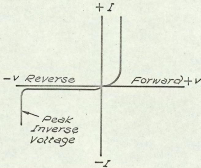
FIG. 1.3. TYPICAL RECTIFIER CHARACTERISTIC.
