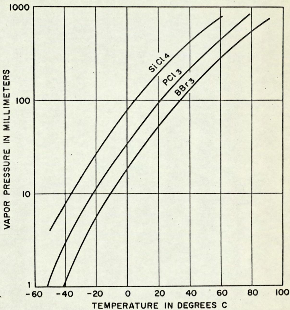
Fig. 5.24 Vapour pressure curves for  $\text{SiCl}_4$ ;  $\text{PCl}_3$  and  $\text{BBr}_3$ .
