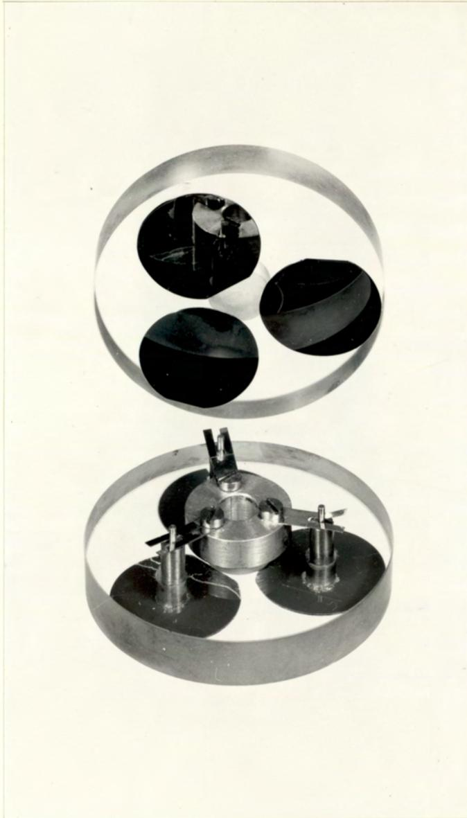
Fig. 3.18 Quartz discs used to support silicon substrates for electropolishing.
