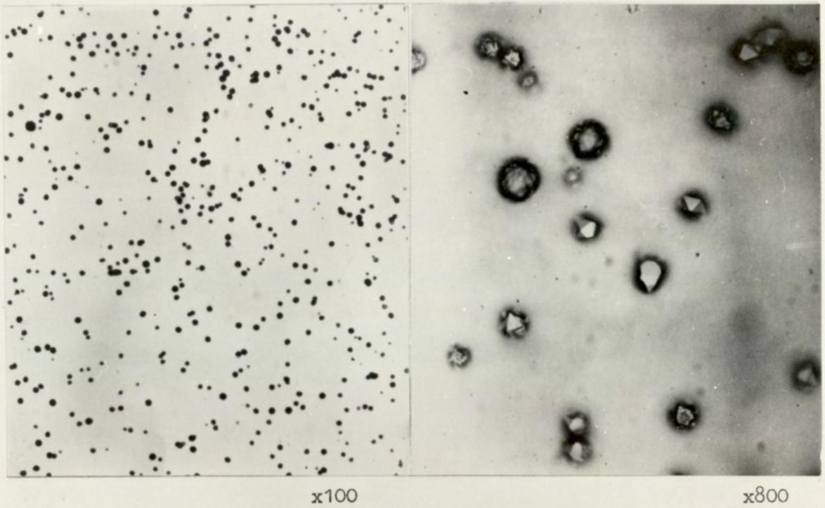
Fig. 5.1 Mechanically polished substrate surface after deposition at  $1000^{\circ}\text{C}$
