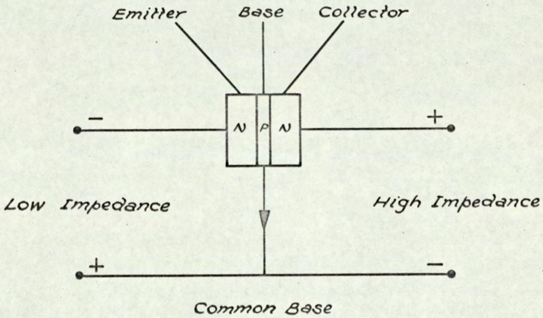
FIG. 4.20. FUNCTIONAL TRANSISTOR.
