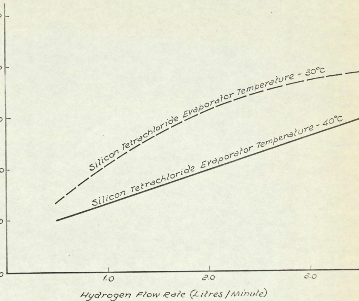
G.5.9. EFFECT OF HYDROGEN FLOW RATE ON THE LAYER GROWTH RATE IN THE INITIAL DEPOSITION APPARATUS.
