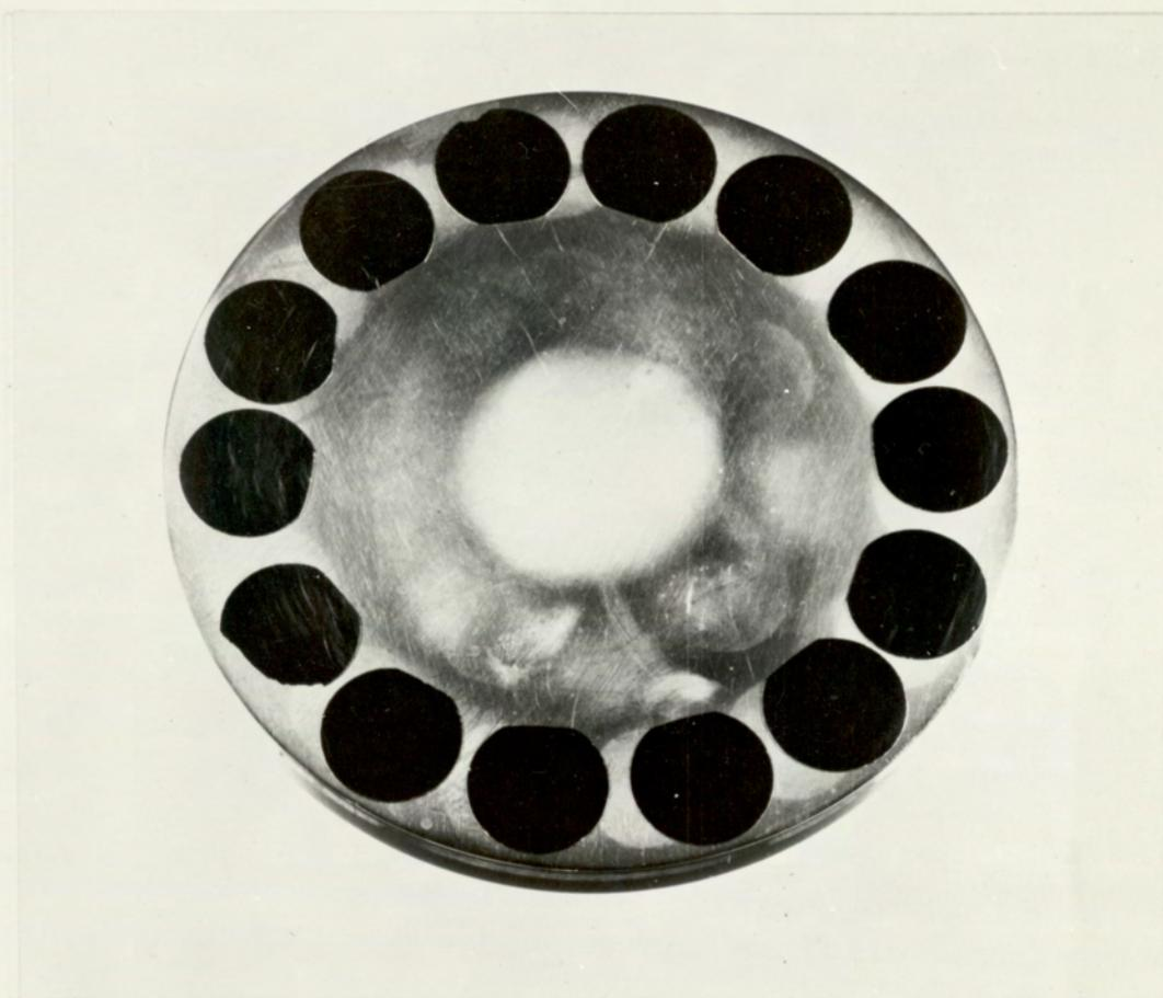
Fig. 3.16 Polishing plate with silicon substrates
