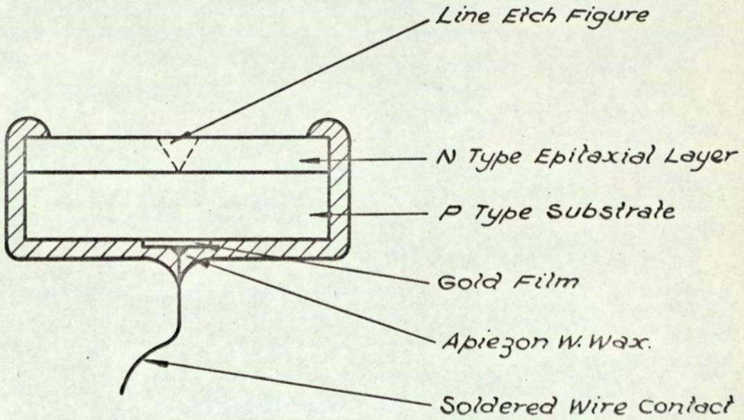
FIG. 4.17. EPITAXIAL SUBSTRATE PREPARED FOR
