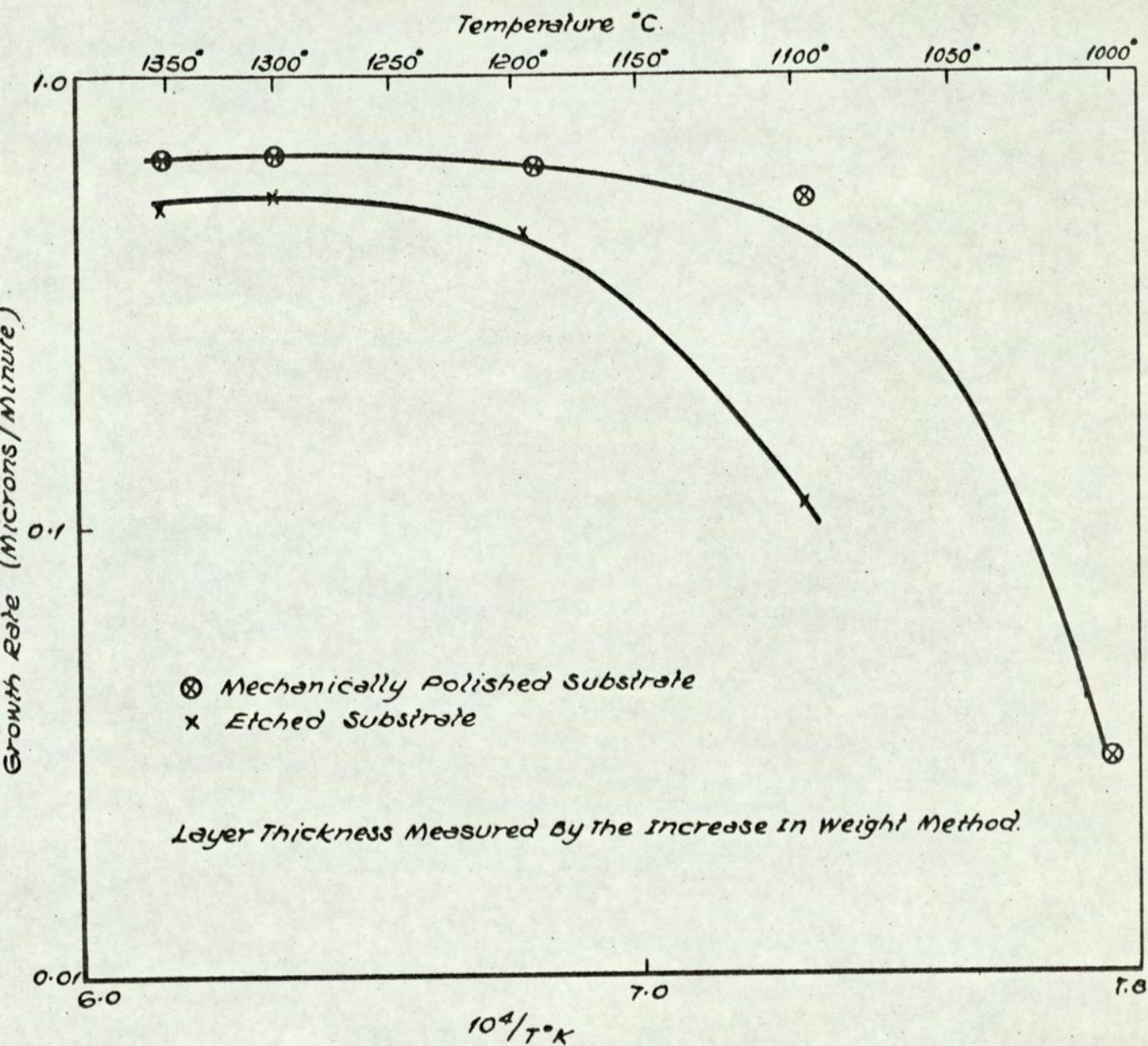
FIG 5.7 GROWTH RATE AS A FUNCTION OF TEMPERATURE.
