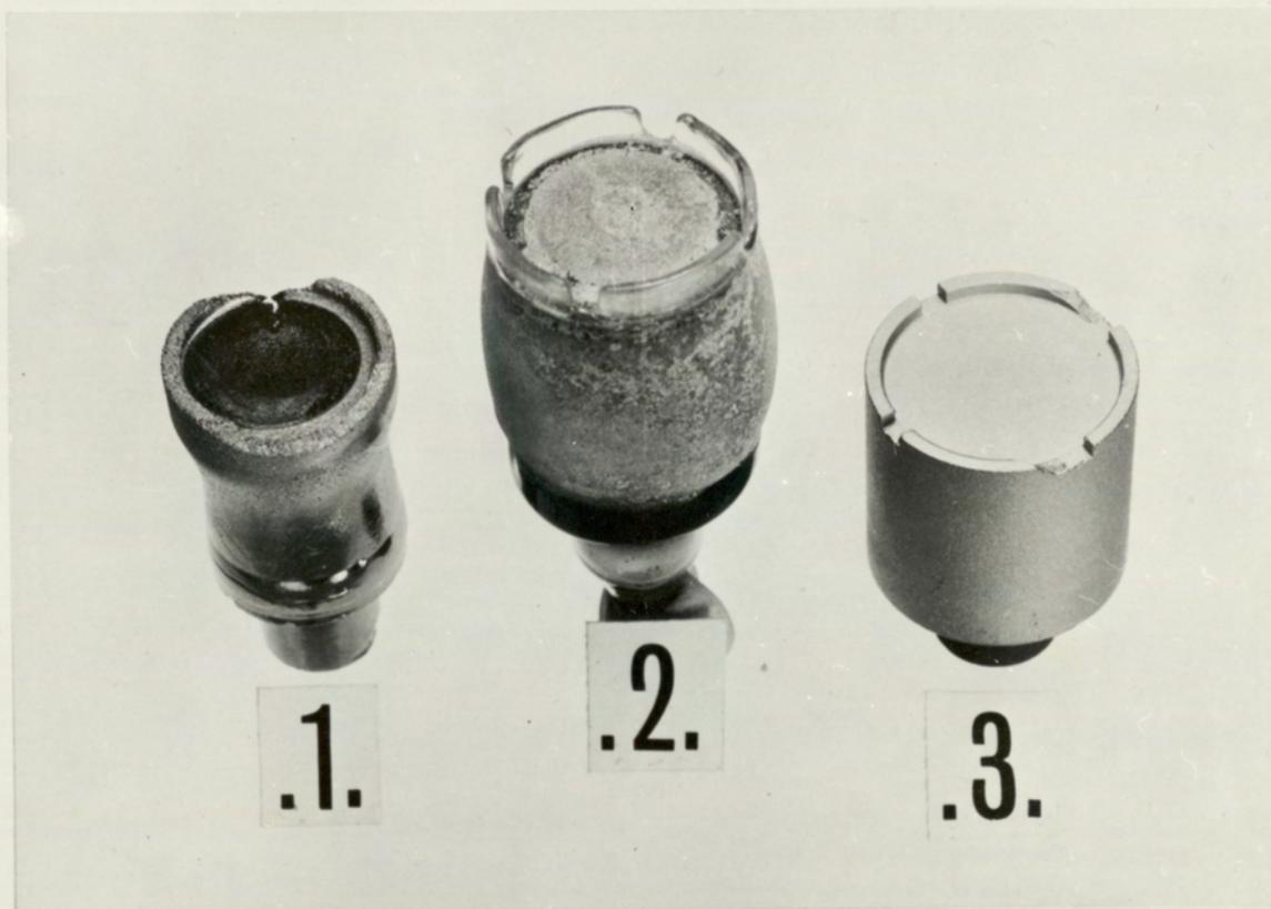
Fig. 3.13 Susceptors for the initial deposition apparatus -
