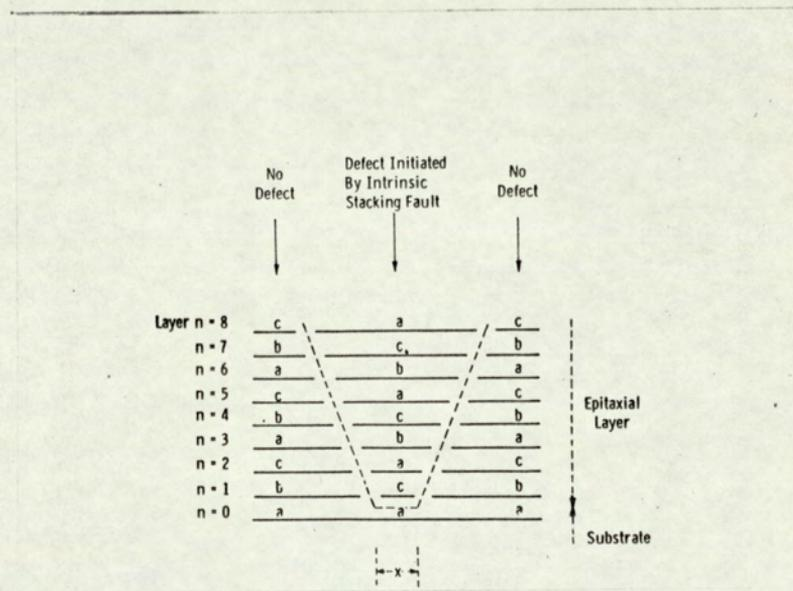
Fig. 7.4 Cross section through the defect of Fig. 7.3(d) corresponding to the line GH. The defect is initiated by a stacking fault on the (111) plane parallel to the substrate, and then propagates as stacking faults on the three inclined  $\{111\}$  planes. The defect has the form of a regular tetrahedron.
