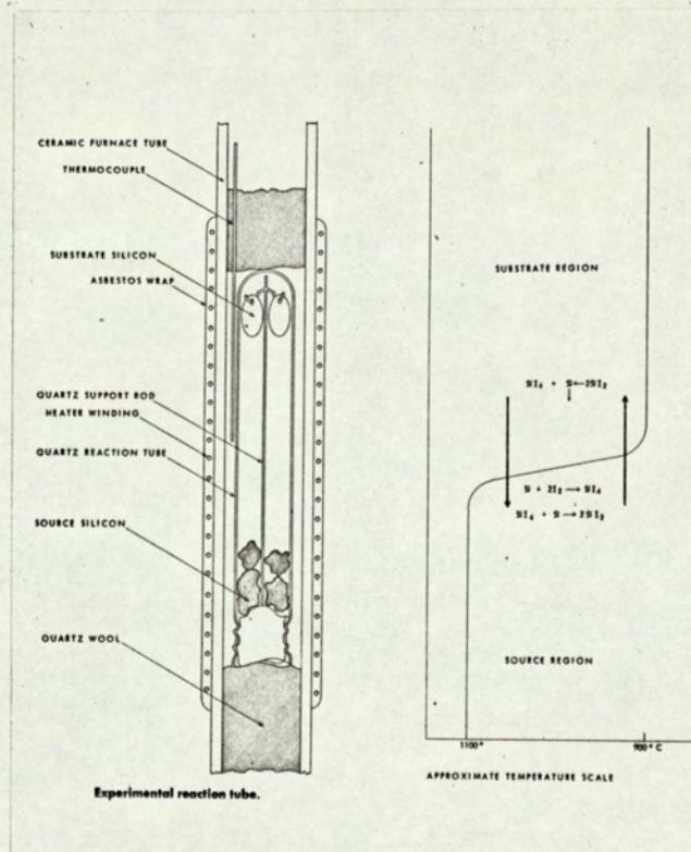
Fig. 2.5 Experimental reaction system. Ref. 4
