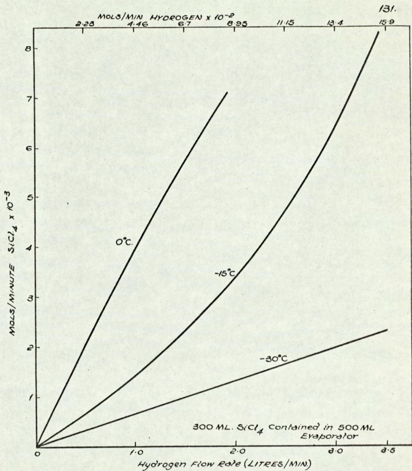
FIG. 58. EFFECT OF HYDROGEN FLOW RATE ON THE CONCENTRATION OF  $\text{SiCl}_4$  IN THE GAS STREAM OF THE INITIAL DEPOSITION APPARATUS.
