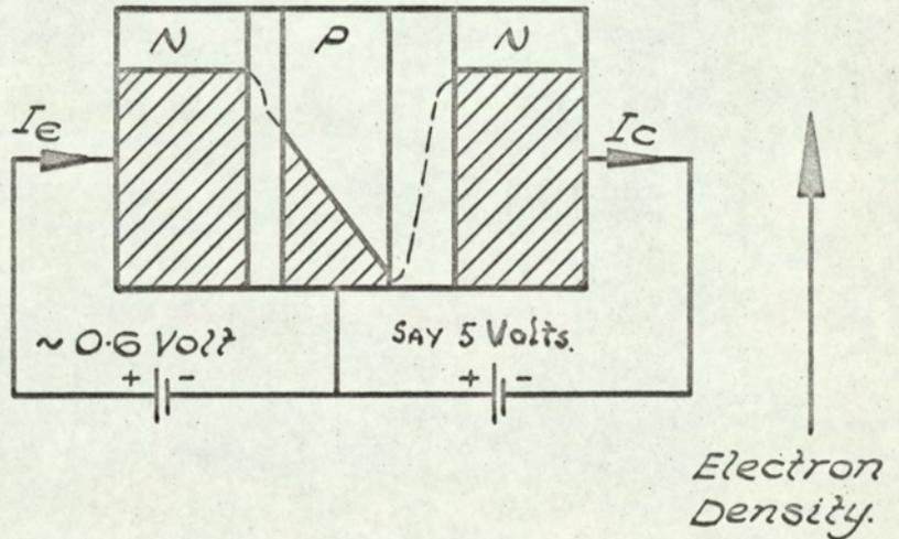
FIG. 1.5. ELECTRON DENSITY DISTRIBUTION IN AN N.P.N. TRANSISTOR.
