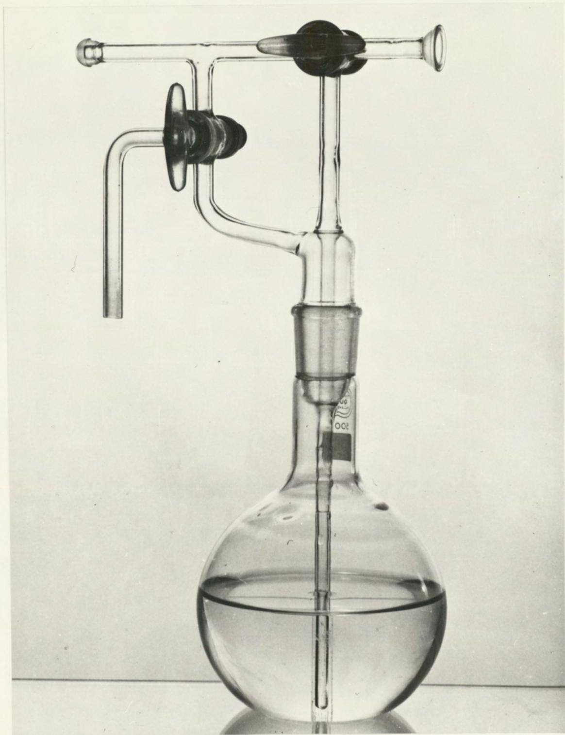
Fig. 3.3 Silicon tetrachloride evaporator for the initial deposition apparatus
