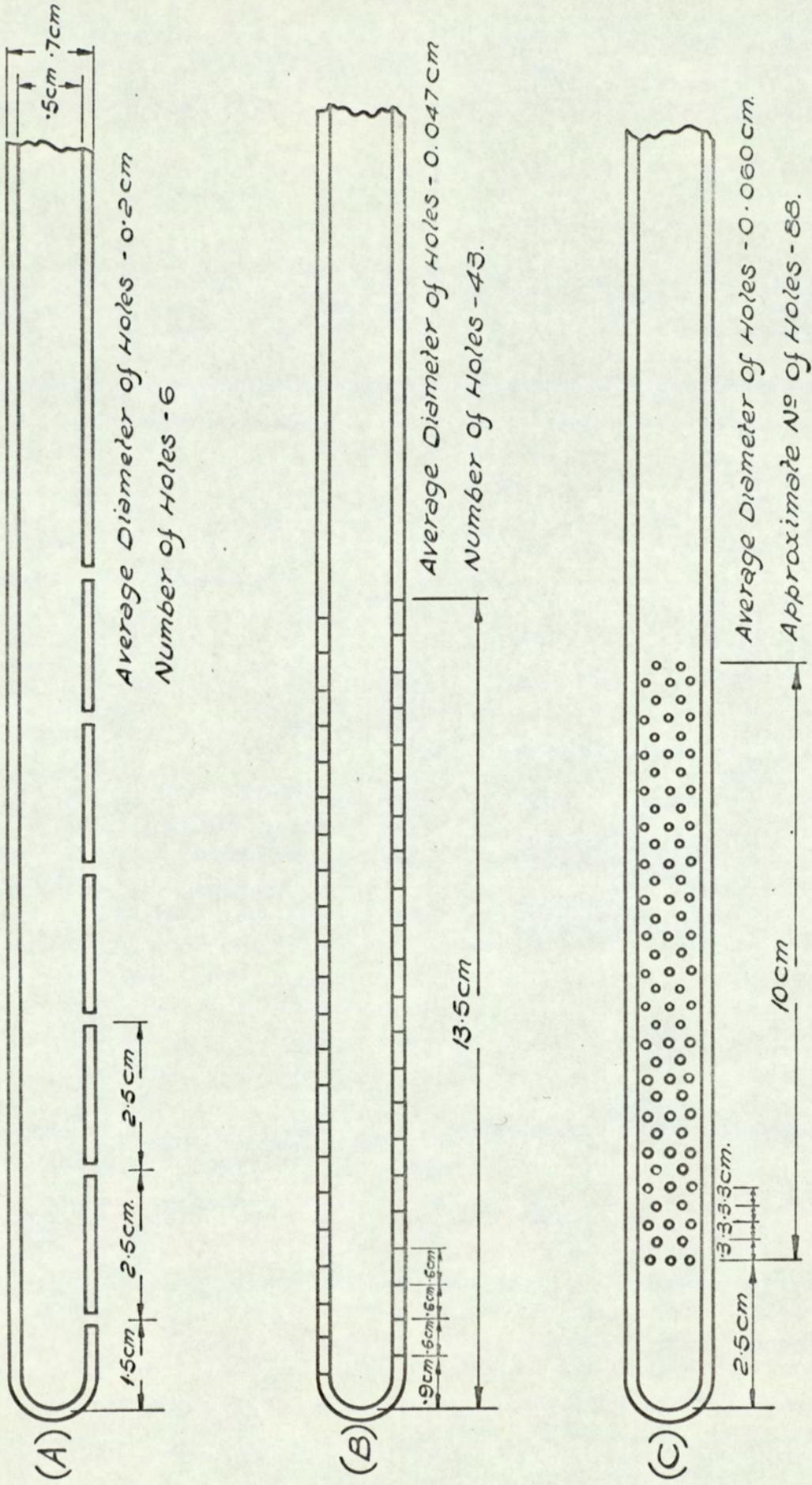
FIG. 3.7. QUARTZ INLET TUBES FOR VERTICAL GAS FLOW IN HORIZONTAL REACTION TUBE.
