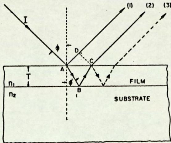
Ray diagram for reflection from a film deposited on a thick substrate. The amplitudes of rays 1, 2, 3, etc., add vectorially resulting in maxima and minima in the reflectance spectrum.
