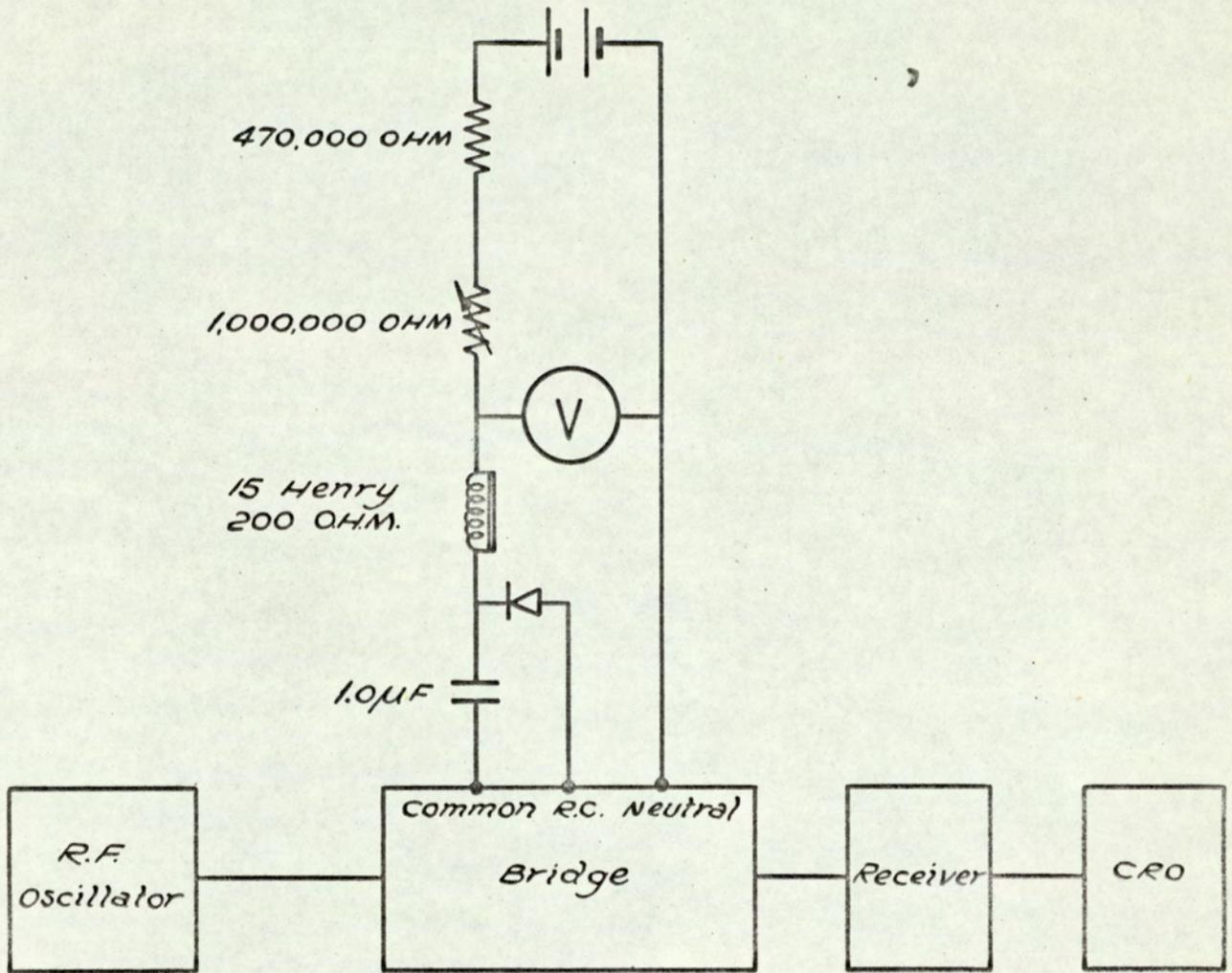
FIG 4.16 CIRCUIT FOR JUNCTION CAPACITANCE MEASUREMENTS.
