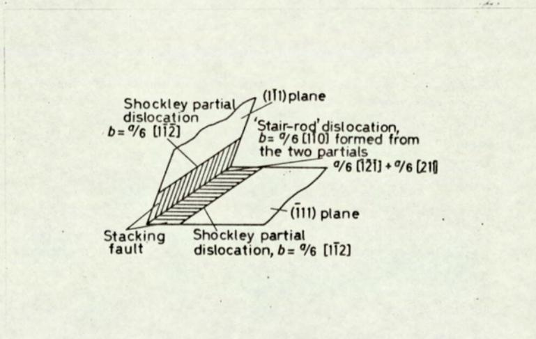
Fig. 7.2 Formation of a stair rod dislocation
