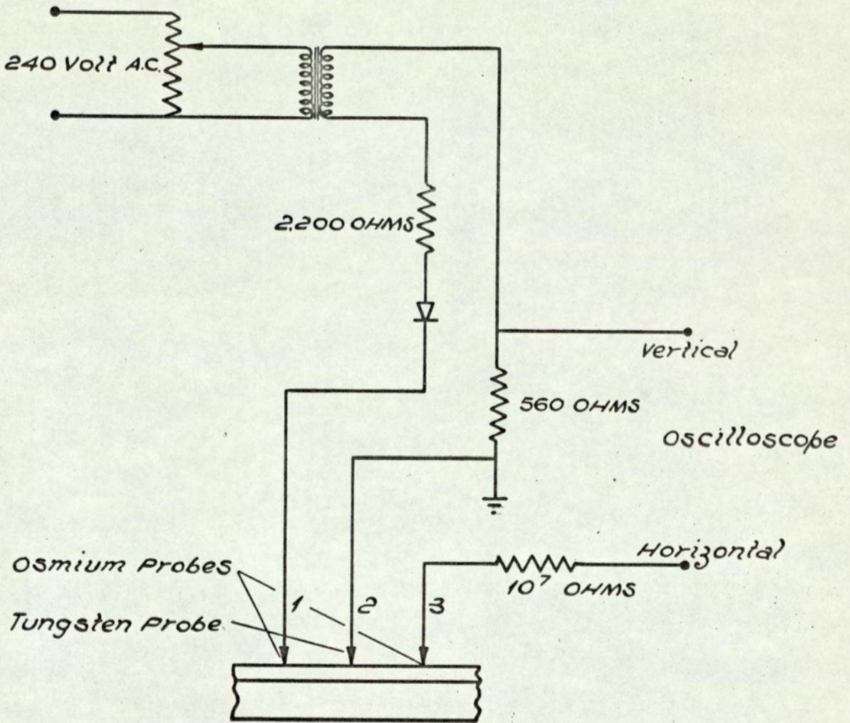
FIG. 4.10. CIRCUIT FOR THREE POINT PROBE MEASUREMENTS.
