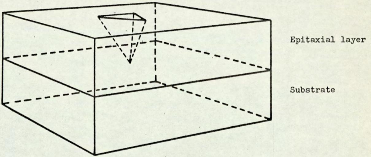
Fig. 4.7 Stacking fault formation on (111) substrate
