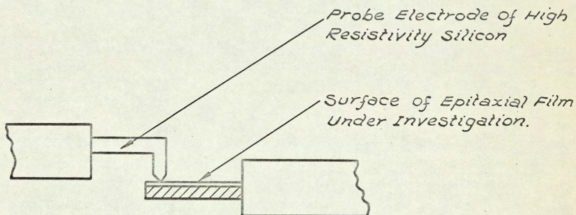
FIG. 4. 19. MASS SPECTROMETER ELECTRODE ARRANGEMENT.
