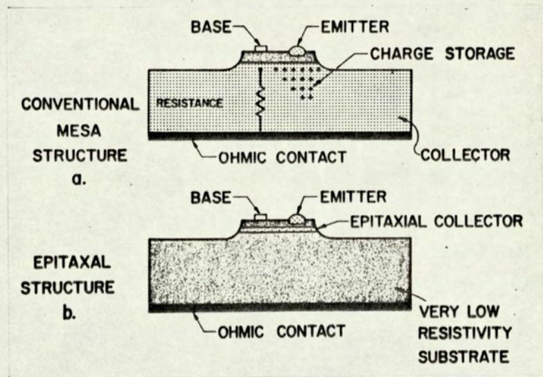
Fig. 1.8 Conventional and epitaxial diffused mesa transistors
