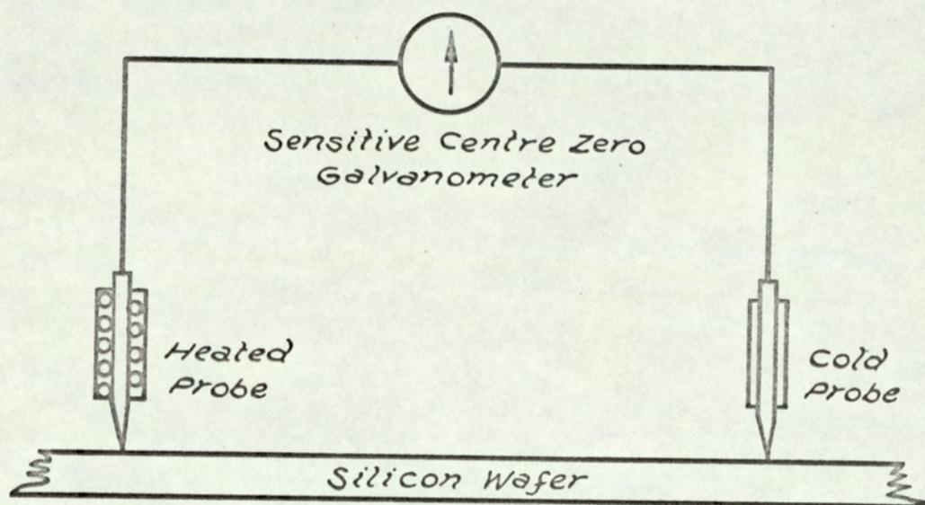
6 4.1 SCHEMATIC DIAGRAM OF THERMO-ELECTRIC PROBE.
