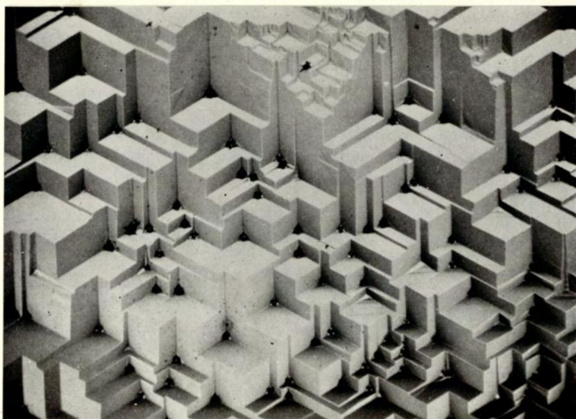
Fig. 2.4 Surface of layer prepared from  $\text{SiHCl}_3$  at low temperature. (x28) Ref. 8
