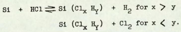
With this process the substrate surface free of mechanical damage and oxide is produced in situ immediately prior to the epitaxial deposition. The rate of removal of the silicon from the substrate can be accurately controlled by the gas concentration and polishing time and unlike the electropolishing method is not a function of the resistivity or conductivity type of the silicon (49).
