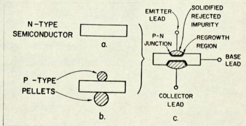
Fig. 1.7 Alloyed PN junction
