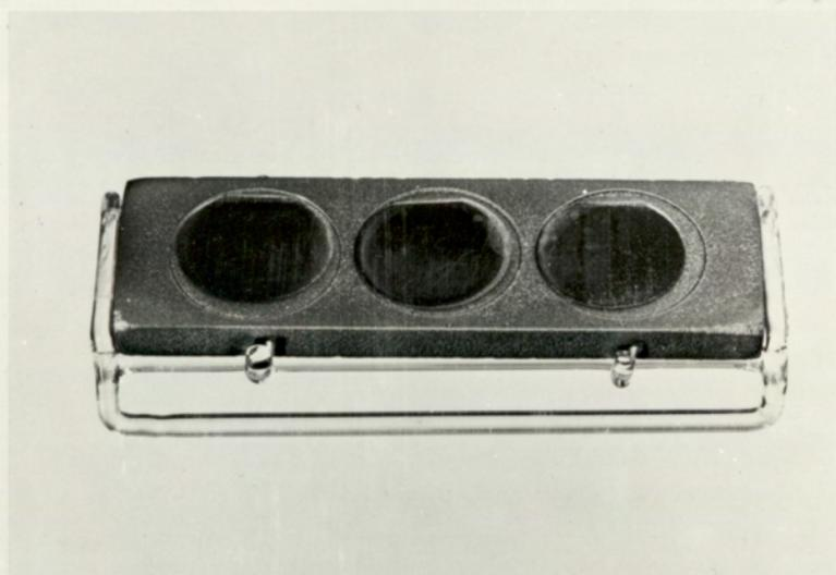
Fig. 3.14 Susceptor for the initial deposition apparatus - horizontal system
