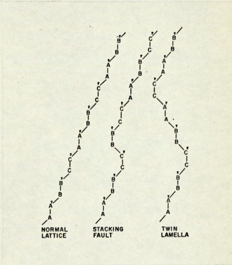
Fig. 7.1 Defects in the diamond lattice
