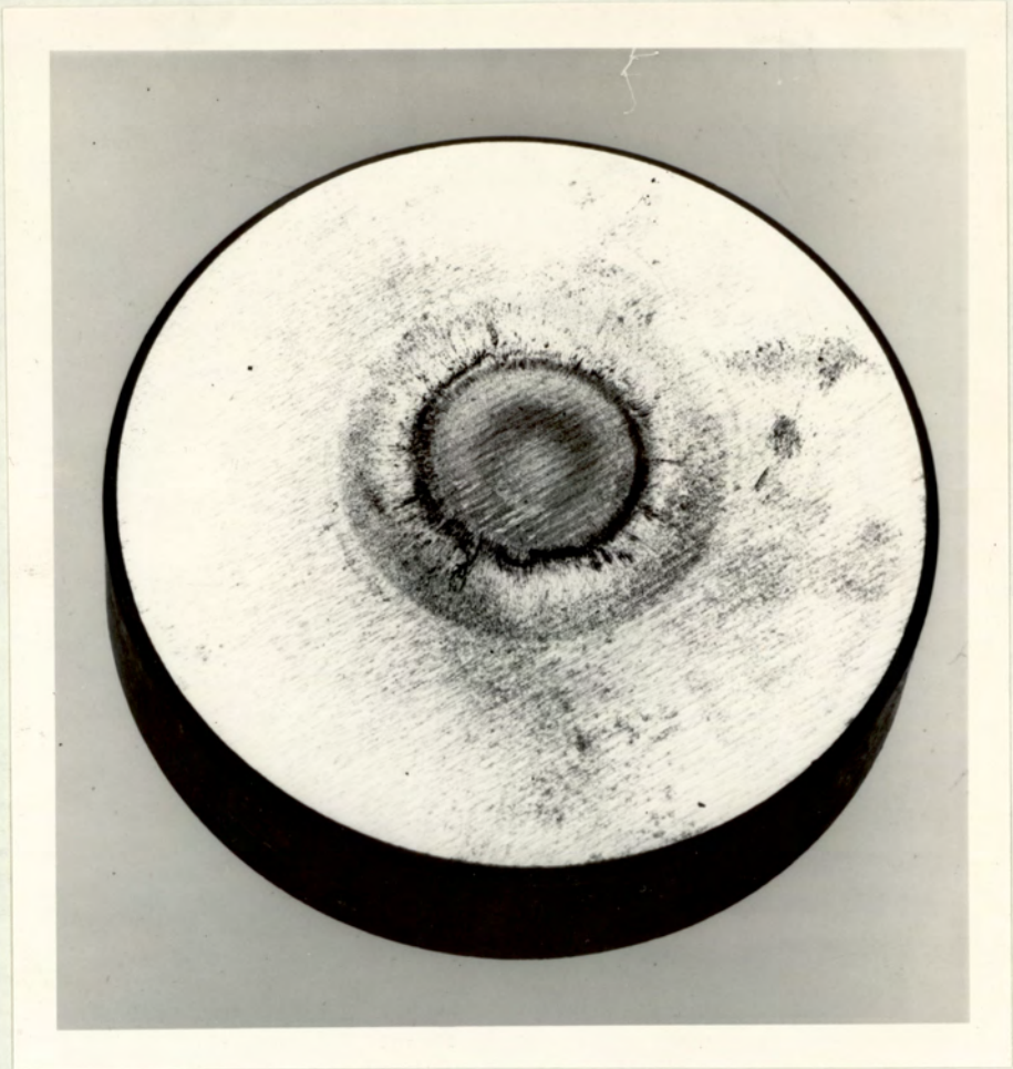
Fig. 25. Photograph of a die showing the wear pattern at the centre. X 2.
