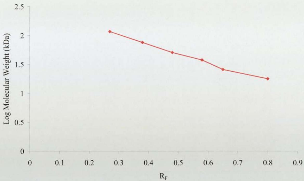
The  $R_F$  value in relation to the molecular weight of standard molecular weight markers.
