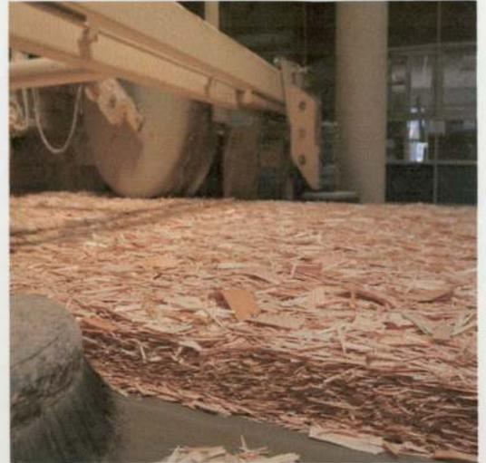
Figure 12: OSB during production stage [19]
