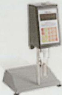
Figure 68: Brookfield rheometer
