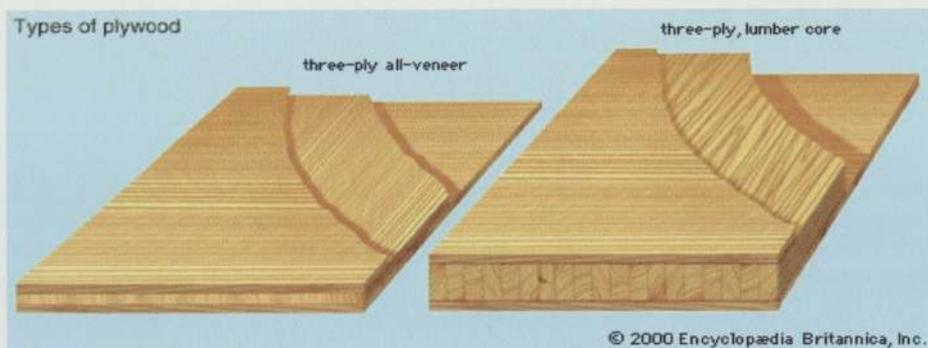
Figure 19: Types of plywood
