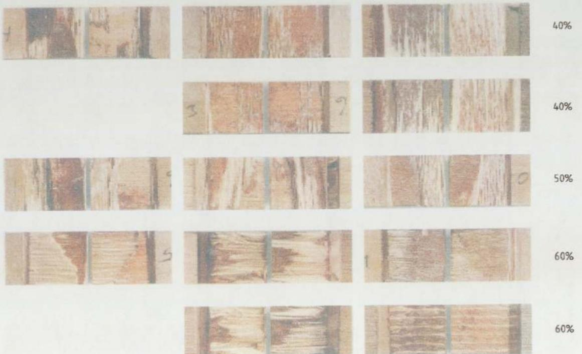
Figure 103: Wood fibre failure 40-60% reference illustrations by EN 413.1 standard
