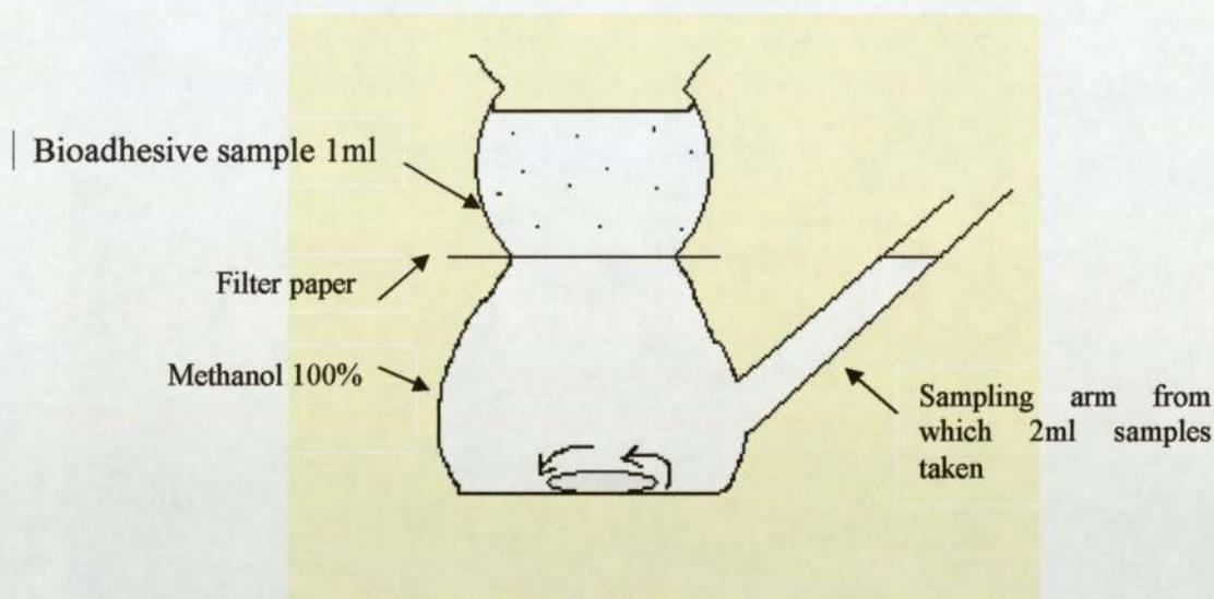
*Figure 2.2: The release model apparatus*
