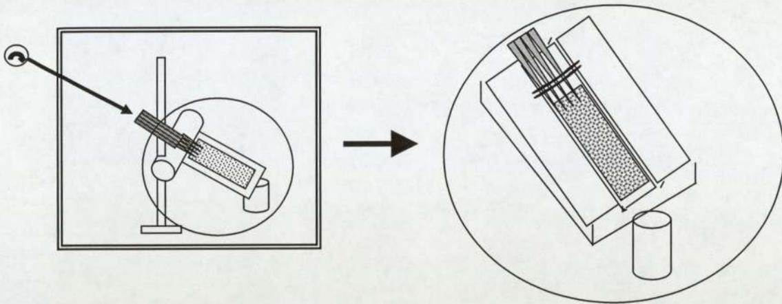
***Figure 2.6: Retention model apparatus***
