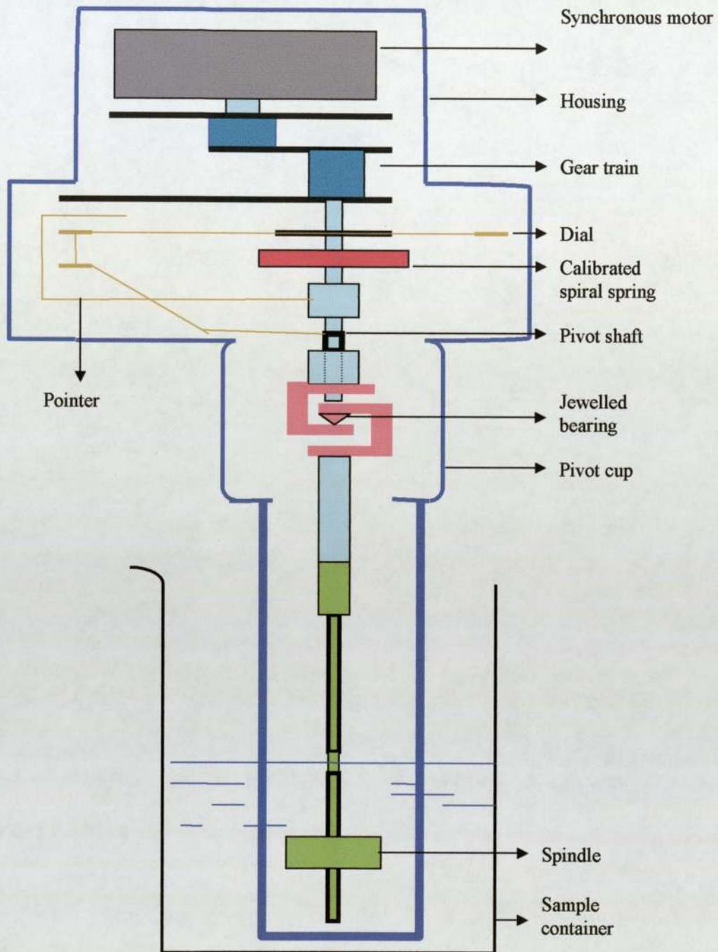
Figure 2.1: Schematic view of the structure of Brookfield viscometer (from Tang, 2004).
