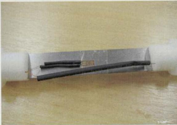
*Figure 2.6, Strain Gauge Position*
