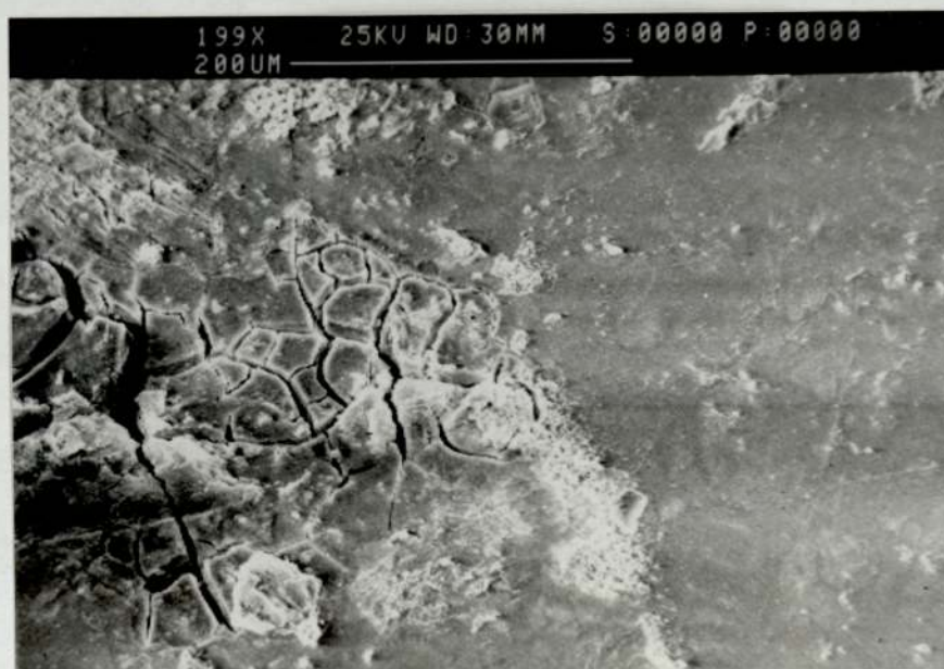
Figure 4.21 Zinc coated sample after being embedded in "salt" wood for ten weeks - localised cracking
