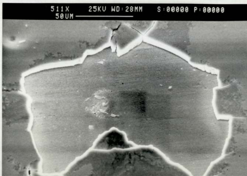
Figure 4.19 Zinc cobalt alloy coated sample after two weeks immersion in "salt" solution showing exfoliated area
