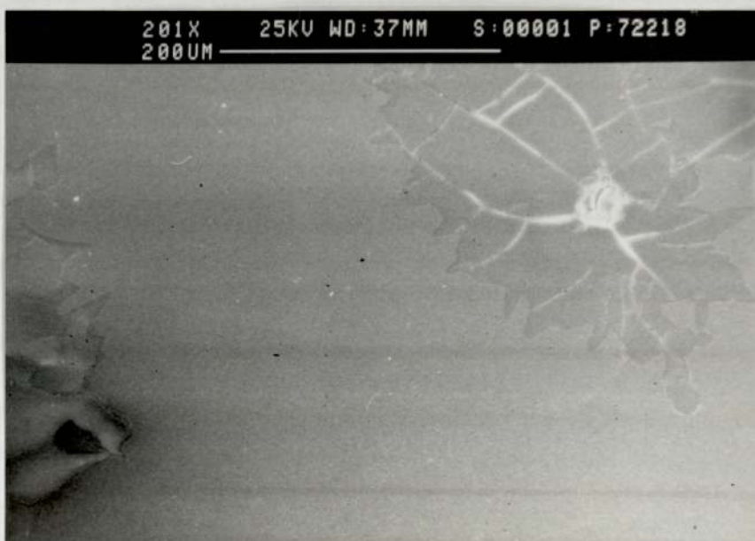
Figure 4.25 zinc coated steel with "full passivation" sample after being embedded in "oxide" wood for ten weeks
