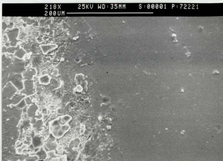
Figure 4.24 Zinc cobalt alloy coated sample after being embedded in "oxide" wood for ten weeks
