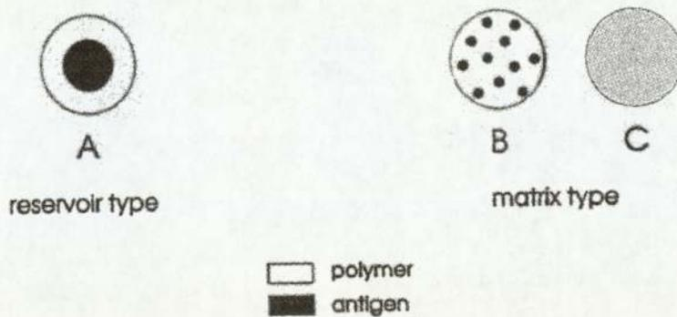
**Figure 1.5** Typical structures of microparticles
