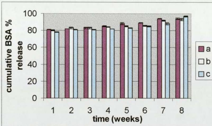
**Figure 5.15** Release of different initial Mw microspheres made of poly(CPB:SA 20:80) (n=3, mean $\pm$ s.d.).
