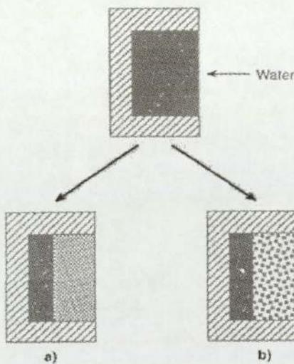
**Figure 1.2.** Illustration of water diffusion and degradation in degradable polymers:
