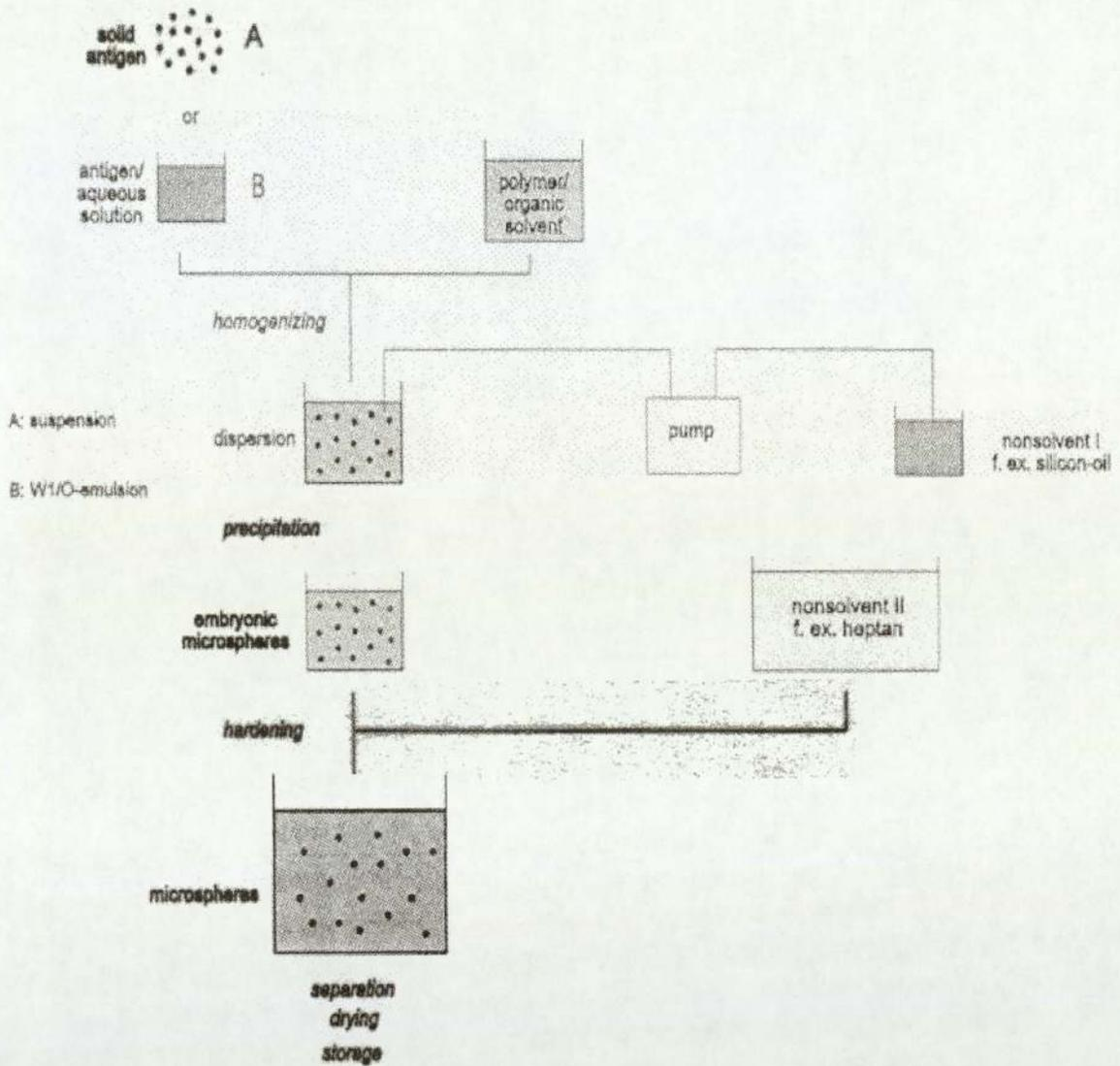
**Figure 1.9** Manufacturing of microspheres: solvent-removal technique
