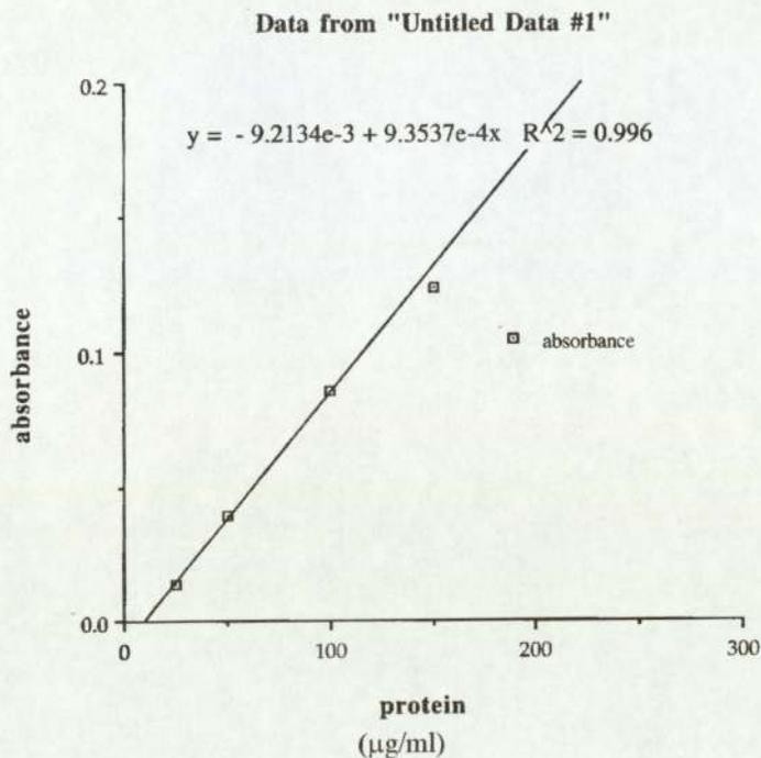
**Figure 5.6** Typical calibration curve for protein loading
