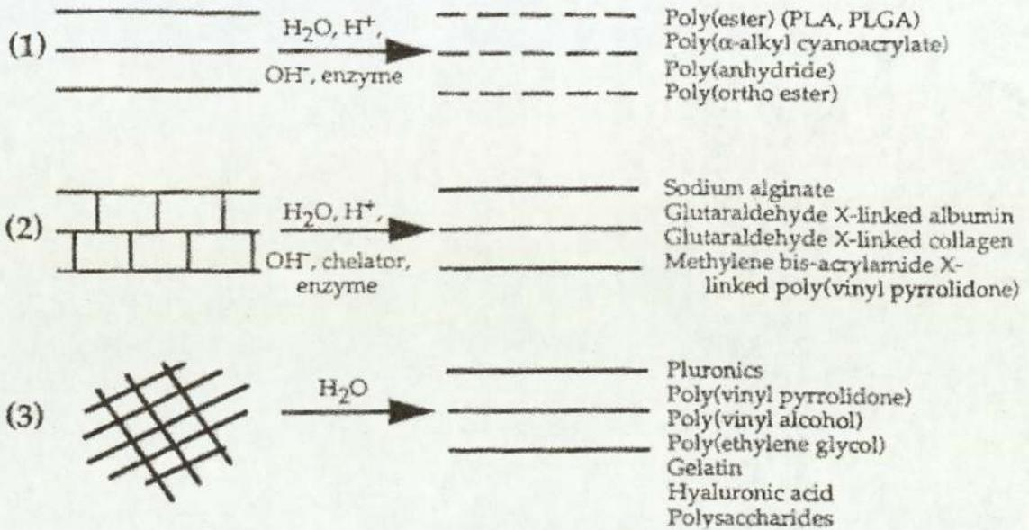
**Figure 1.1** Schematic representation of different polymer degradation mechanisms:
