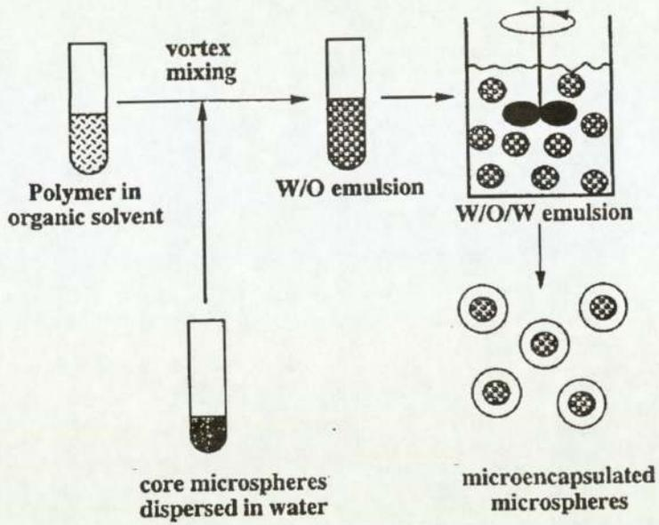
**Figure 1.11** Manufacturing of double-walled microspheres by a modified double-emulsion technique
