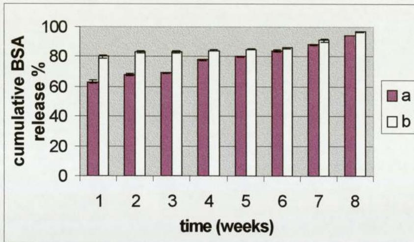
**Figure 5.13** Release of different initial BSA loaded microspheres made of poly(CPB:SA 20:80) (n=3, mean±s.d.).
