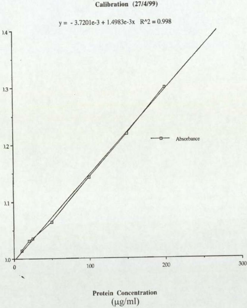
**Figure 5.12** Calibration curve for protein release
