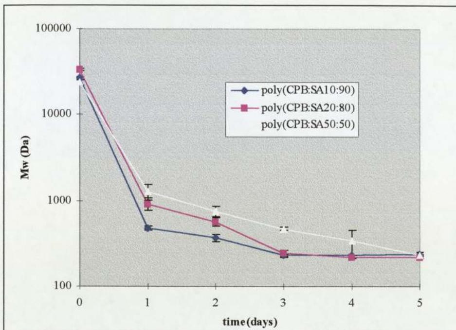
**Figure 5.1** GPC analysis of degradation of polymers in PBS (represented by Mw decrease) (n=3, mean±s.d.)
