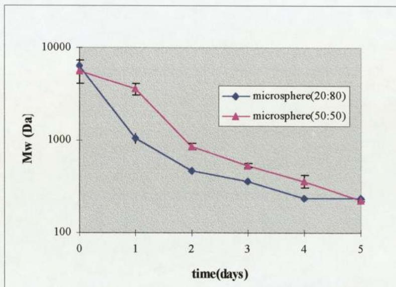
**Figure 5.9** GPC analysis of degradation of microspheres in PBS (represented by Mw decrease) (n=3, mean±s.d.)
