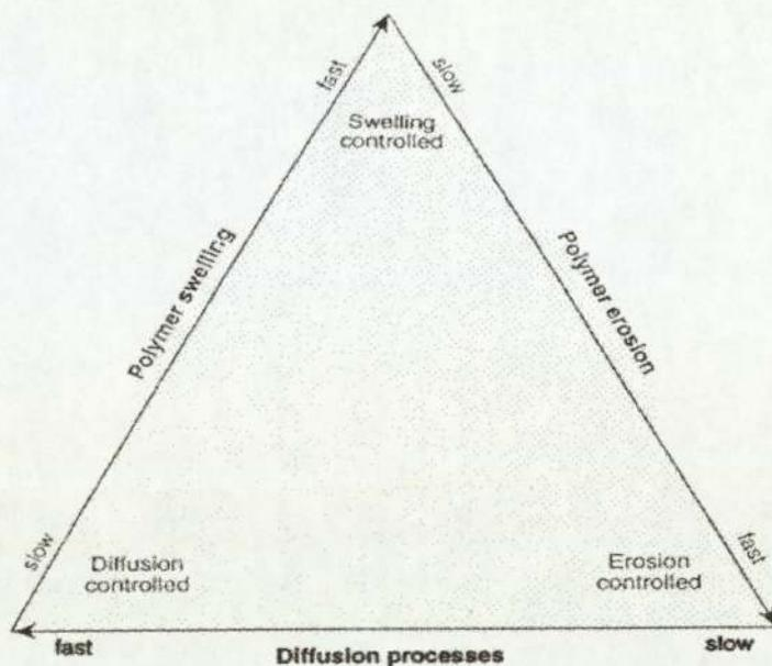
**Figure 1.4** Possible mechanisms of drug release from degradable polymers
