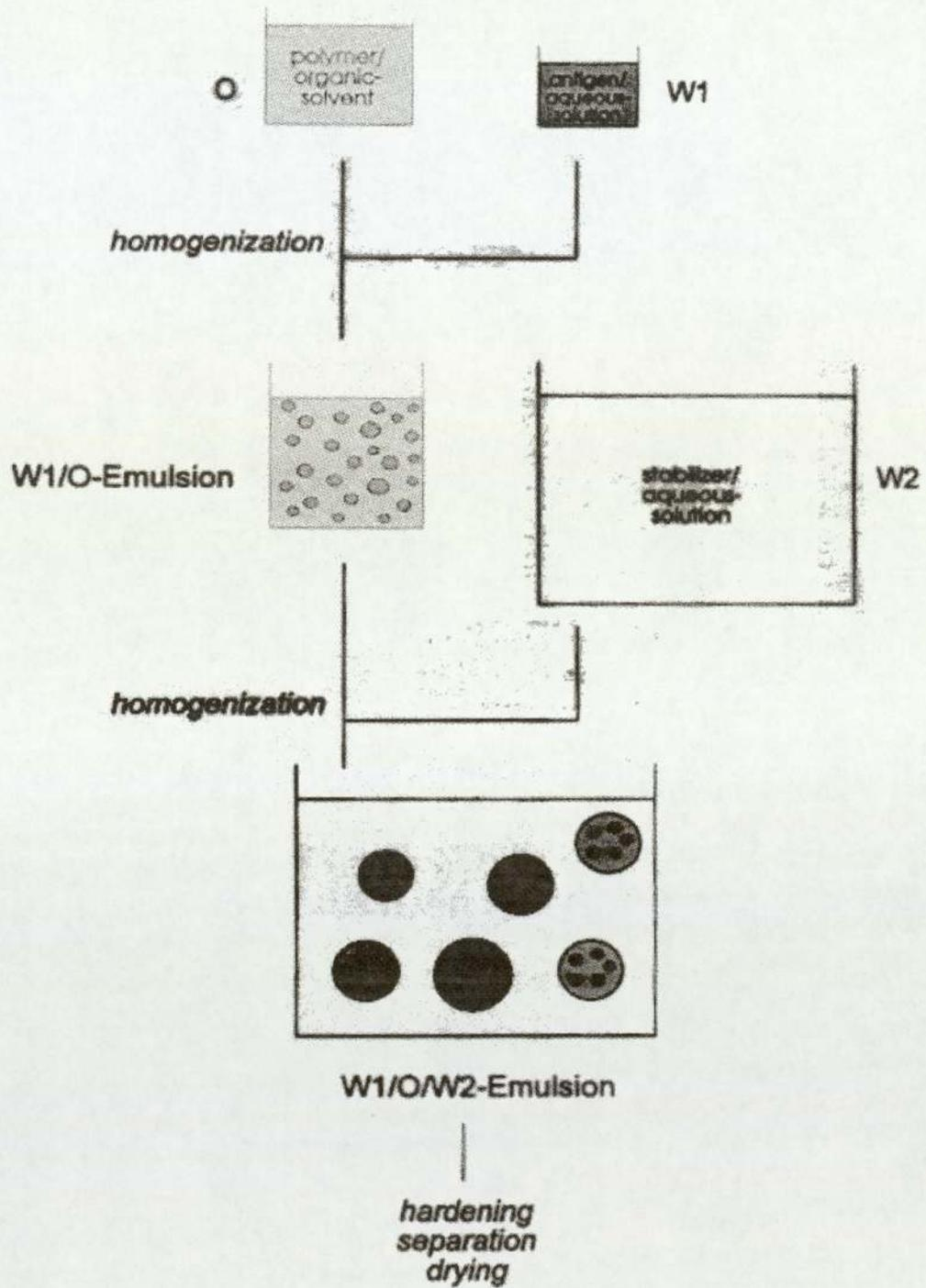
**Figure 1.8** Manufacturing of microspheres: W/O/W double-emulsion method
