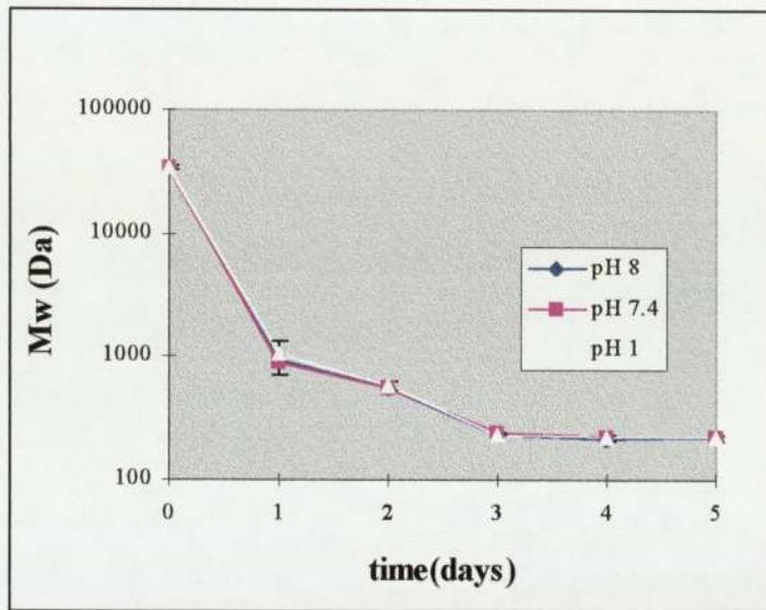
**Figure 5.2** Effect of buffer pH on poly(CPB:SA 20:80) degradation (n=3, mean±s.d.)
