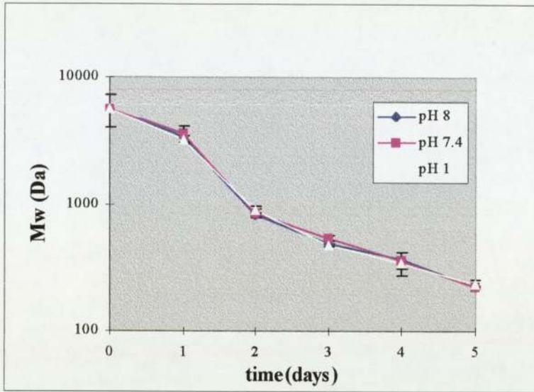
**Figure 5.10** Effect of buffer pH on microspheres (50:50) degradation (n=3, mean±s.d.)
