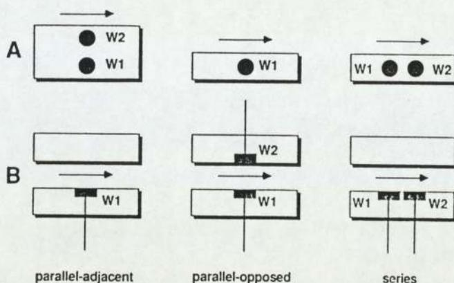
Figure 7. Dual-electrode configuration. (A) Front sight, and (B) side sight; W1,W2 working electrodes; ->, flow direction.
