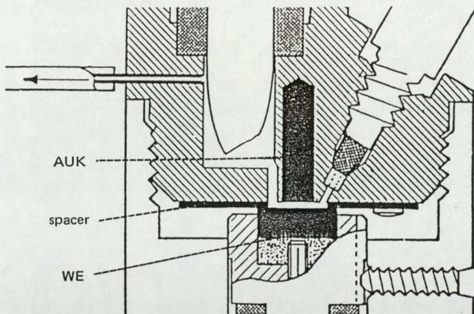
**Figure 6. Three electrode detection system.(65)**
