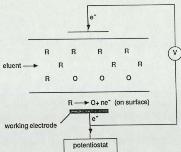
**Figure 5 . Amperometric detection principle (65)**
