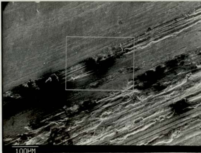
Photomicrograph 14: Surface of worn electro-deposited tin/cobalt, pin no. 46, showing the electrodeposit still intact and highlighting the generation of a wear particle, x 200 magnification.
