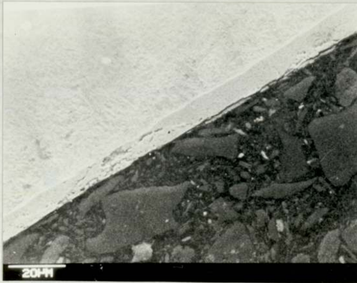
Photomicrograph 2: Transverse section of worn Electroless nickel/PTFE showing some delamination of the deposit. Pin No. 5 x 1000 magnification.
