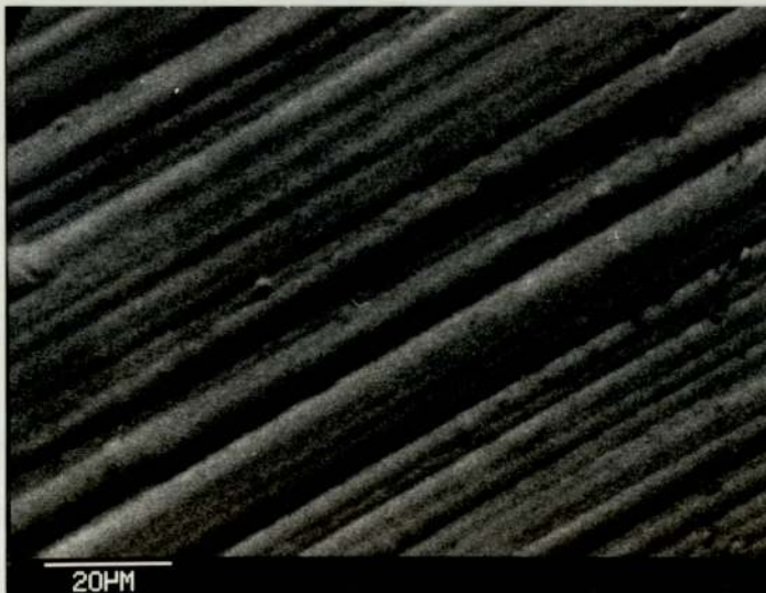
Photomicrograph 6: Surface of unworn Electroless nickel, pin no. 31, showing the electroless deposit following the grinding marks of the substrate, x 1000 magnification.
