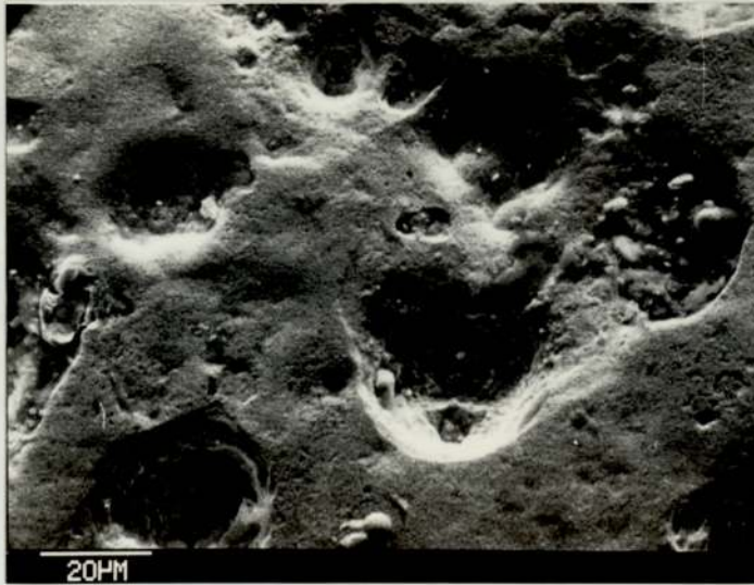
Photomicrograph 4: Surface of unworn Electroless nickel/PTFE Pin no. 53, showing some porosity in the coating, x 1000 magnification.
