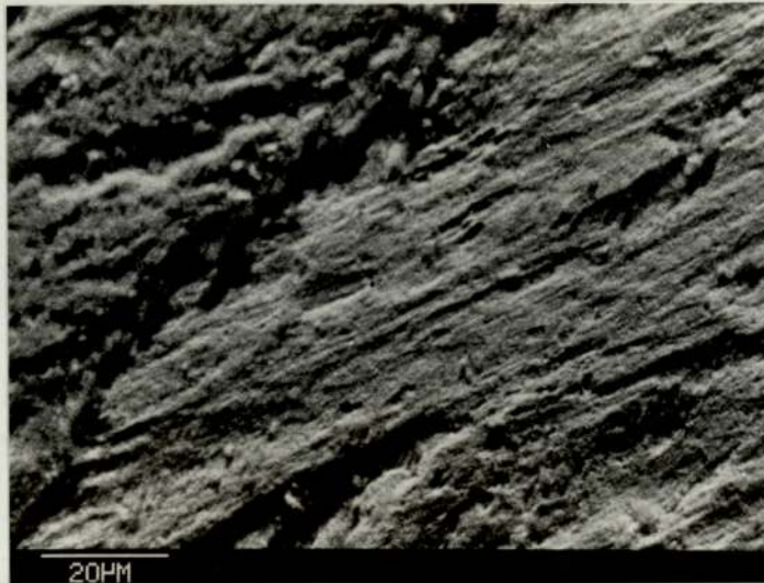
Photomicrograph 12: Surface of worn electrodeposited tin/nickel, pin no. 43, showing both wear of the coating and substrate, x 1000 magnification.
