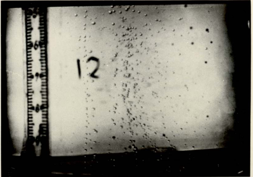
FIGURE 7.14 EFFECT OF VELOCITY ON NUMBER OF ACTIVE CHANNELS AND DROP SIZE.
