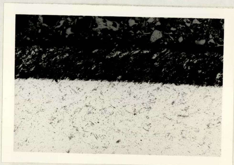
Plate-8 Microstructure of Plasma Nitrided AISI 321 Stainless steel X178
