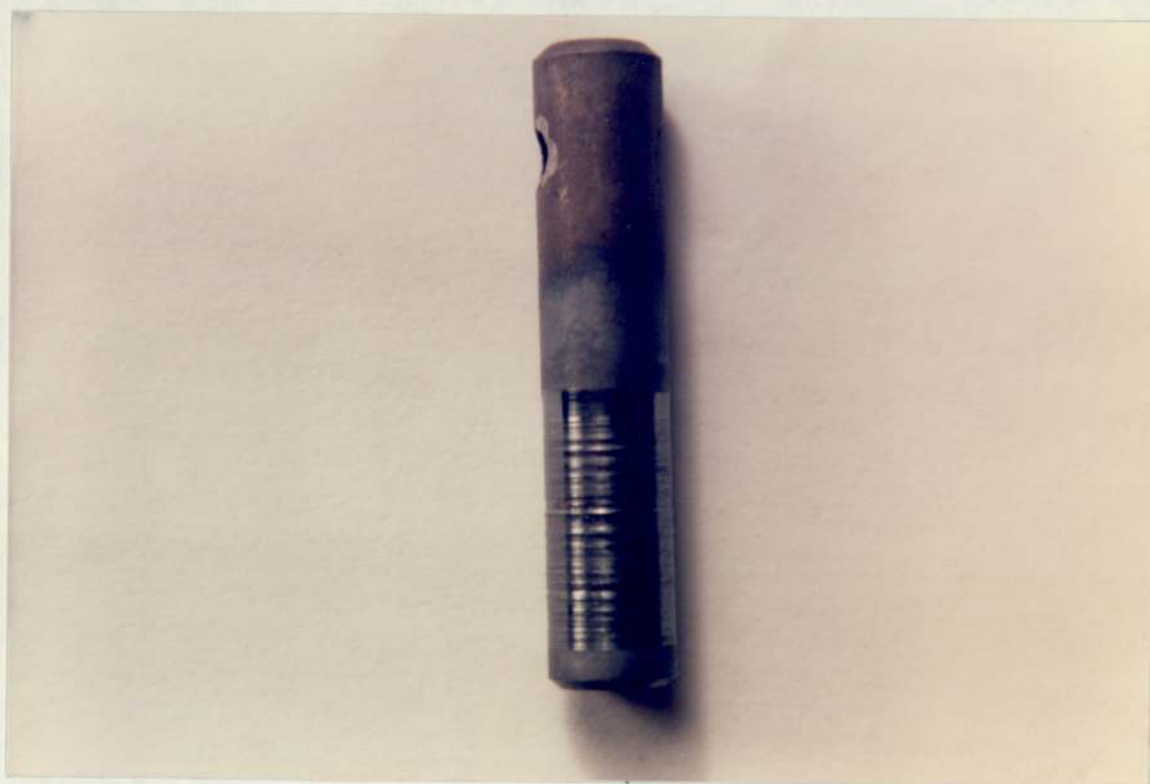
Plate-28 Scuffed Specimen after Falex Test
