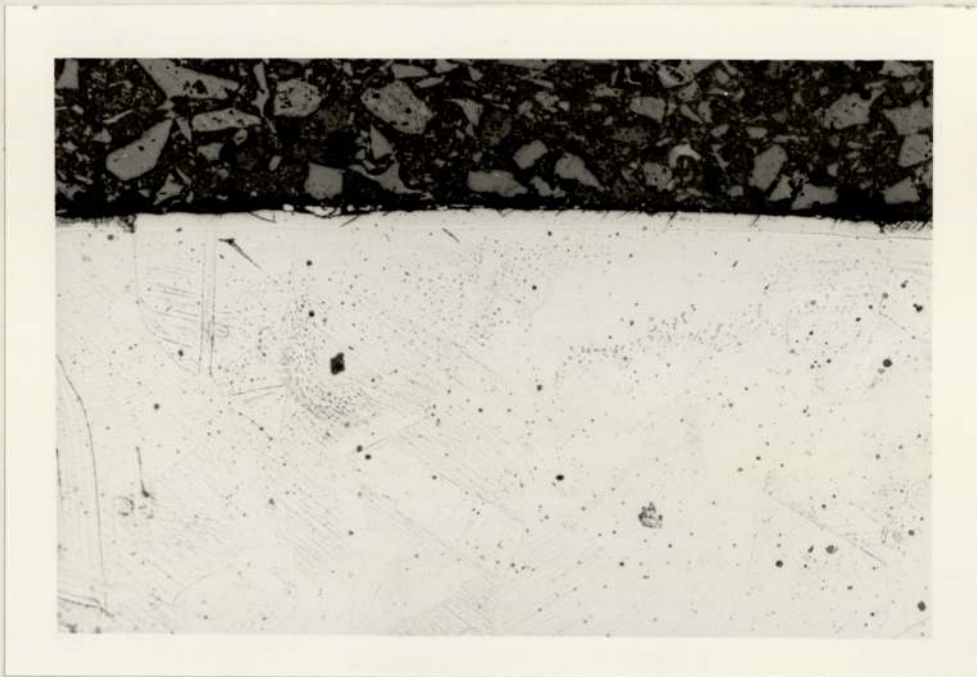
Plate-13 Microstructure of Plasma Nitrided AISI 316 Stainless Steel at 380°C X178
