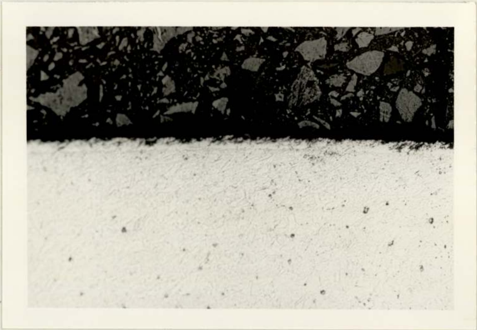
Plate-17 Microstructure of Tufftrided AISI 321 Stainless Steel X178
