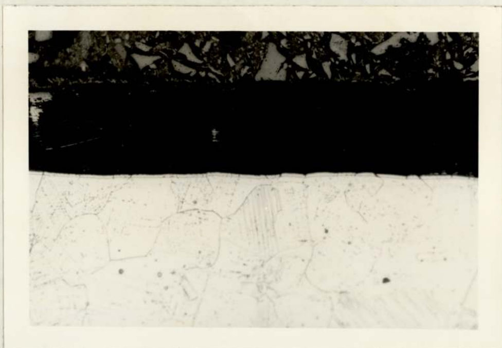
Plate-7 Microstructure of Plasma Nitrided AISI 316 Stainless Steel X178
