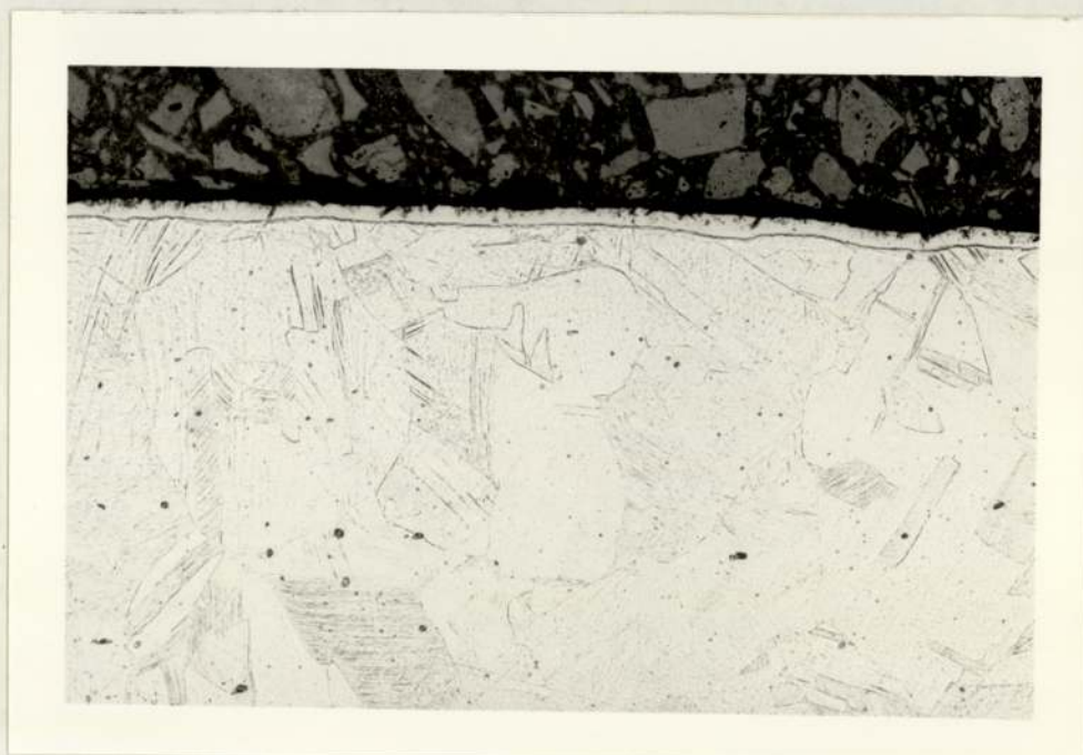
Plate-12 Microstructure of Plasma Nitrided AISI 304 Stainless Steel at 380°C X178
