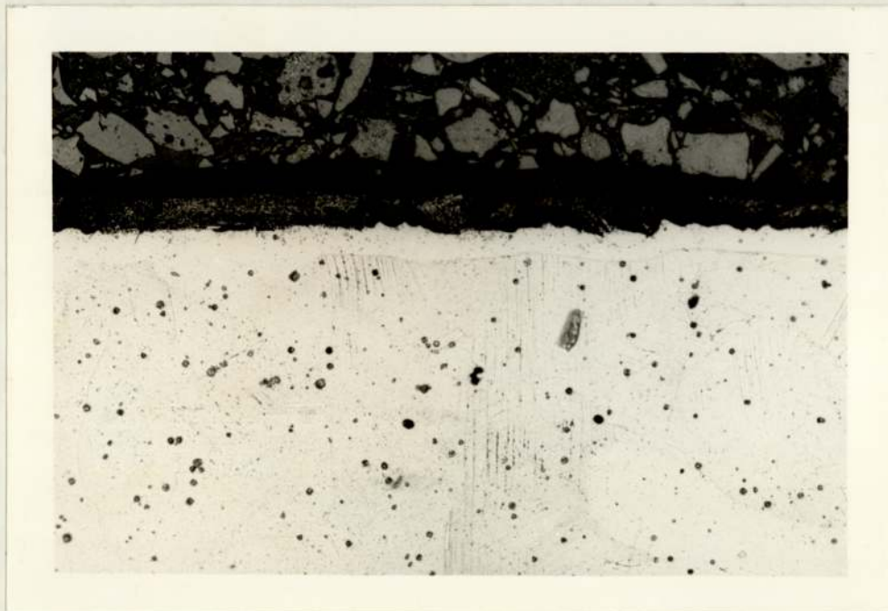
Plate-16 Microstructure of Tufftrided AISI 316 Stainless Steel X178
