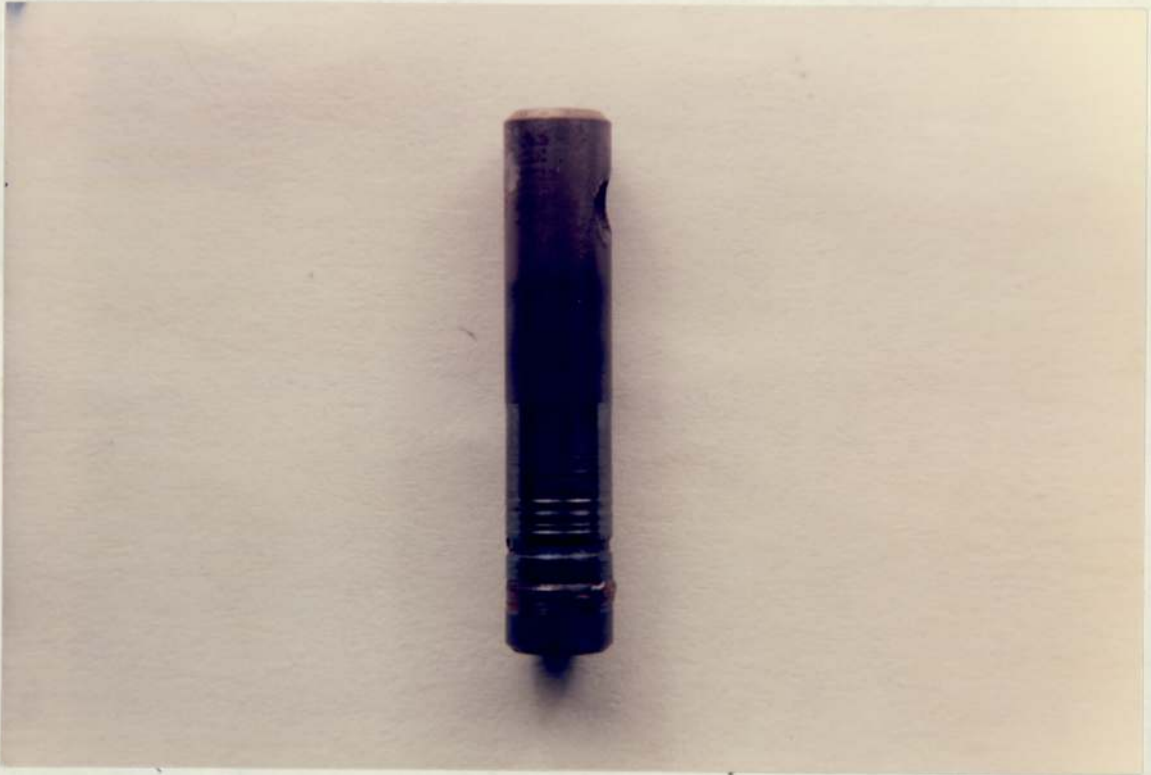
Plate-29 Badly Scuffed Specimen after Falex Test
