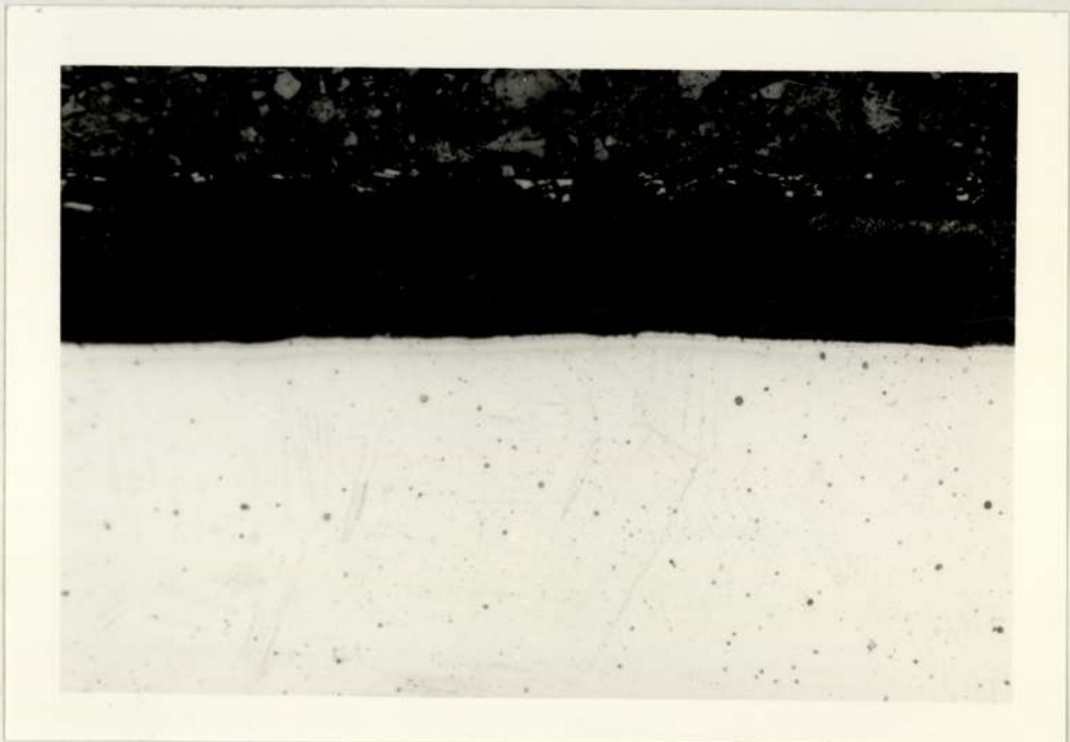
Plate-10 Microstructure of Plasma Nitrided AISI 316 Stainless Steel With Post-Oxidation X178
