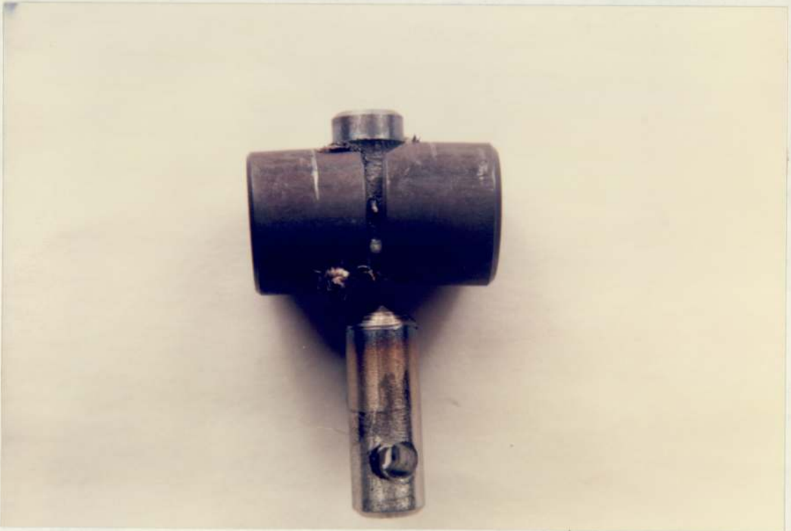
Plate-30 Totally Seized and Sheared Specimen after Falex Test
