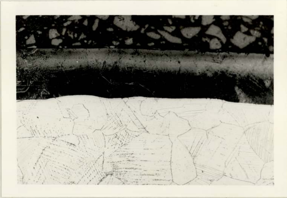
Plate-9 Microstructure of Plasma Nitrided AISI 304 Stainless Steel With Post-Oxidation X178
