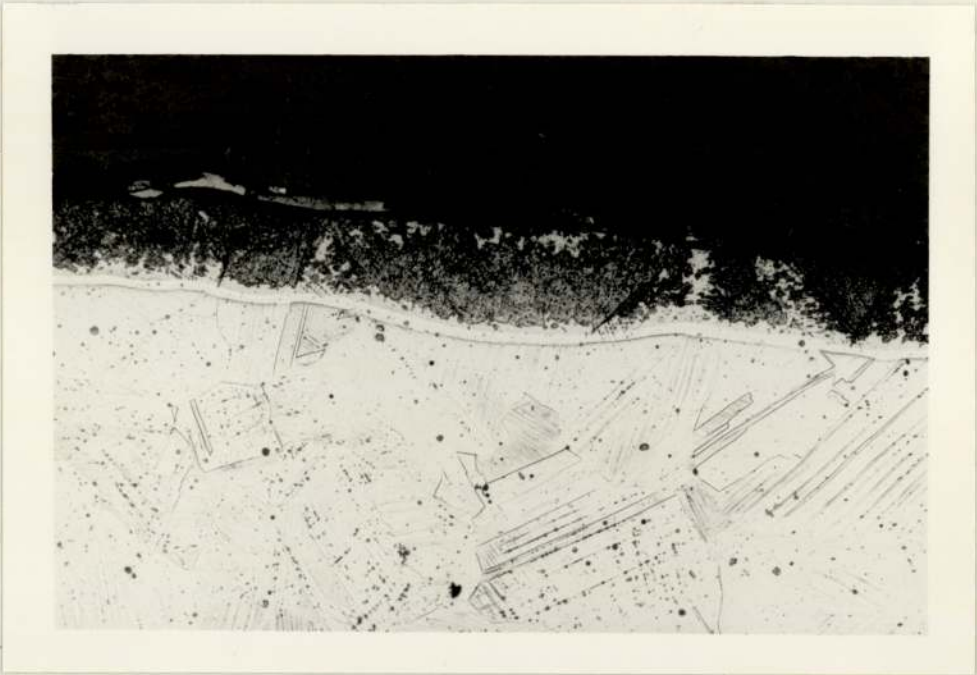
Plate-19 Microstructure of Gas Nitrided AISI 316 Stainless Steel X178
