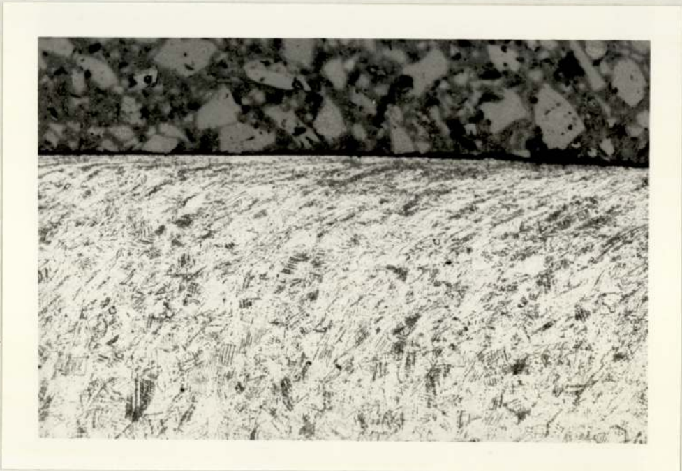
Plate-20 Microstructure of Gas Nitrided AISI 321 Stainless Steel X178
