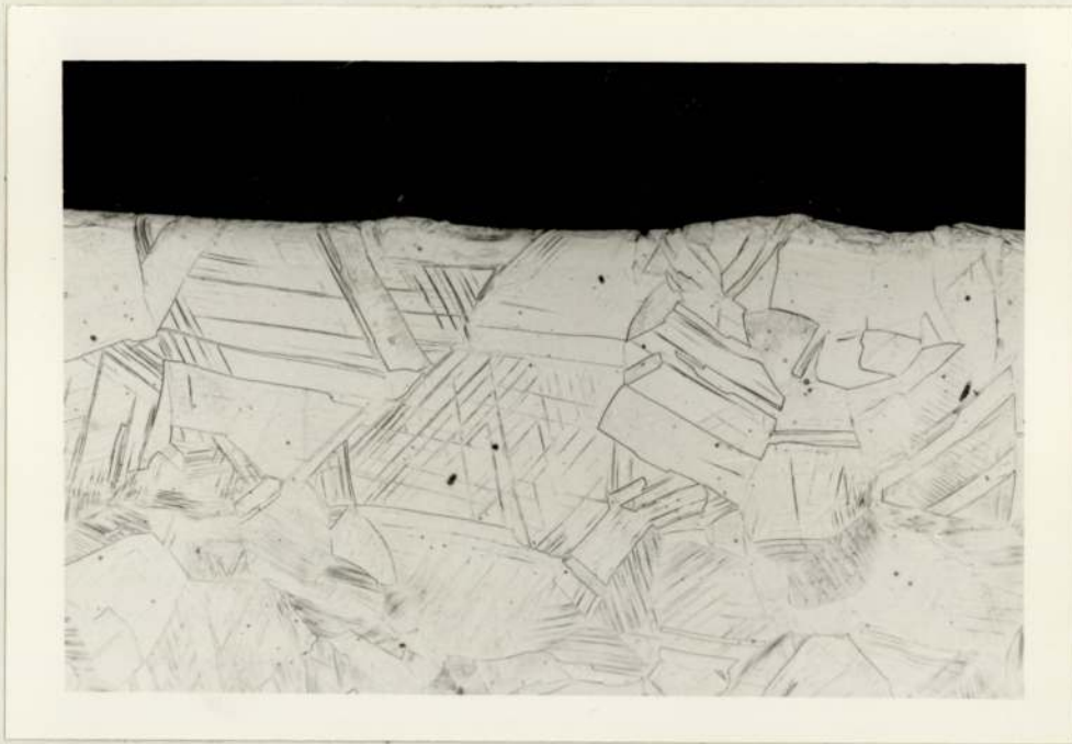
Plate-3 Microstructure of Untreated AISI 304 Stainless Steel X178
