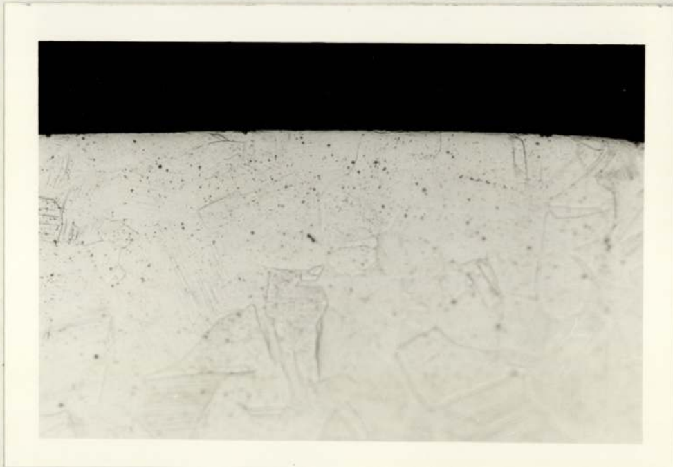
Plate-4 Microstructure of Untreated AISI 316 Stainless Steel X178
