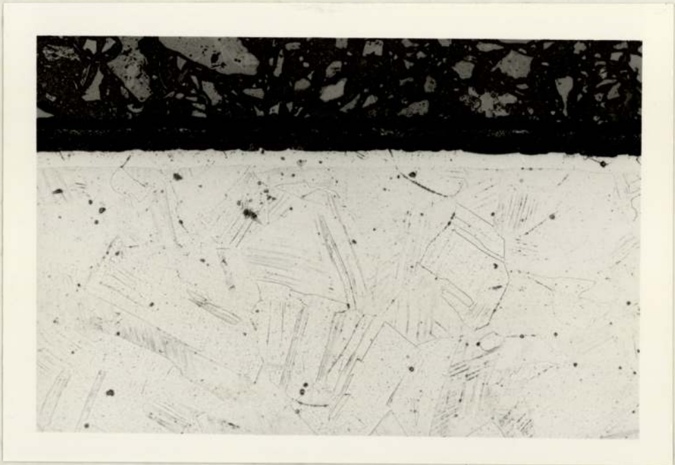
Plate-15 Microstructure of Tufftrided AISI 304 Stainless Steel X178
