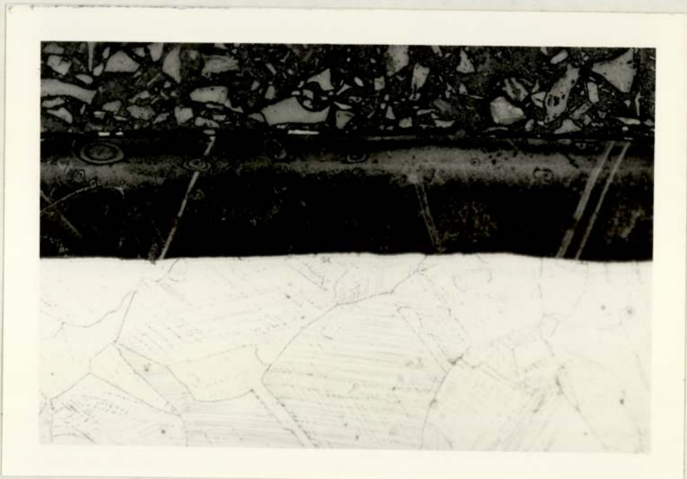
Plate-6 Microstructure of Plasma Nitrided AISI 304 Stainless Steel X178
