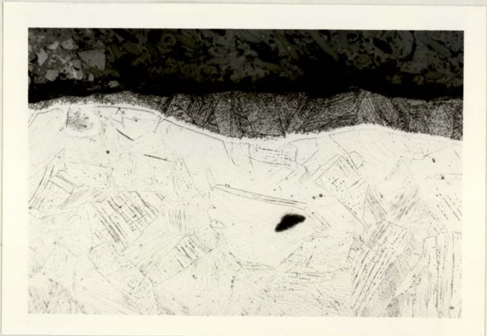
Plate-18 Microstructure of Gas Nitrided AISI 304 Stainless Steel X178
