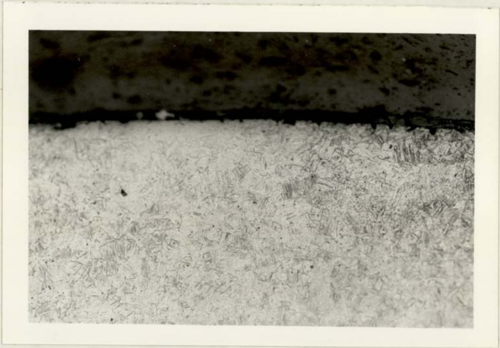
Plate-5 Microstructure of Untreated AISI 321 Stainless Steel X178
