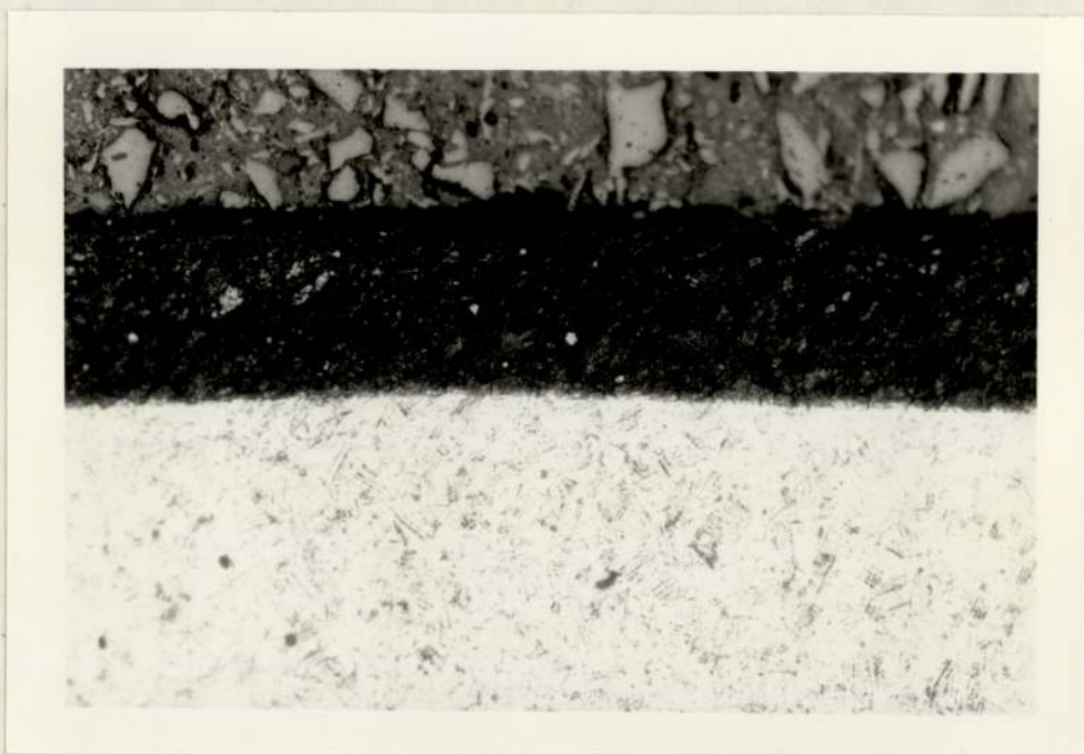
Plate-11 Microstructure of Plasma Nitrided AISI 321 Stainless Steel With Post-Oxidation X178
