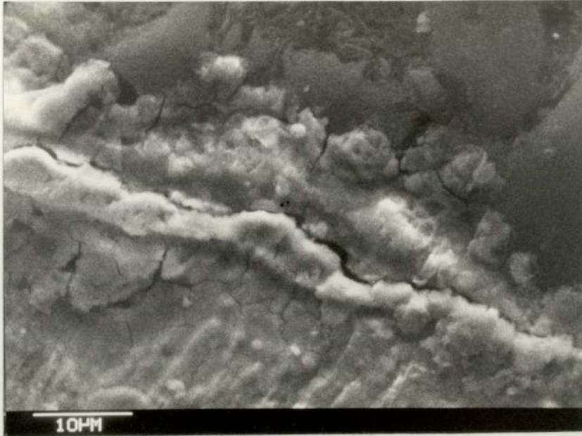
FIGURE 37: S.E.M. micrograph of a vertical section in the same die of Figure 36 inside the wear ring. It shows the propagation of sub-surface and interface cracks, and the delamination wear, x 2000
