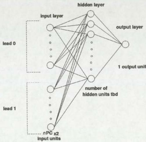
Figure 4.8: Sketch of MLP for classification using data fusion.
