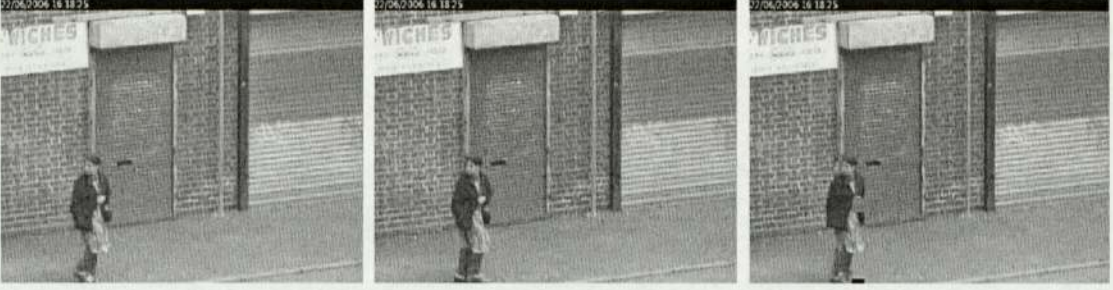
Figure 3.7: Example of motion estimation. From the initial frame (left), we reconstruct the current frame (centre) using diamond search motion estimation. The reconstructed frame is displayed on the right.
