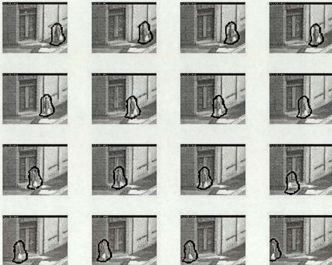
Figure 7.4: Automatic probabilistic video tracking. Initialisation of the template surrounding the shape of the man is done using motion estimation feature extraction. The probabilistic tracking algorithm with constraints is then run over a 50-frame background subtracted video sequence. One frame of every three is displayed. The black curves correspond to the fitted curves.
