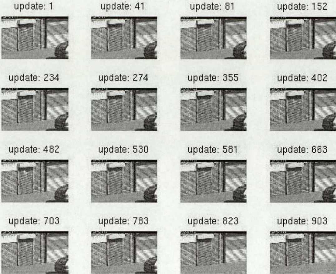
Figure 5.2: Dynamic background update. The algorithm is run over a 1000-frame video sequence. The successive backgrounds are displayed. The numbers at the top of the images correspond to the times of update (in frames). The difference between two updates varies from 40 (the minimum time step) to more than 80, depending on the number of events occurring in the scene.
