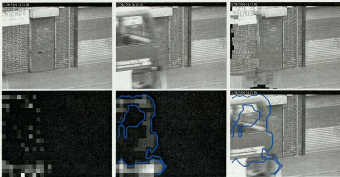
Figure 3.12: Motion estimation of a bus. Motion has been detected in the region where the bus has appeared. However, several regions of motion are extracted from only one moving object.
