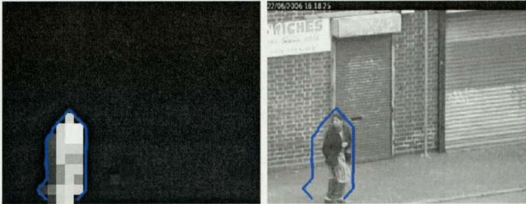
Figure 3.9: Contours of the moving objects. The motion frame is filtered to get rid of the noise due to little illumination changes (left). Contours of the moving objects are then drawn (blue curve). They are finally converted from macroblock to pixel to fit the real data (right).
