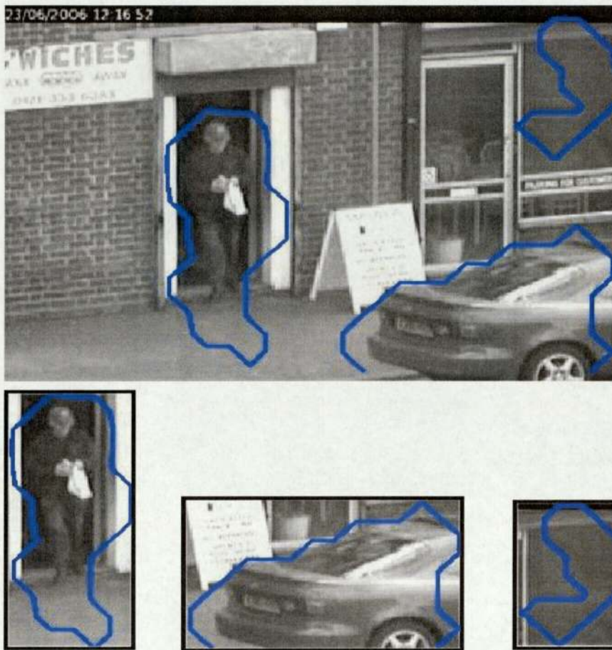
Figure 6.4: Event extraction using motion estimation. Three rectangular areas of motion (bottom images) have been detected by the motion estimation feature extraction module. Blue lines represent the boundaries of moving object found by the motion estimation algorithm.
