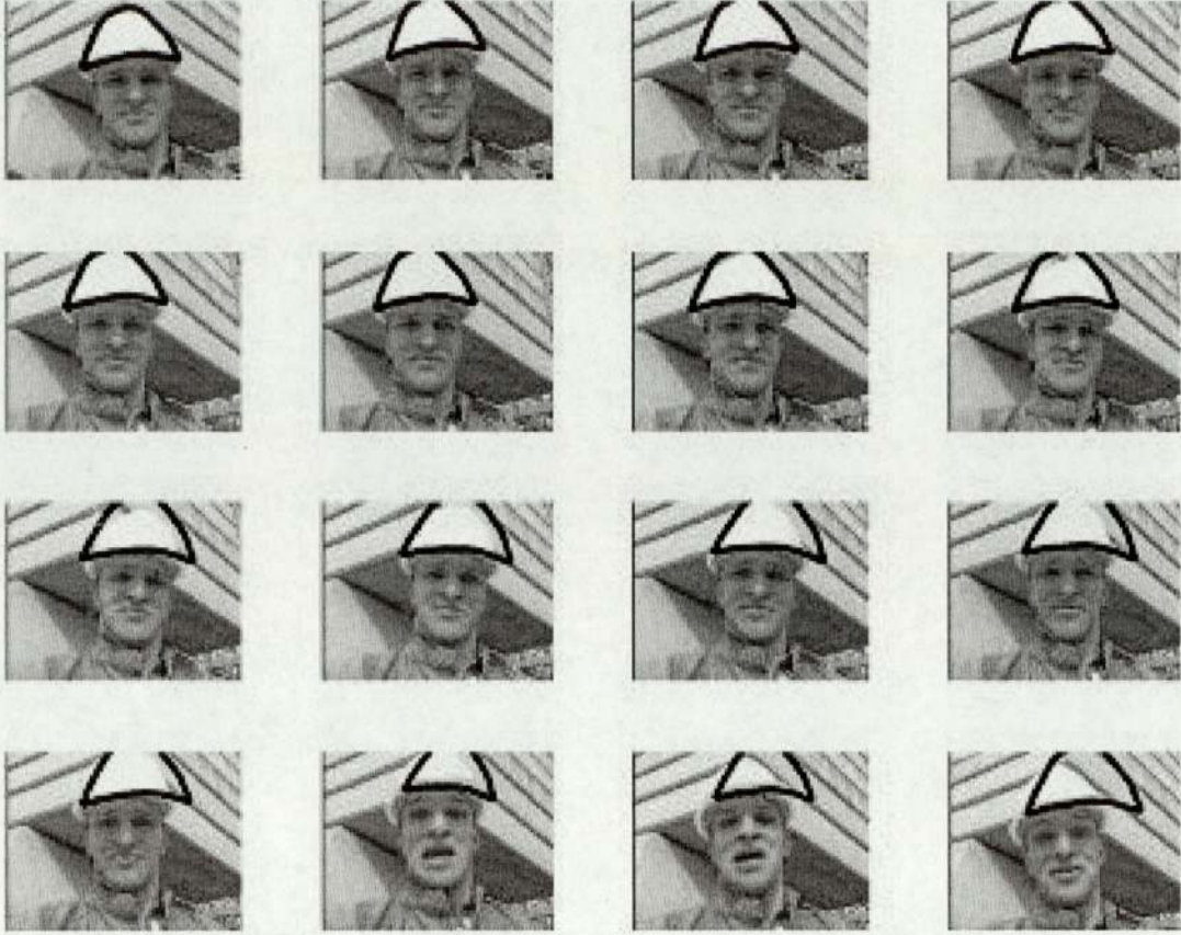
Figure 4.7: Deterministic tracking. The deterministic tracking algorithm is run over a 80-frame video sequence. One frame out of five is displayed. The black curves represent the fitted curves. After the tenth image (the fiftieth frame of the actual video sequence), the fitted curve starts to diverge to the right due to background clutter. This is the main drawback of deterministic tracking.
